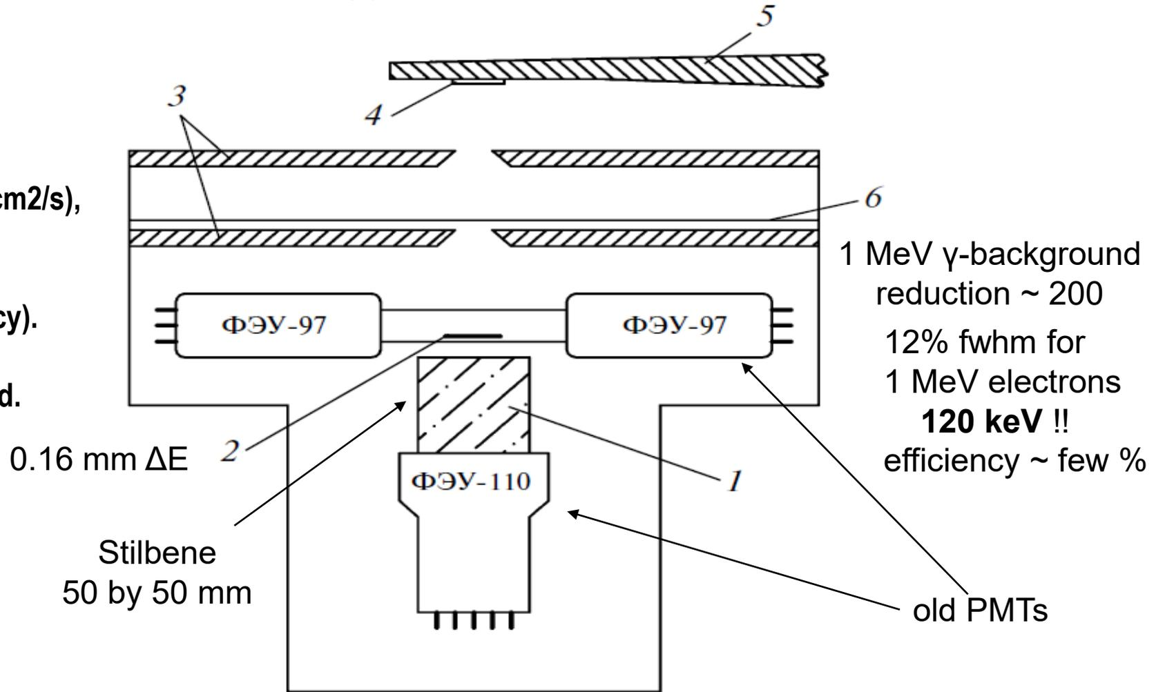
**Fig. 2.** Diagram of the  $\beta$  spectrometer: (1) main  $E$  detector, (2) drift  $\Delta E$  detector, (3) diaphragms, (4) targets, (5) rotating disk-target holder, and (6) Mylar membrane.
