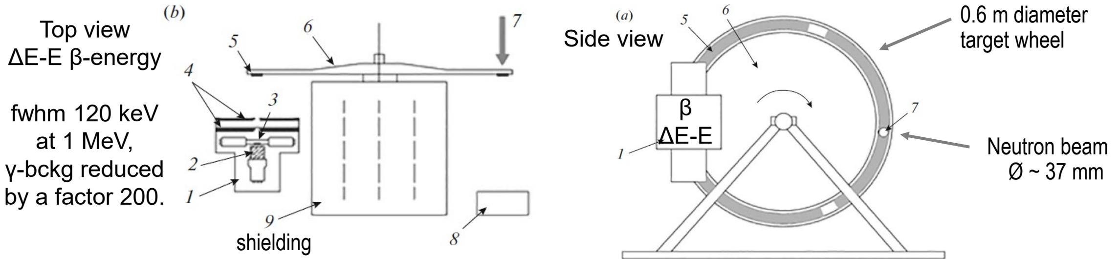
**Moderate neutron flux at KI (HFIR  $3 \times 10^7$  n/cm<sup>2</sup>/s), thick targets (!!??), small size setup with poor energy resolution but reasonable transmission (efficiency). Measurements lasting ~ days after the method was established, verified and calibrated.**
