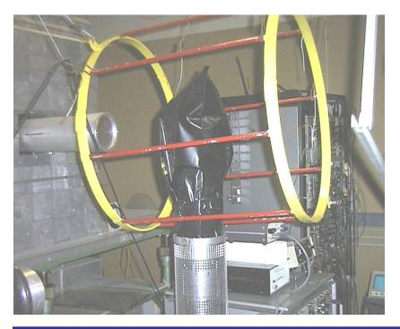
Low energy : <sup>6</sup>Li(n,t) $\alpha$  Li-glass High energy : H(n,n)H Plastic scintillator
