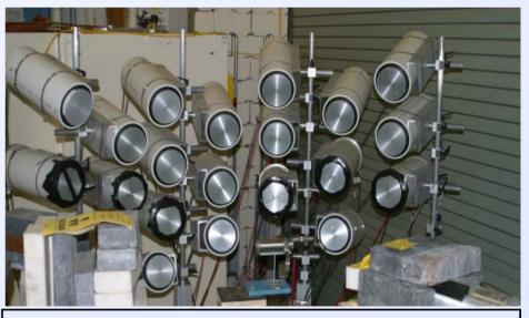
FIGARO array for the fission-neutron spectrum measurement (R. Haight of LANL)
