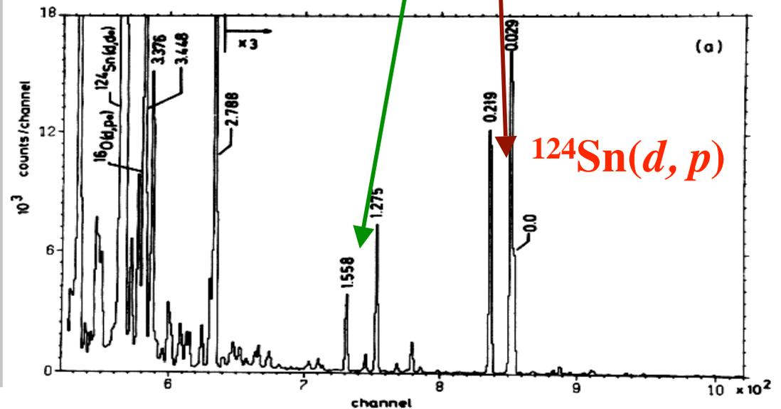
**Detect  $\gamma$  in  $\sim 4\pi$  to resolve overlapping peaks**
