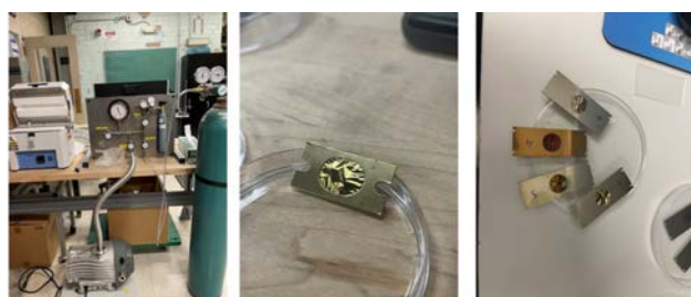
Figure 6. A tube furnace with a manifold for pumping, purging, and H source is needed. Test foils with deuterium as a surrogate.
