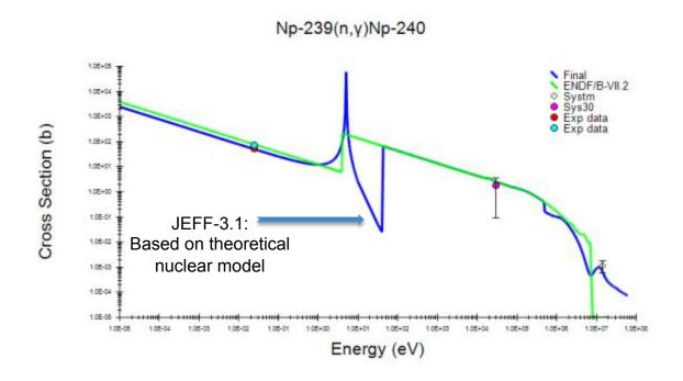
Large differences between <sup>239</sup>Np(n,γ) resulted in dramatic different Pu isotopics at low burnup. ORIGEN results for experimental Pu isotopic data from Hanford support the use of ENDF/B-VII <sup>239</sup>Np cross section data.
