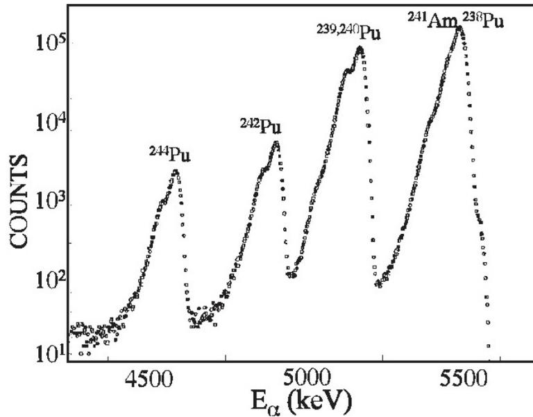
**Spectrum from alpha counting of Pu-244 samples used for fission cross section measurement by Staples and Morley**
