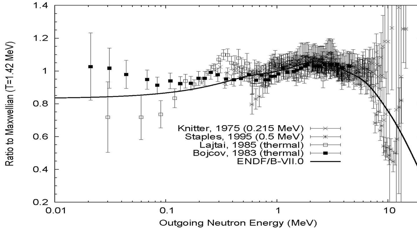
FIGURE 1. Prompt fission neutron spectrum for low-energy ( $<0.5$  MeV) neutron-induced fission of  $^{239}\text{Pu}$ .
