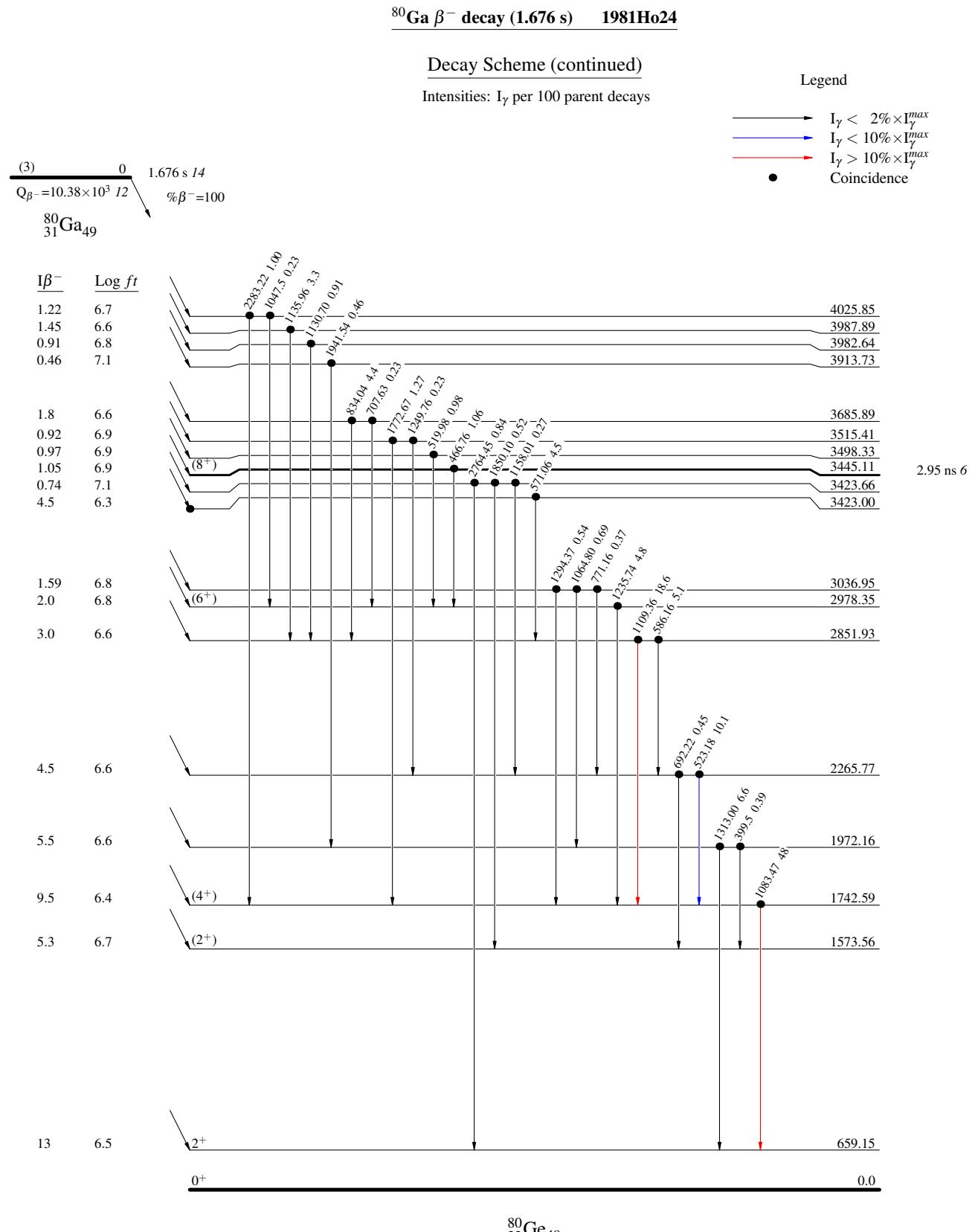
$^{80}\text{Ga } \beta^-$  decay (1.676 s)    1981Ho24Decay Scheme (continued)Intensities:  $I_{\gamma}$  per 100 parent decays
