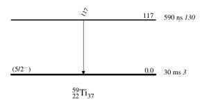
$<sup>^{59}</sup>$ Ti produced in fragmentation of  $^{76}$ Ge $^{30+}$  beam on a  $^{58}$ Ni target. LISE3 achromatic spectrometer used to separate fragments; magnetic rigidity was tuned to optimize transmission of <sup>62</sup>V and <sup>64</sup>Cr fragments. Transmitted nuclei were identified by three consecutive Si detectors where two served for energy loss and time-of-flight measurements while the last one determined their residual energies.
