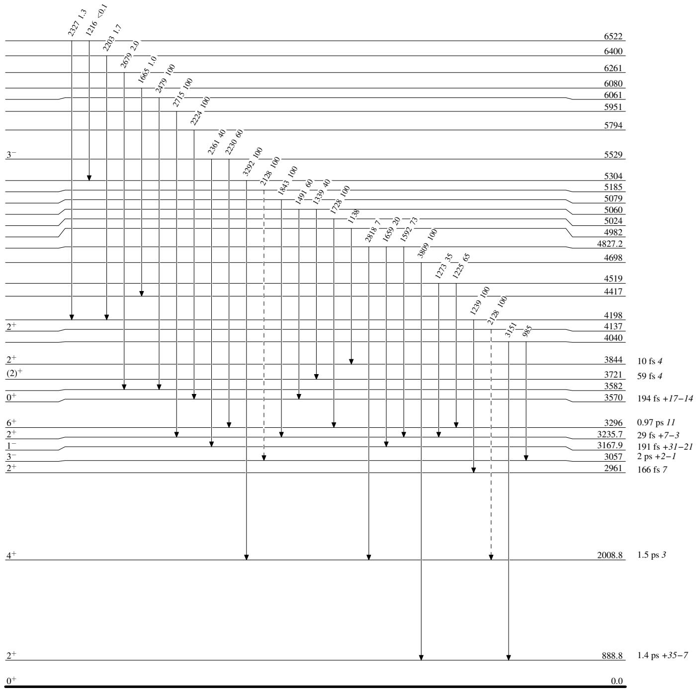
$^{45}\text{Sc}(\text{p},\gamma)$ : secondary  $\gamma$ 's    1987Mo17Level Scheme (continued)
