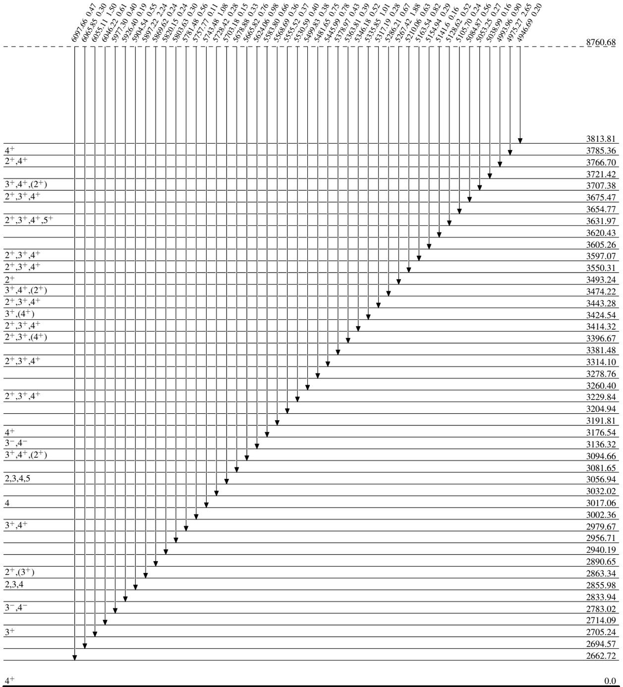
$^{45}\text{Sc}(n,\gamma) \text{E=thermal}$  1982Ti02
