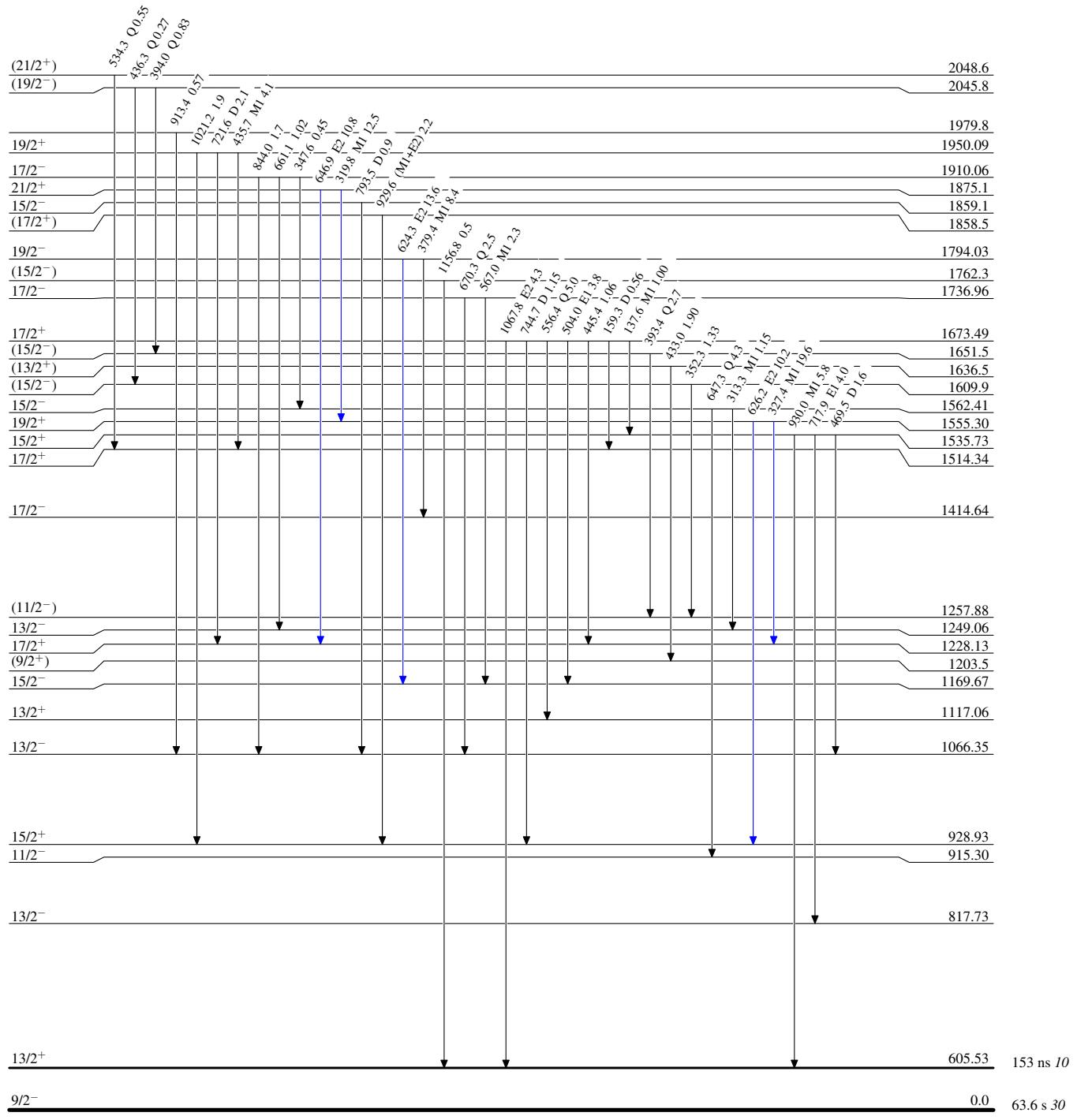
$^{165}\text{Ho}(\text{32S},4n\gamma)$     2015He27Level Scheme (continued)Intensities: Relative  $I_\gamma$
