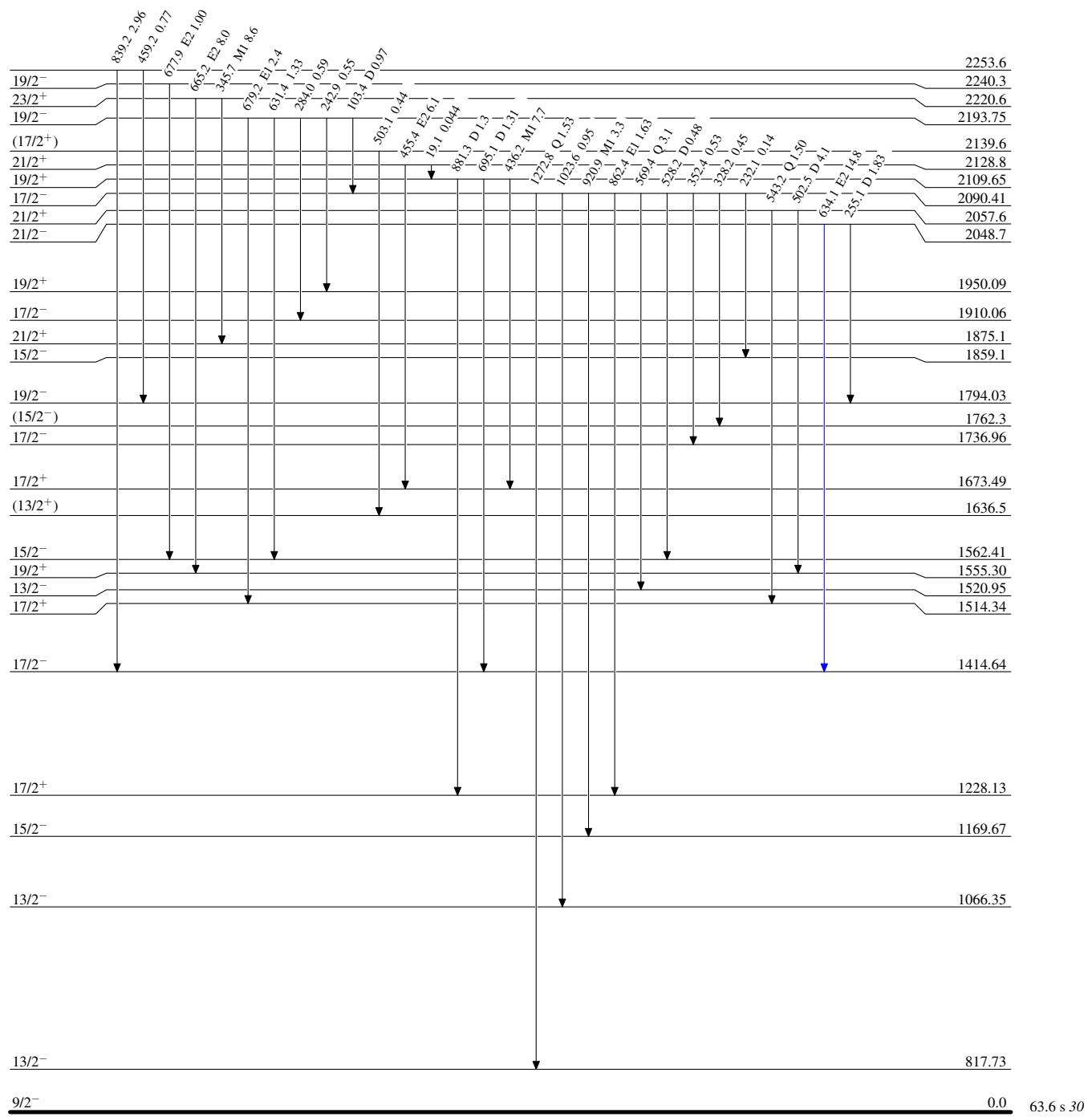
**$^{165}\text{Ho}(\text{<sup>32</sup>S},4\gamma)$  2015He27****Level Scheme (continued)****Legend**Intensities: Relative  $I_\gamma$
