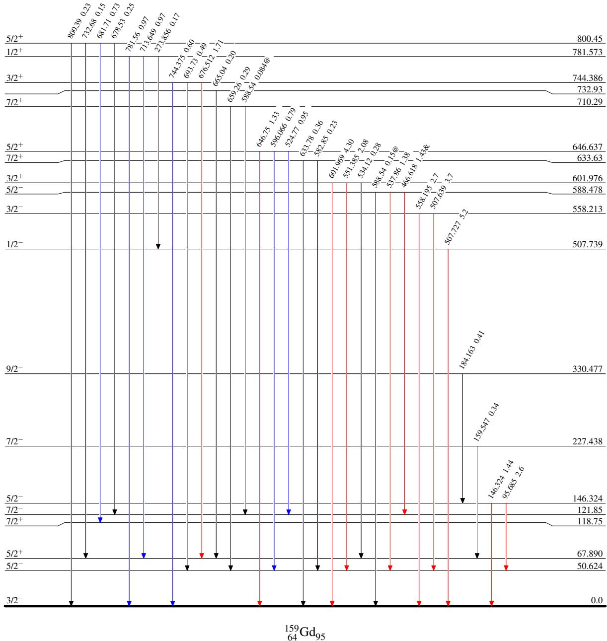
$^{158}\text{Gd}(n,\gamma)$  E=thermal    2004Gr26,1971Gr42Band(F):  $v3/2[402]$  band $\underline{\underline{5/2^+}} \quad \underline{\underline{800.45}}$  $\underline{\underline{3/2^+}} \quad \underline{\underline{744.386}}$ Band(E): Proposed
