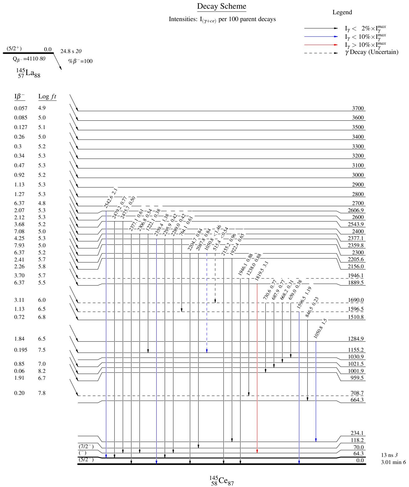
$^{145}\text{La } \beta^- \text{ decay} \quad 1978\text{Pf02,1997Gr09}$
