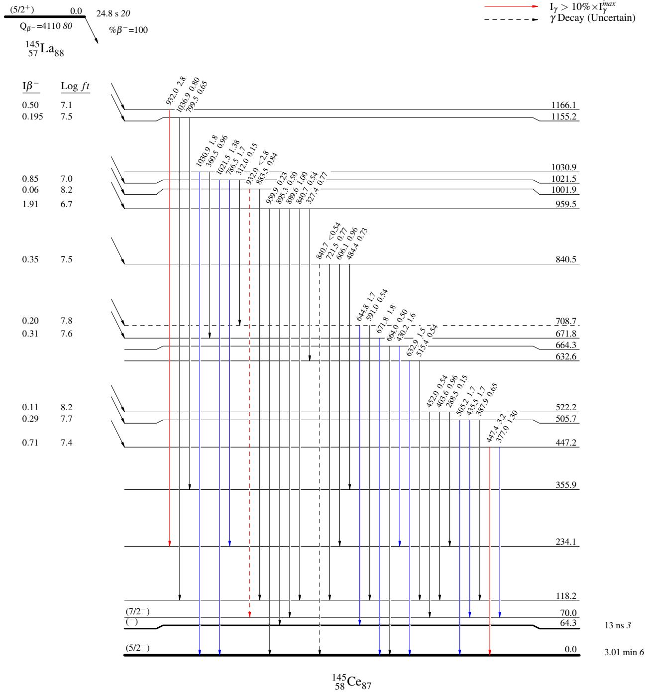
$^{145}\text{La} \beta^- \text{ decay} \quad 1978\text{Pf02,1997Gr09}$
