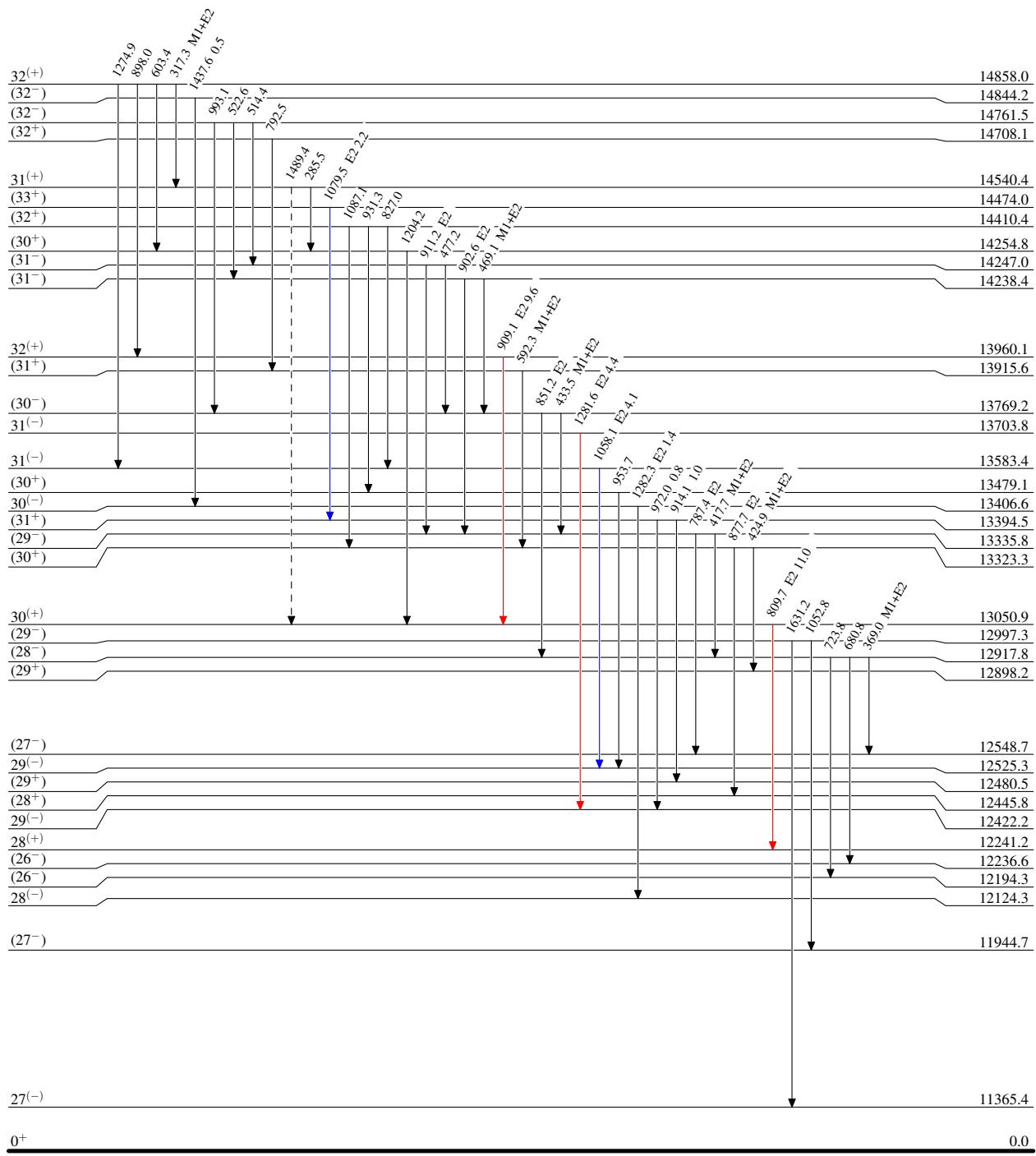
**$^{96}\text{Zr}({}^{48}\text{Ca},4n\gamma)$**     **2013Le22,2013Va10****Level Scheme (continued)**Intensities: Relative  $I_\gamma$
