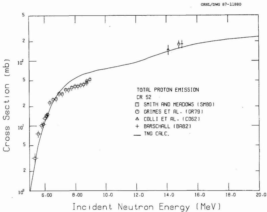
**Fig. 37.** Comparison of calculated and experimental cross sections for the total proton emission of  $^{52}\text{Cr}$ .
