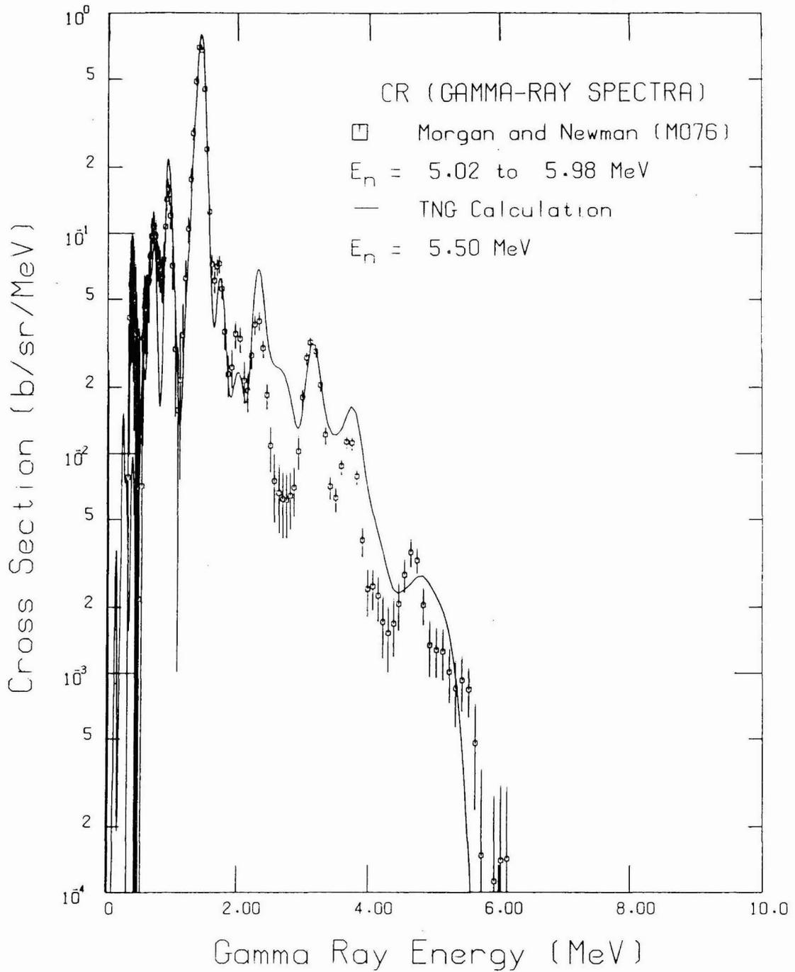
Fig. 53. Secondary gamma-ray spectra versus gamma-ray energy from the TNG calculation (incident energy  $E_n = 5.5$  MeV) compared with the data of Morgan and Newman (MO76).
