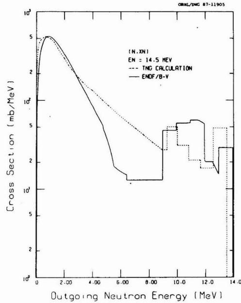
**Fig. 61. Comparison of  $(n, xn)$  from ENDF/B-V with the TNG calculation for incident neutron energy of 14.5 MeV.**
