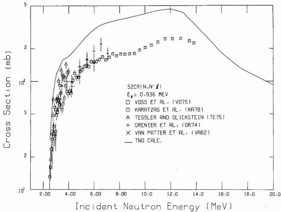
Fig. 44. Comparison of calculated and experimental data of the excitation function for the  $E_\gamma = 0.936$  MeV transition following  $^{52}\text{Cr}(n,n'\gamma)$ .
