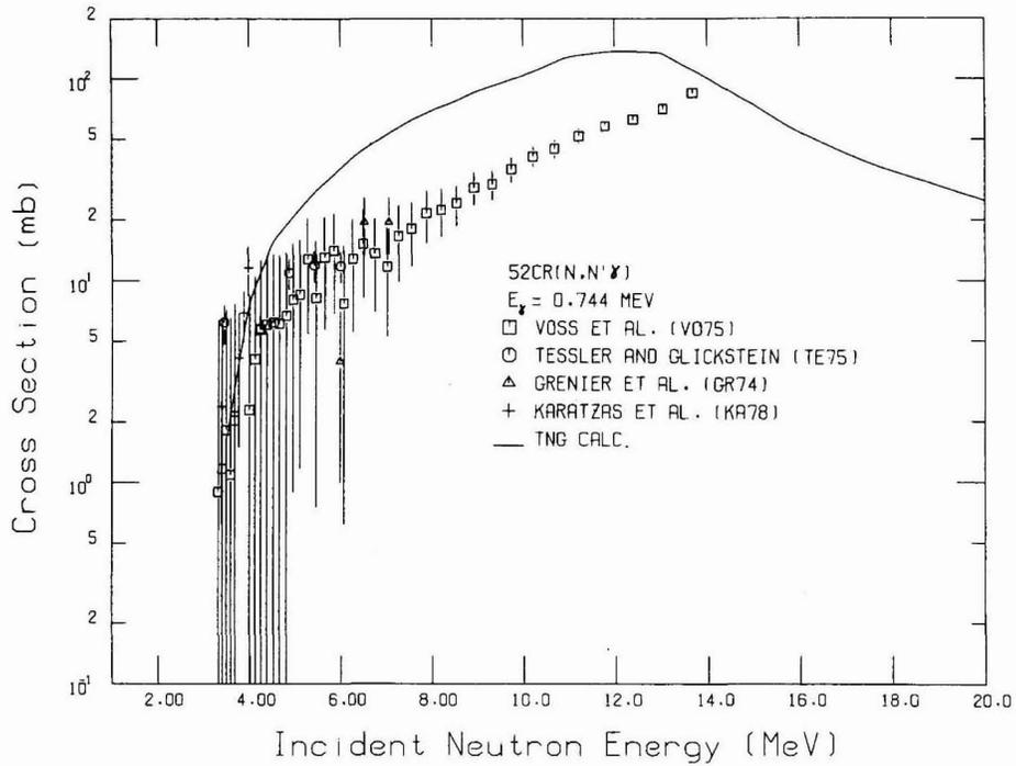
Fig. 43. Comparison of calculated and experimental data of the excitation function for the  $E_\gamma = 0.744$  MeV transition following  $^{52}\text{Cr}(n,n'\gamma)$ .
