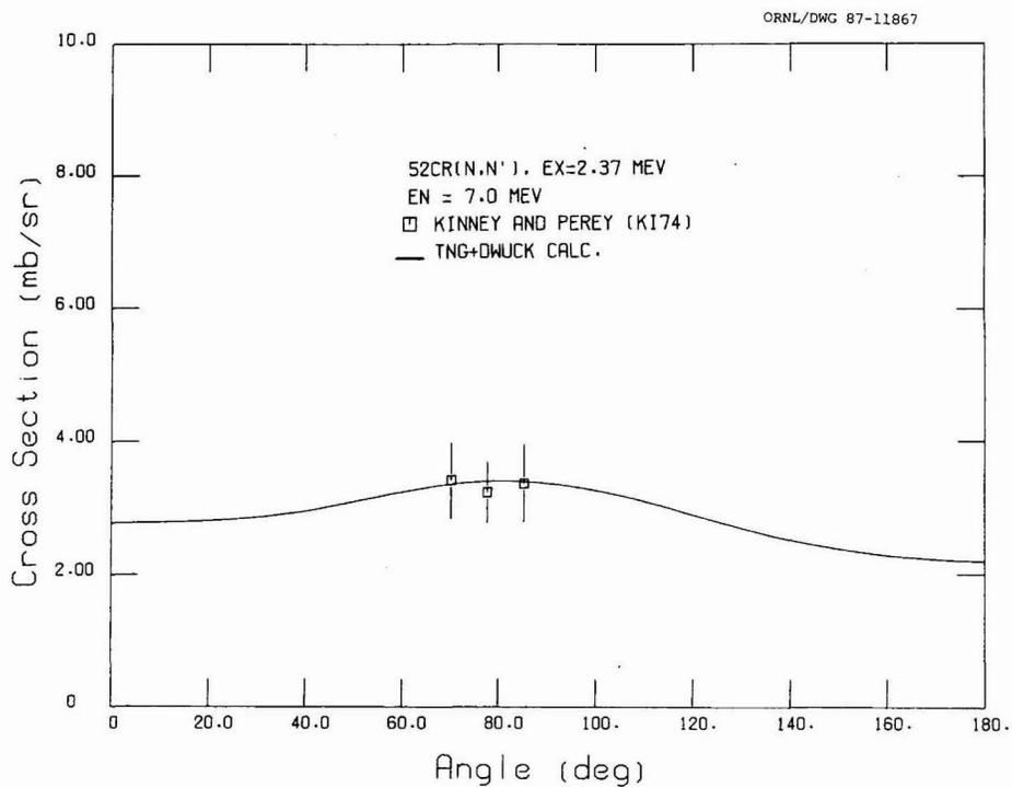
**Fig. 23.** Comparison of calculated and experimental differential cross sections for exciting the 2.37-MeV level at  $E_n = 7.0$  MeV.
