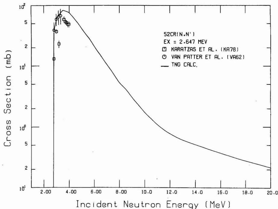
Fig. 28. Comparison of calculated and experimental  $^{52}\text{Cr}(n,n')$  cross sections for exciting the 2.647-MeV level.
