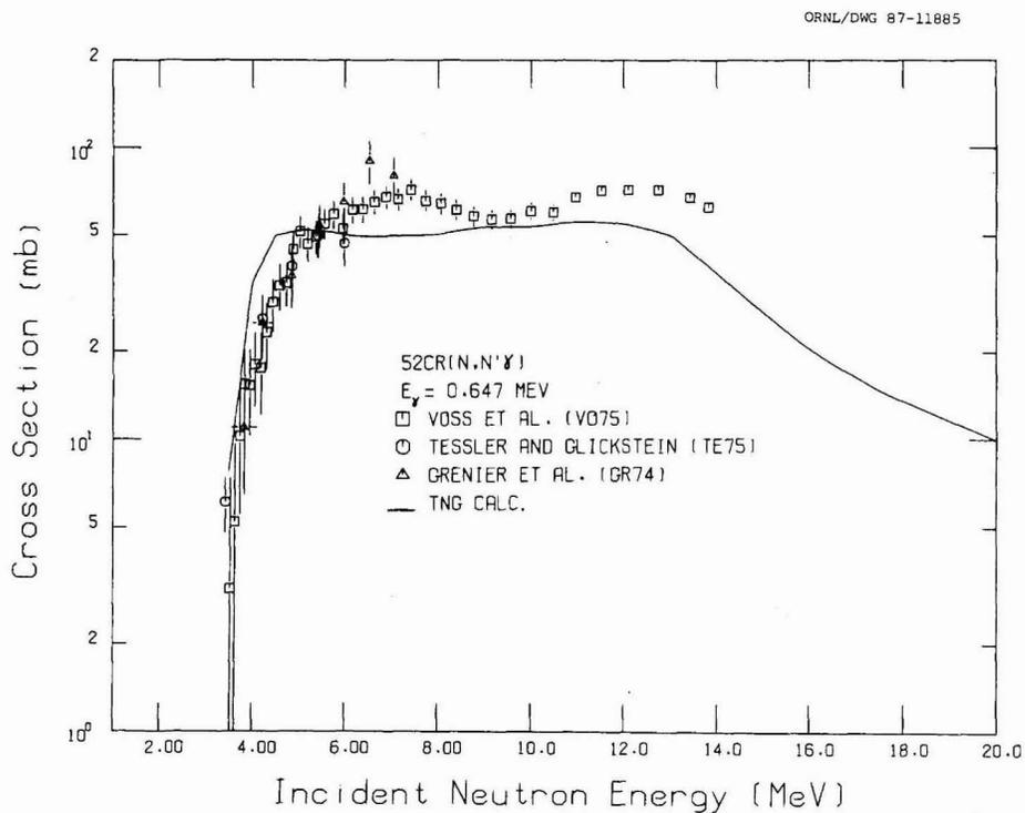
Fig. 42. Comparison of calculated and experimental data of the excitation function for the  $E_\gamma = 0.647 \text{ MeV}$  transition following  $^{52}\text{Cr}(n,n'\gamma)$ .
