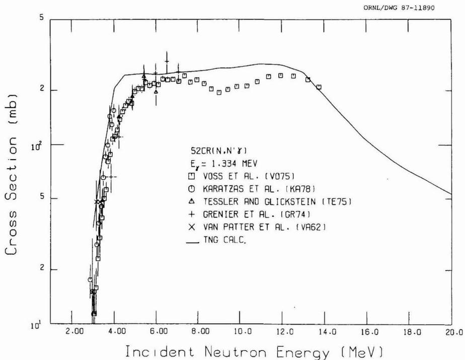
**Fig. 47. Comparison of calculated and experimental data of the excitation function for the  $E_{\gamma} = 1.334$  MeV transition following  $^{52}\text{Cr}(n,n'\gamma)$ .**
