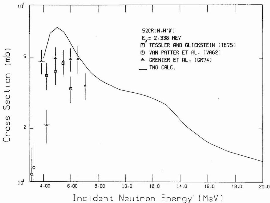
**Fig. 51.** Comparison of calculated and experimental data of the excitation function for the  $E_\gamma = 2.338$  MeV transition following  $^{52}\text{Cr}(n,n'\gamma)$ .
