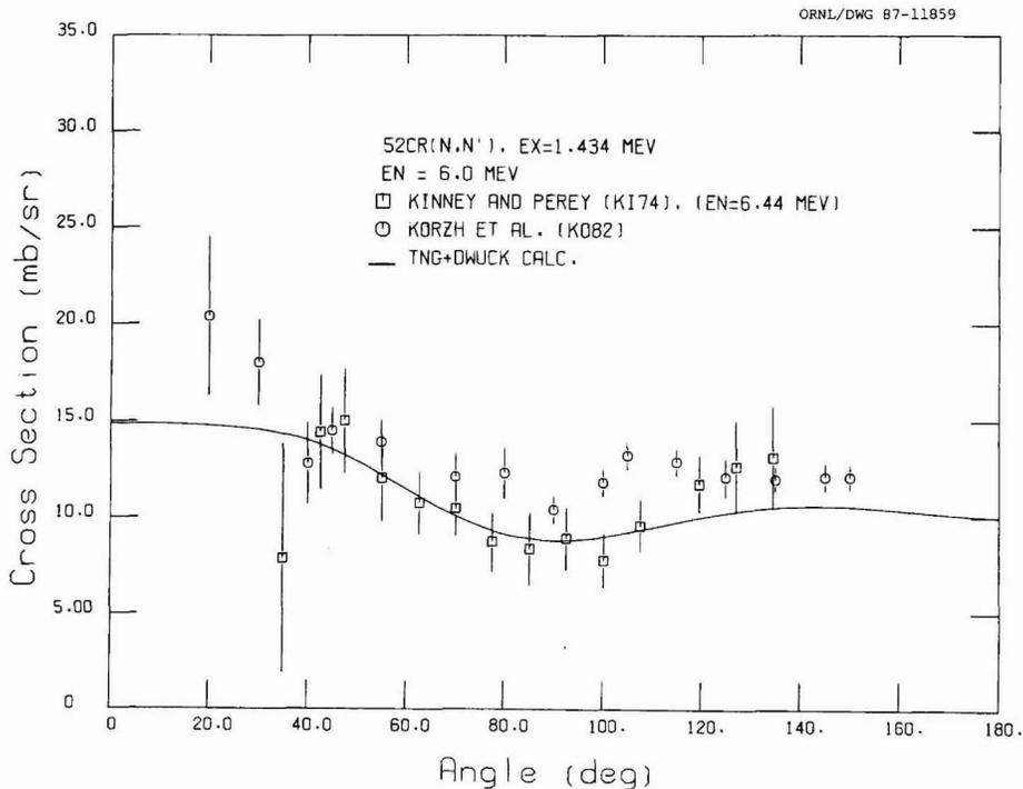
**Fig. 15.** Comparison of calculated and experimental differential cross sections for exciting the 1.434-MeV level at  $E_n = 6.0$  MeV.
