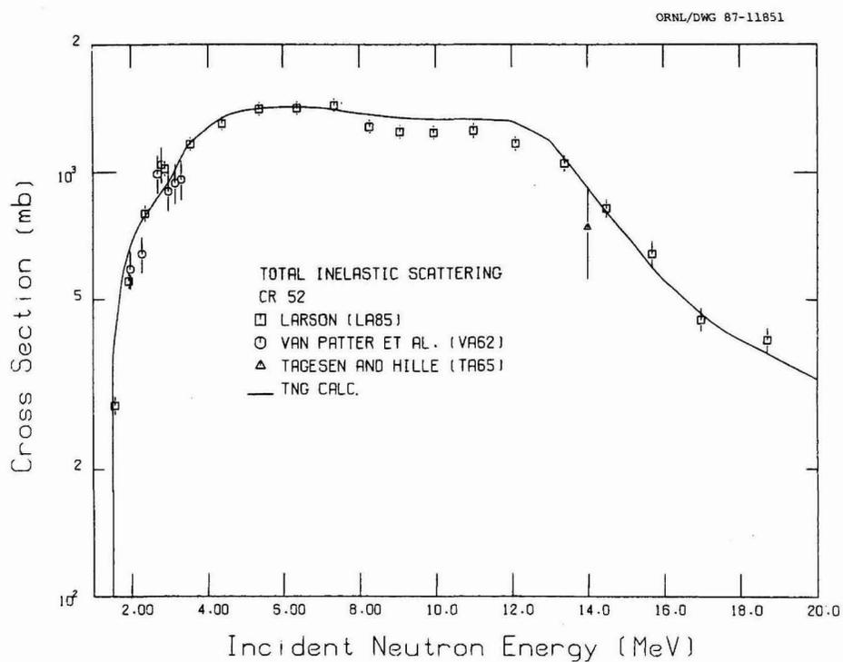
**Fig. 10. Comparison of calculated and experimental total inelastic scattering cross sections for  $^{52}\text{Cr}$ .**
