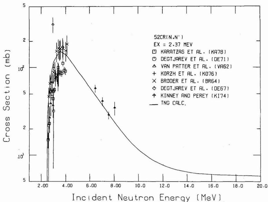
Fig. 27. Comparison of calculated and experimental  $^{52}\text{Cr}(n,n')$  cross sections for exciting the 2.37-MeV level.
