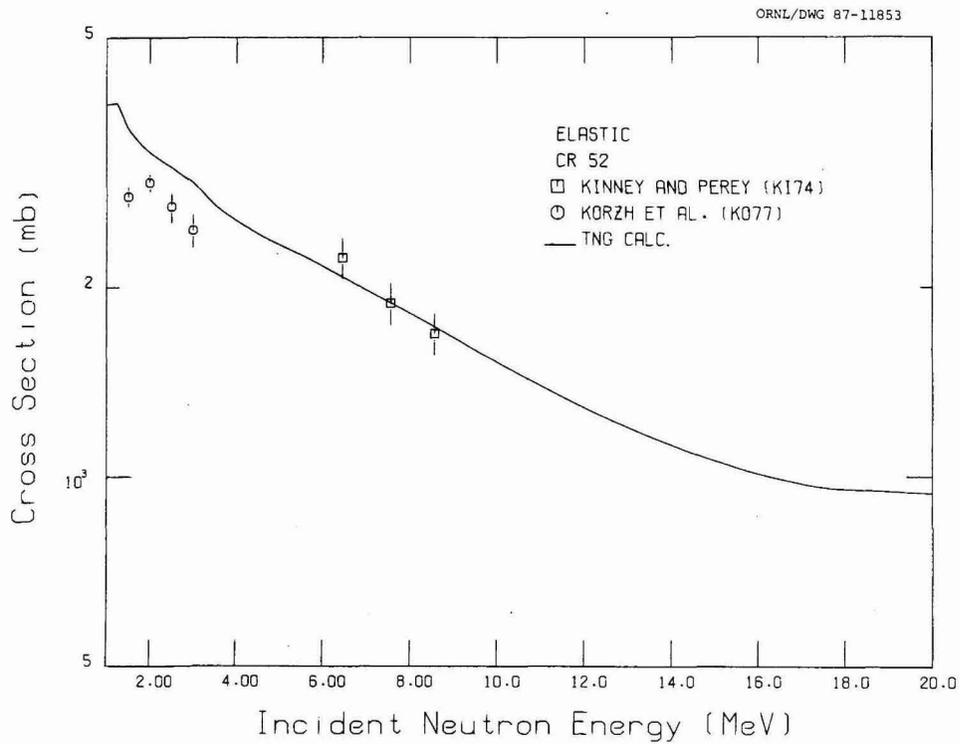
**Fig. 4. Comparison of calculated and experimental elastic cross sections for  $^{52}\text{Cr}$ .**
