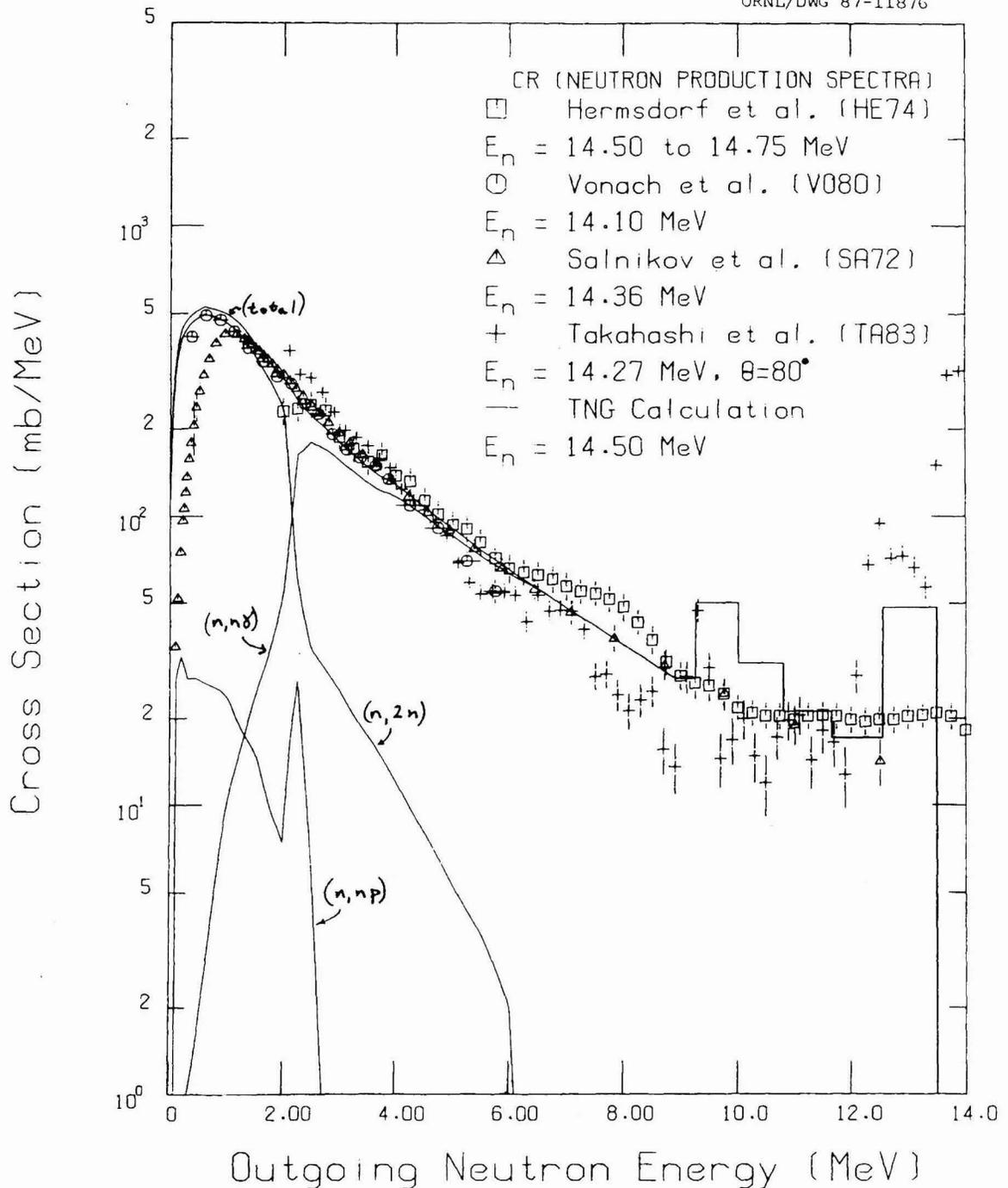
**Fig. 33. Neutron emission spectra from the TNG calculation compared with experimental data.** The data of Takahashi et al. (TA83) were taken at  $80^\circ$ , and the other measured data sets shown (HE74, VO80, and SA72) are angle integrated. Contributions from the various neutron-producing components are shown (they sum to the total). The curves labeled  $(n,np)$  and  $(n,n\alpha)$  include the  $(n,pn)$  and  $(n,\alpha n)$  components, respectively.
