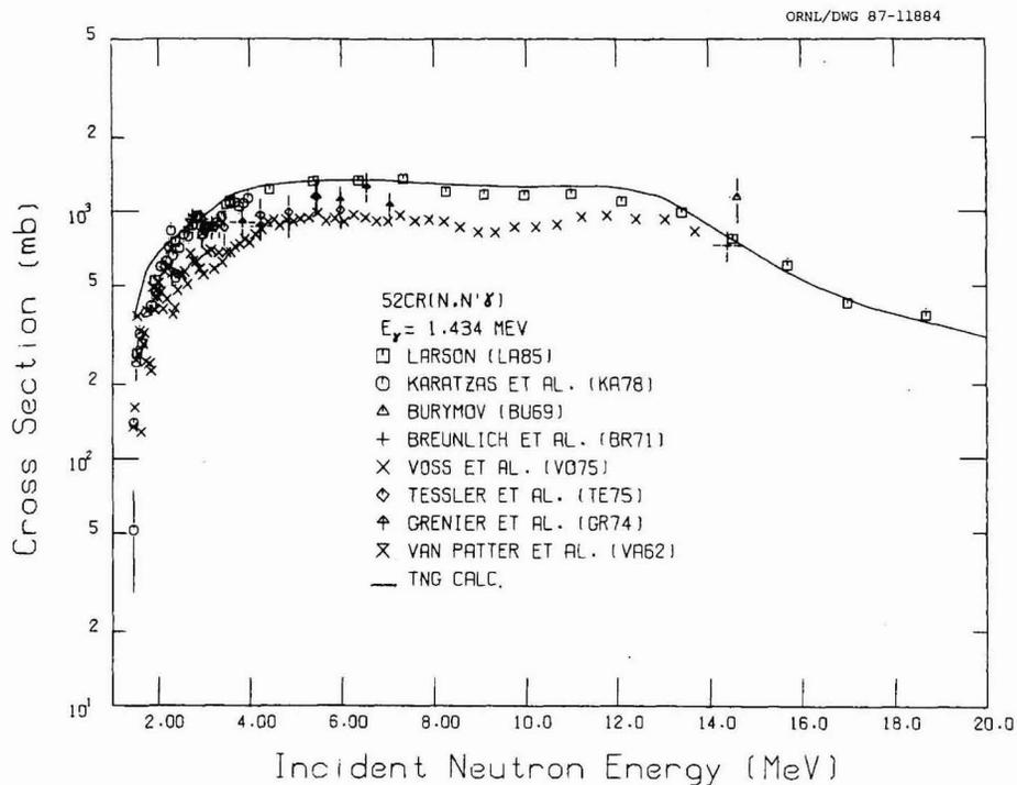
Fig. 41. Comparison of calculated and experimental data of the excitation function for the  $E_\gamma = 1.434 \text{ MeV}$  transition following  $^{52}\text{Cr}(n,n'\gamma)$ .
