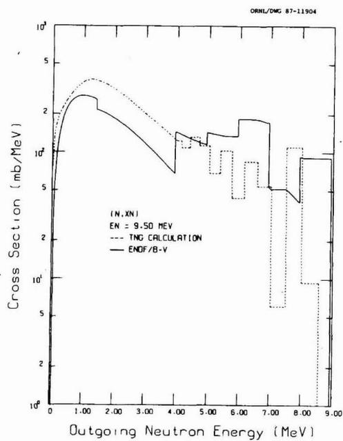
**Fig. 60. Comparison of  $(n, xn)$  from ENDF/B-V with the TNG calculation for incident neutron energy of 9.5 MeV.**
