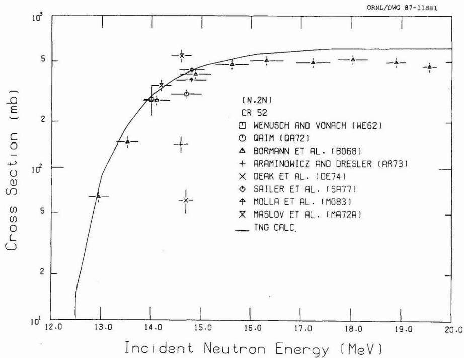
**Fig. 38.** Comparison of calculated and experimental  $^{52}\text{Cr}(n,2n)$  cross sections.
