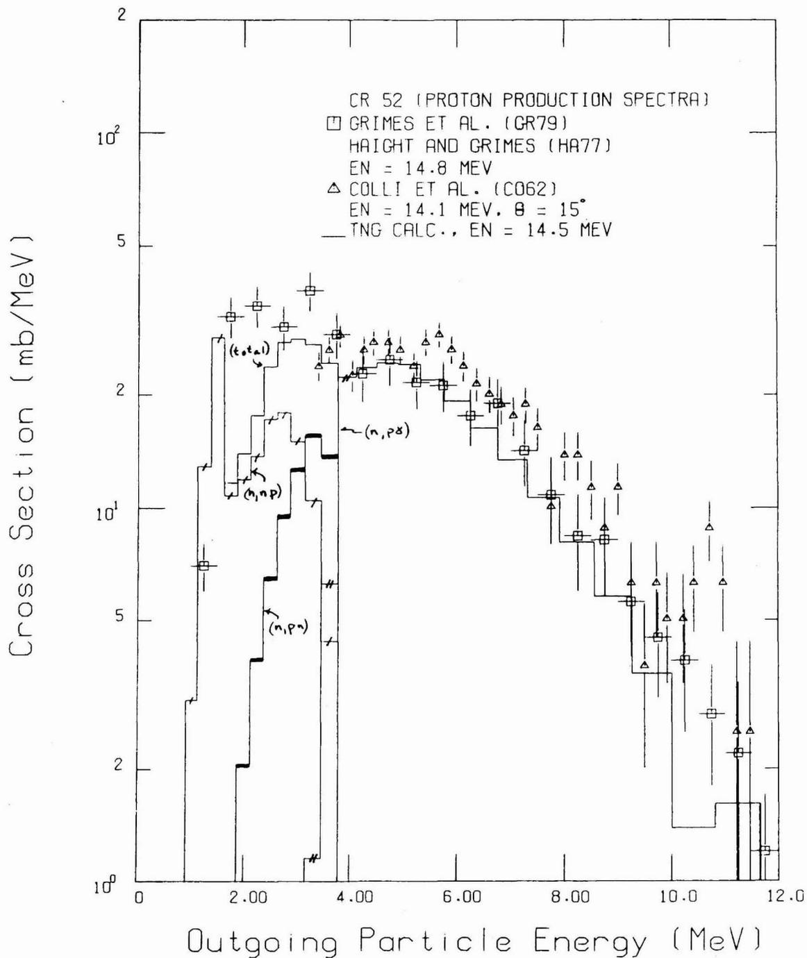
**Fig. 34. Comparison of calculated experimental proton production spectra for  $^{52}\text{Cr}$ .** The measurements were taken at incident energies of 14.8 and 14.1 MeV; the TNG calculation was for  $E_n = 14.5$  MeV. The data of Grimes et al. (GR79, HA77) are angle integrated; the data of Colli et al. (CO62) were taken at  $15^\circ$ .
