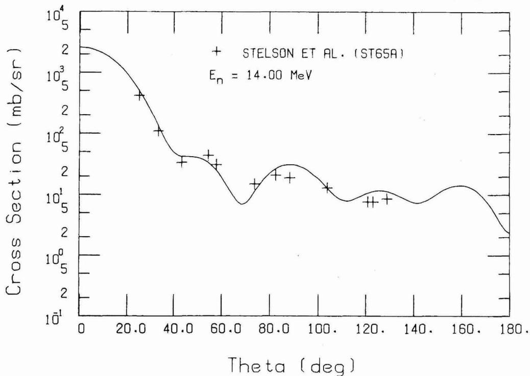
Fig. 9. Comparison of calculated ( $^{52}\text{Cr}$ ) and experimental ( $^{64}\text{Cr}$ ) differential elastic scattering cross sections at  $E_n = 14.0$  MeV.
