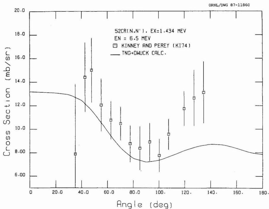
**Fig. 16. Comparison of calculated and experimental differential cross sections for exciting the 1.434-MeV level at  $E_n = 6.5$  MeV.**
