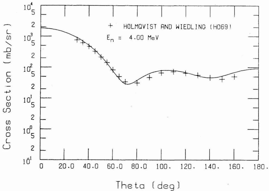
Fig. 7. Comparison of calculated ( $^{52}\text{Cr}$ ) and experimental ( $^{54}\text{Cr}$ ) differential elastic scattering cross sections at  $E_n = 4.0$  MeV.
