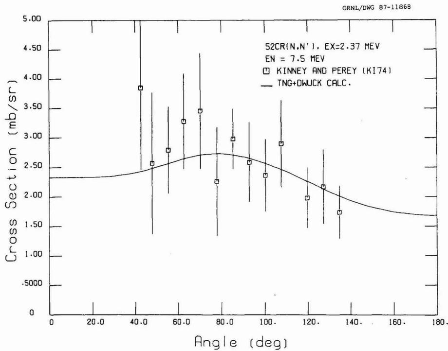
**Fig. 24.** Comparison of calculated and experimental differential cross sections for exciting the 2.37-MeV level at  $E_n = 7.5$  MeV.
