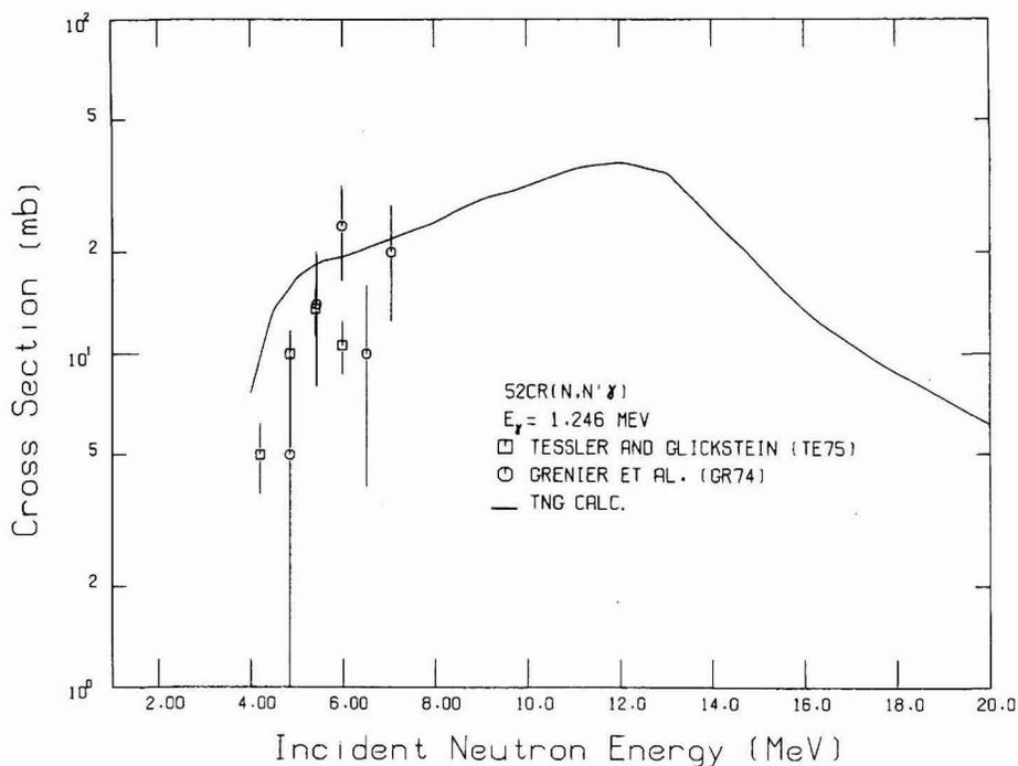
Fig. 45. Comparison of calculated and experimental data of the excitation function for the  $E_\gamma = 1.246 \text{ MeV}$  transition following  $^{52}\text{Cr}(n,n'\gamma)$ .
