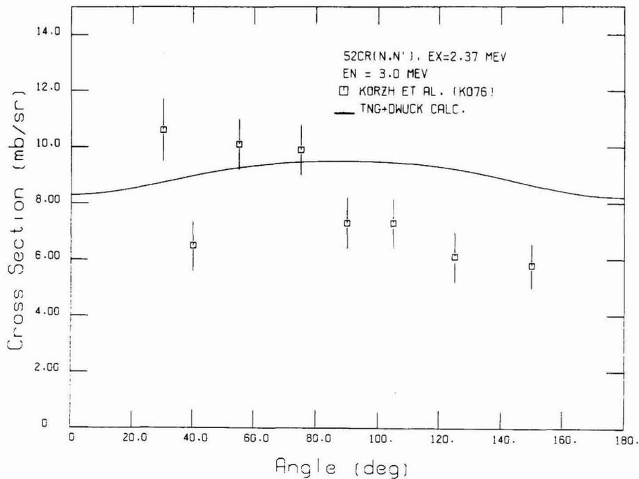
Fig. 21. Comparison of calculated and experimental differential cross sections for exciting the 2.37-MeV level at  $E_n = 3.0$  MeV.
