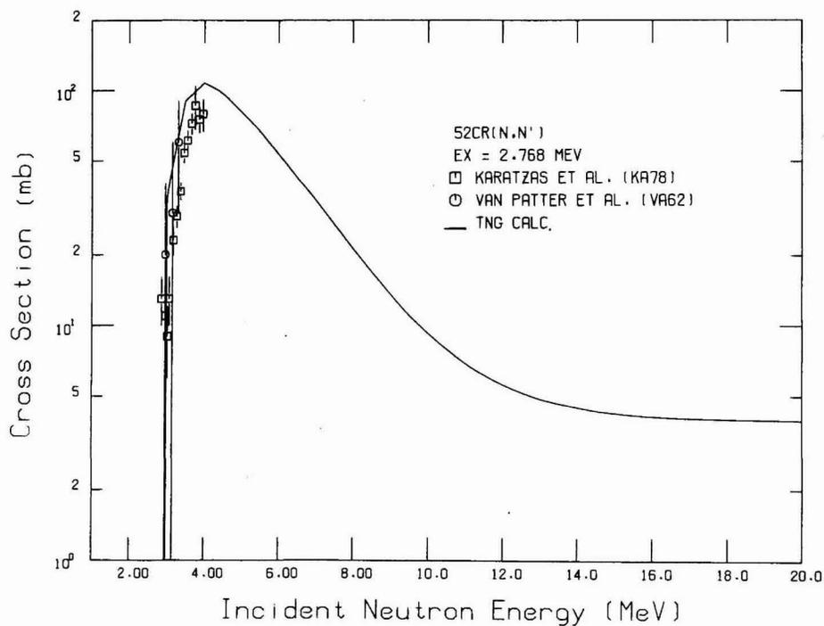
Fig. 29. Comparison of calculated and experimental  $^{52}\text{Cr}(n,n')$  cross sections for exciting the 2.768-MeV level.
