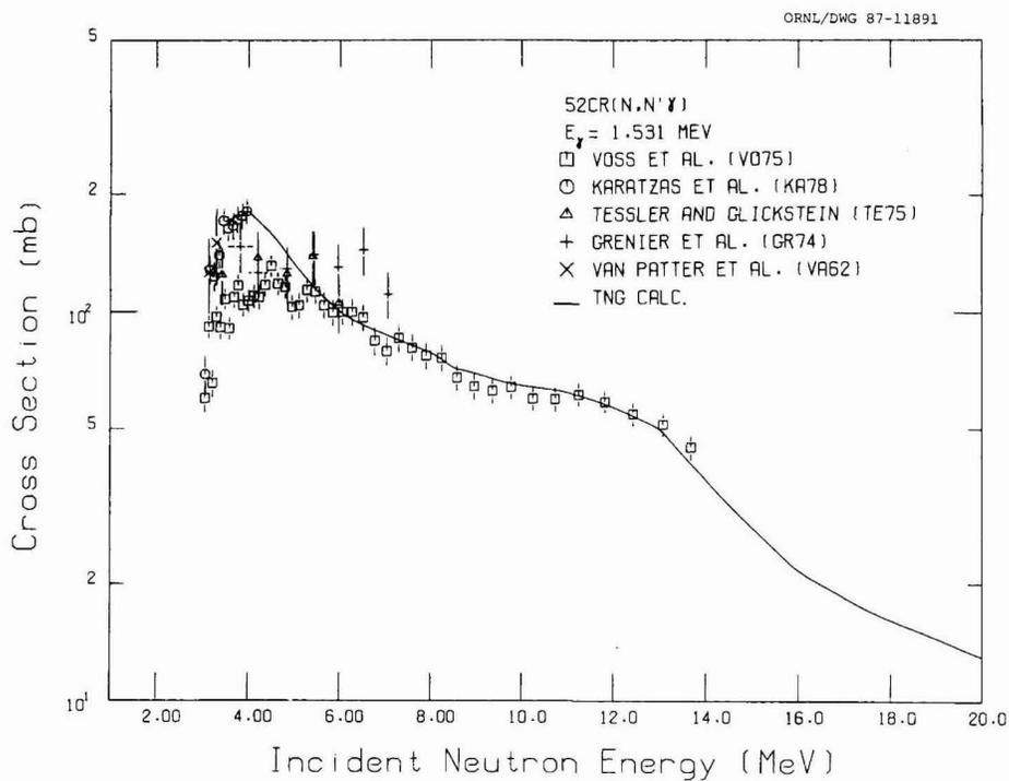
**Fig. 48. Comparison of calculated and experimental data of the excitation function for the  $E_{\gamma} = 1.531$  MeV transition following  $^{52}\text{Cr}(n,n'\gamma)$ .**
