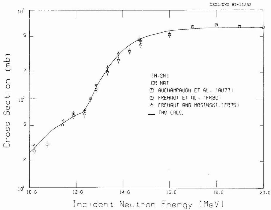
**Fig. 39. Comparison of calculated and experimental  $^{nat}\text{Cr}(n,2n)$  cross sections.**
