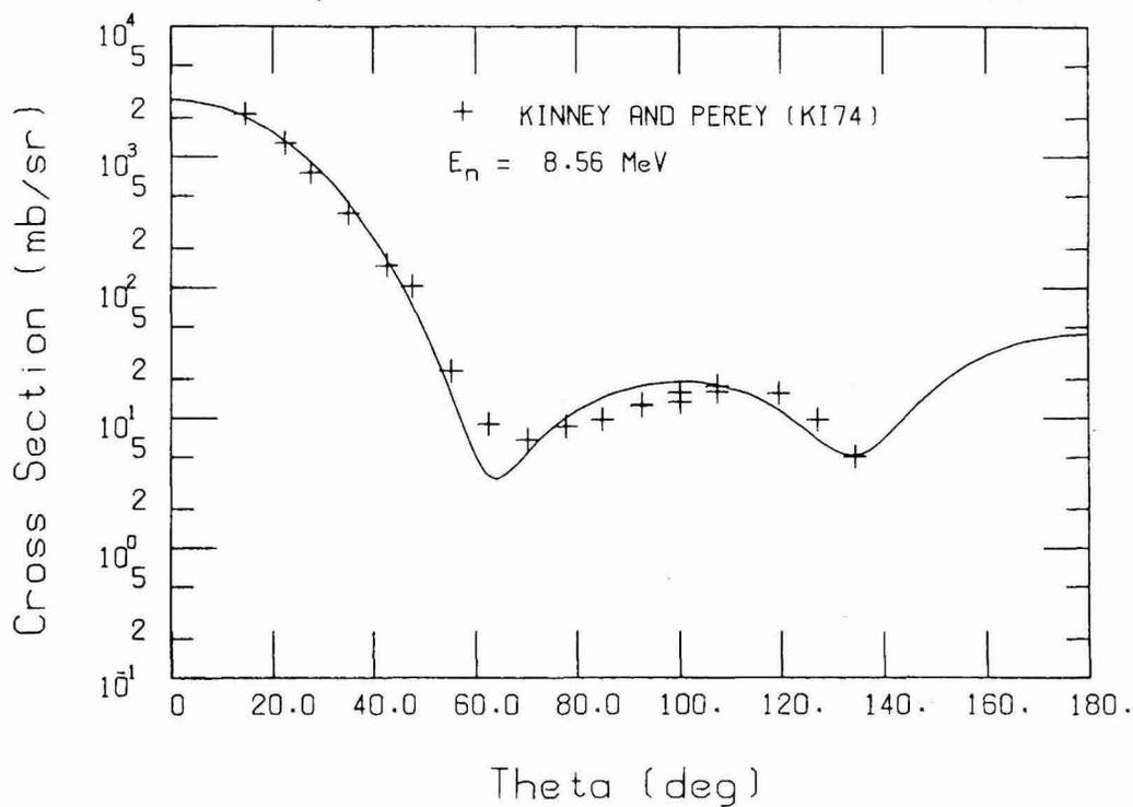
Fig. 8. Comparison of calculated and experimental differential elastic scattering cross sections for  $^{52}\text{Cr}$  at  $E_n = 8.56$  MeV.
