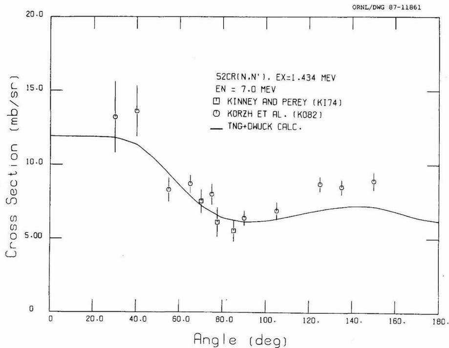
**Fig. 17. Comparison of calculated and experimental differential cross sections for exciting the 1.434-MeV level at  $E_n = 7.0$  MeV.**
