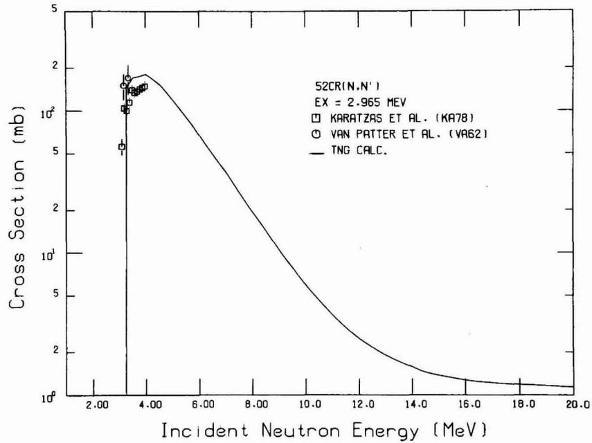
Fig. 30. Comparison of calculated and experimental  $^{52}\text{Cr}(n,n')$  cross sections for exciting the 2.965-MeV level.
