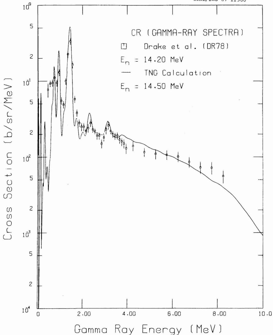
**Fig. 56. Secondary gamma-ray spectra versus gamma-ray energy from the TNG calculation (incident energy  $E_n = 14.5$  MeV) compared with the data of Drake et al. (DR78).**
