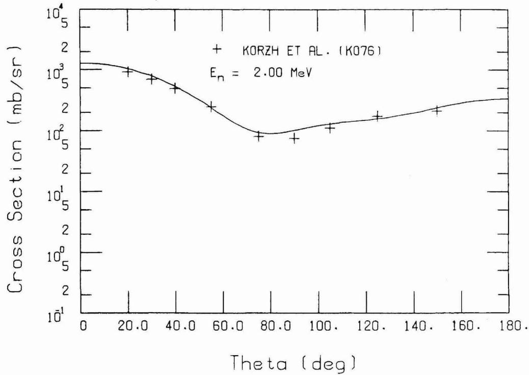
Fig. 6. Comparison of calculated and experimental differential elastic scattering cross sections for  $^{52}\text{Cr}$  at  $E_n = 2.0$  MeV.
