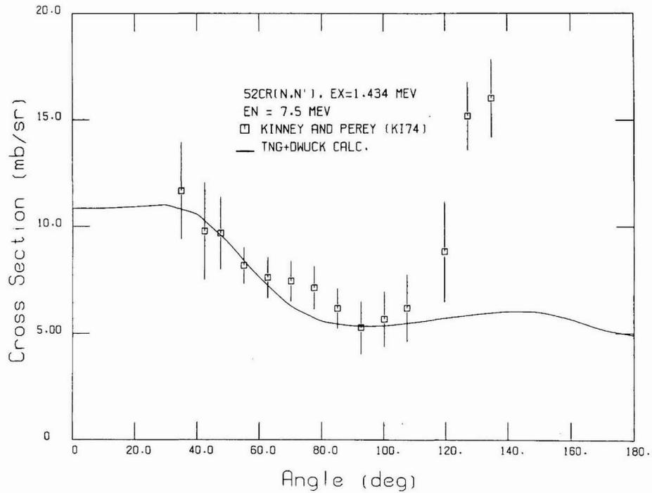
**Fig. 18. Comparison of calculated and experimental differential cross sections for exciting the 1.434-MeV level at  $E_n = 7.5$  MeV.**
