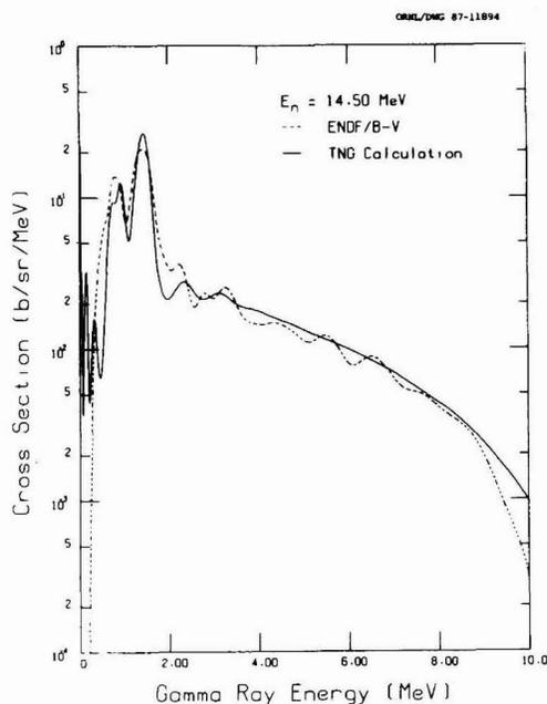
Fig. 67. Comparison of  $(n, x\gamma)$  from ENDF/B-V with the TNG calculation for incident neutron energy of 14.5 MeV.
