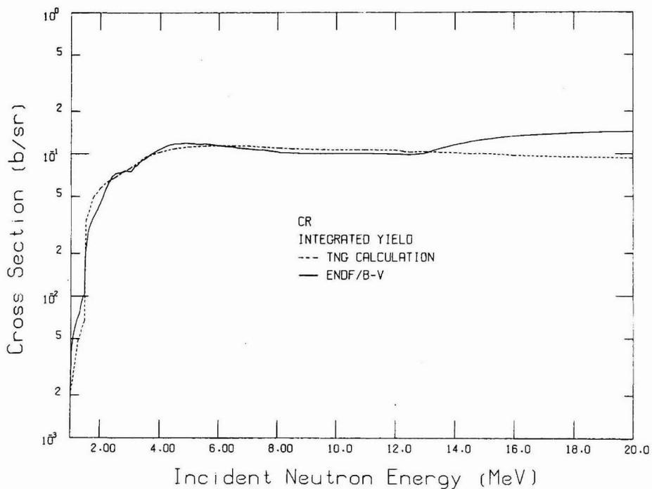
**Fig. 58. Comparison of the TNG calculation with ENDF/B-V for the integrated yield of secondary neutrons as a function of incident neutron energy. The elastic contribution is not included.**
