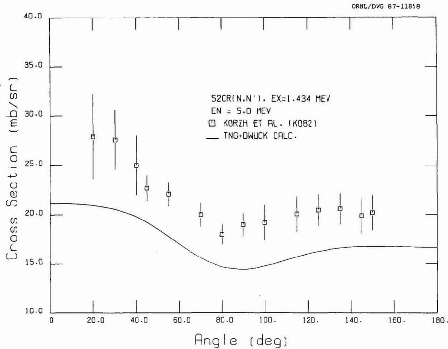
**Fig. 14.** Comparison of calculated and experimental differential cross sections for exciting the 1.434-MeV level at  $E_n = 5.0$  MeV.
