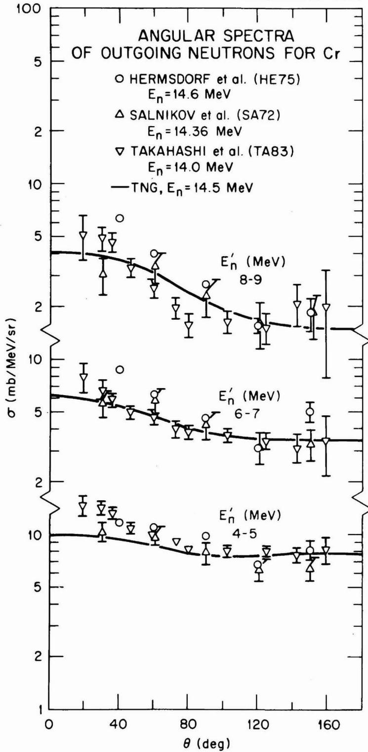
**Fig. 32. Comparison of calculated and experimental neutron production cross sections.**
