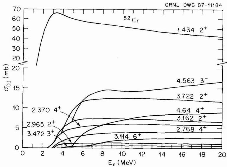
**Fig. 1. Calculated direct inelastic excitation cross sections for  $^{52}\text{Cr}$ .**
