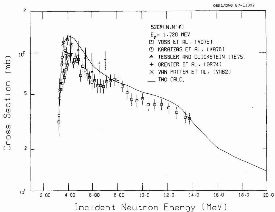
Fig. 49. Comparison of calculated and experimental data of the excitation function for the  $E_\gamma = 1.728 \text{ MeV}$  transition following  $^{52}\text{Cr}(n,n'\gamma)$ .
