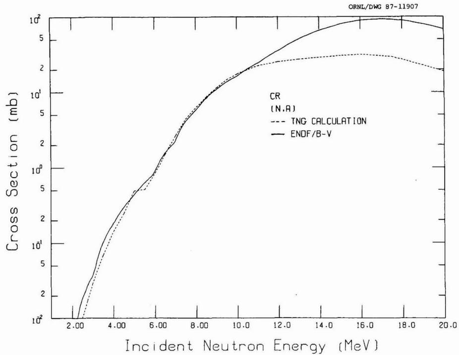
**Fig. 63. Comparison of the TNG calculation with ENDF/B-V for the  $(n,\alpha)$  cross section.**
