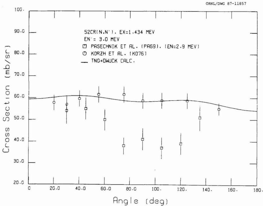
**Fig. 13. Comparison of calculated and experimental differential cross sections for exciting the 1.434-MeV level at  $E_n = 3.0$  MeV.**
