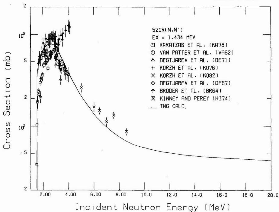
Fig. 26. Comparison of calculated and experimental  $^{52}\text{Cr}(n,n')$  cross sections for exciting the 1.434-MeV level.
