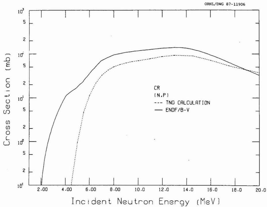
**Fig. 62. Comparison of the TNG calculation with ENDF/B-V for the  $(n, p)$  cross section.**
