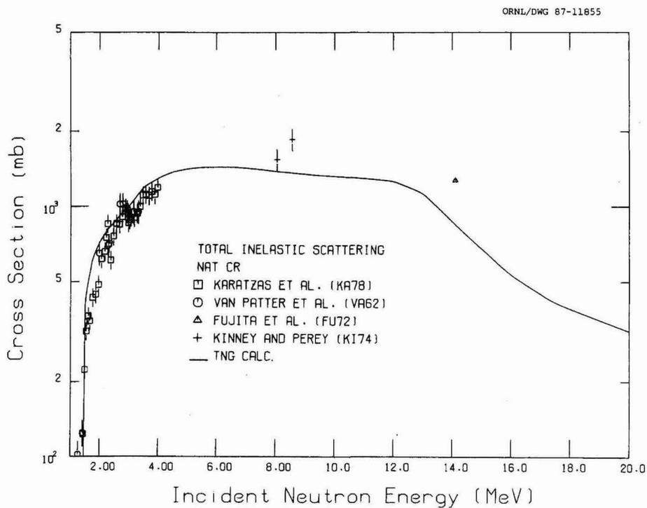
**Fig. 11. Comparison of calculated and experimental total inelastic scattering cross sections for  $^{\text{nat}}\text{Cr}$ .**
