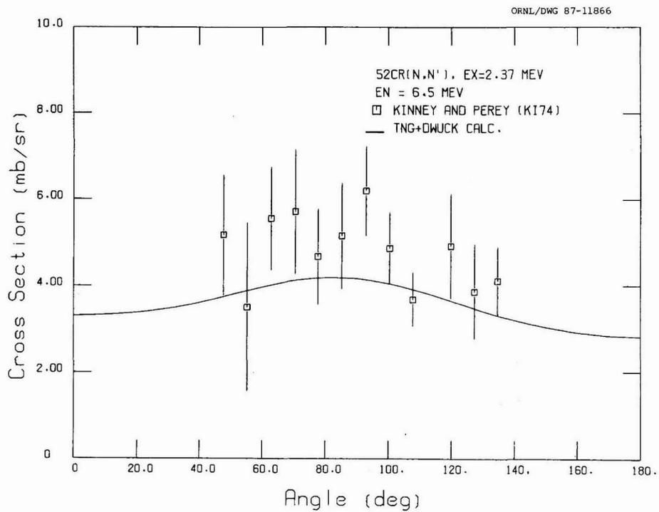
**Fig. 22.** Comparison of calculated and experimental differential cross sections for exciting the 2.37-MeV level at  $E_n = 6.5$  MeV.
