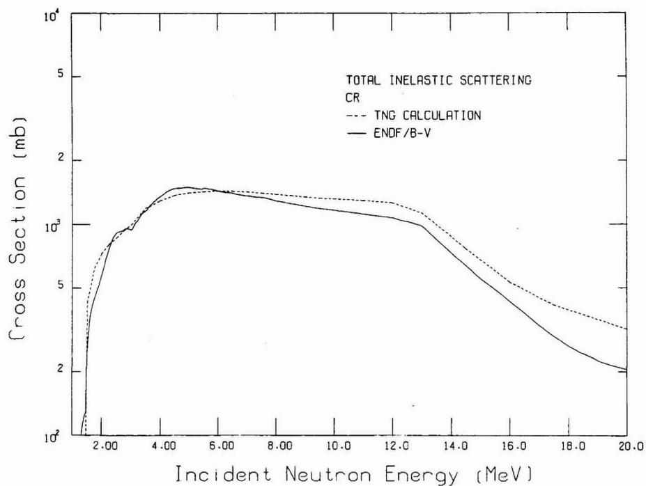
**Fig. 57. Comparison of the TNG calculation with ENDF/B-V for the total inelastic scattering cross section.**
