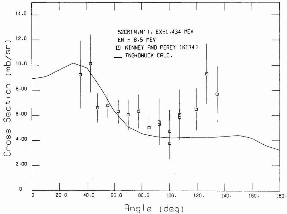
Fig. 20. Comparison of calculated and experimental differential cross sections for exciting the 1.434-MeV level at  $E_n = 8.5$  MeV.
