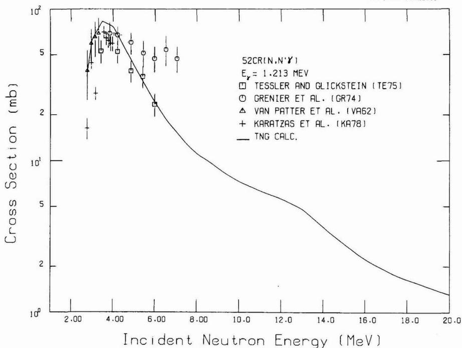
Fig. 46. Comparison of calculated and experimental data of the excitation function for the  $E_\gamma = 1.213 \text{ MeV}$  transition following  $^{52}\text{Cr}(n,n'\gamma)$ .
