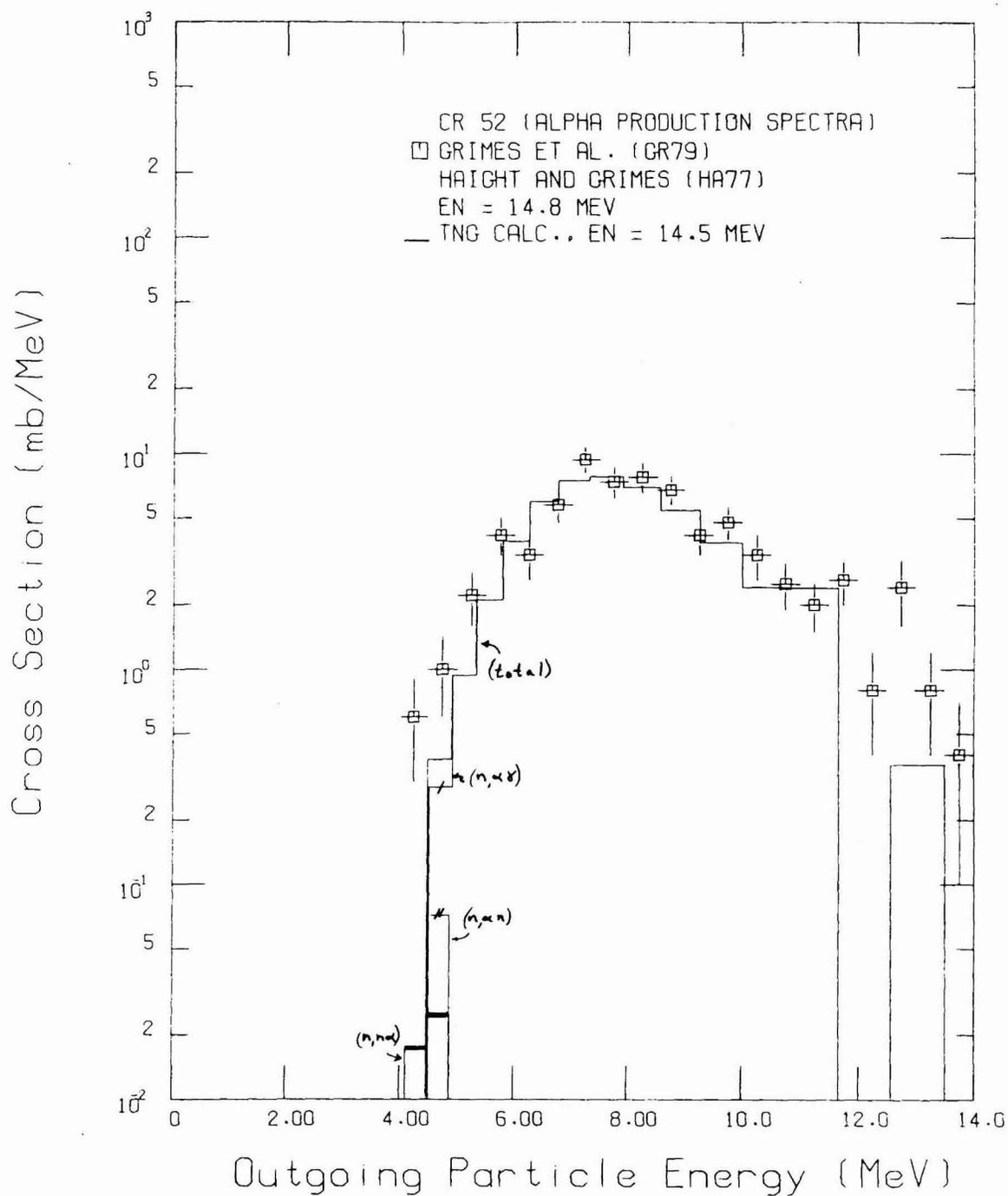
Fig. 35. Comparison of calculated and experimental alpha production spectra for  $^{52}\text{Cr}$ . The measurement was taken at an incident energy of 14.8 MeV, the TNG calculation was for  $E_n = 14.5$  MeV.
