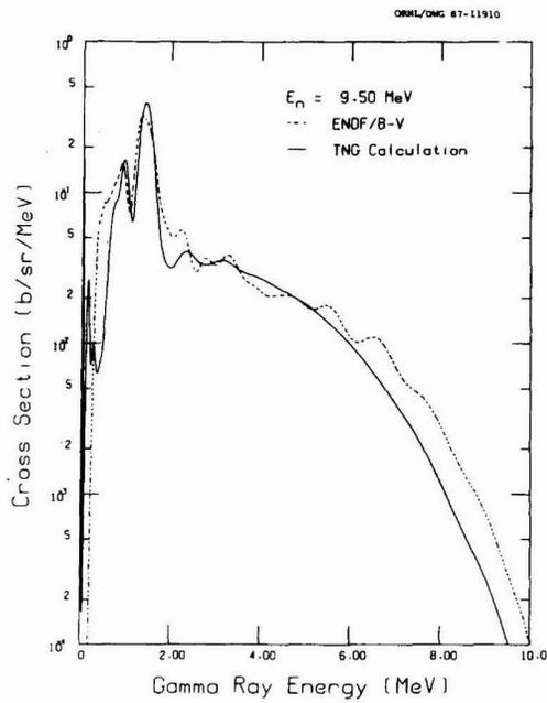
Fig. 66. Comparison of  $(n, x\gamma)$  from ENDF/B-V with the TNG calculation for incident neutron energy of 9.5 MeV.
