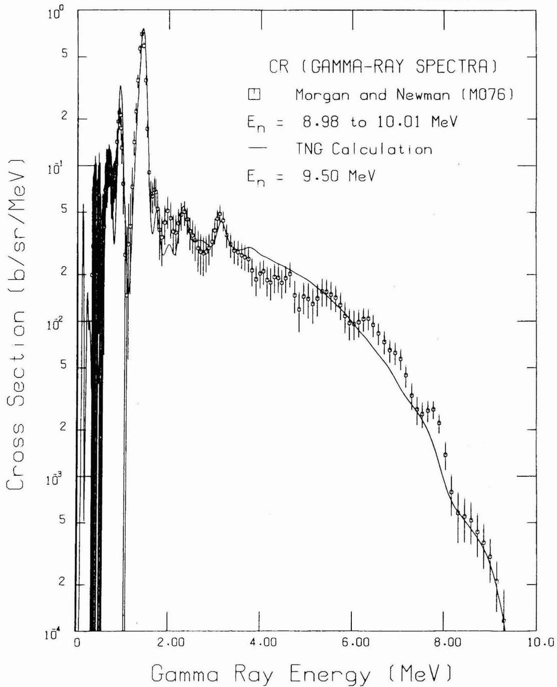
**Fig. 54. Secondary gamma-ray spectra versus gamma-ray energy from the TNG calculation (incident energy  $E_n = 9.5$  MeV) compared with the data of Morgan and Newman (M076).**
