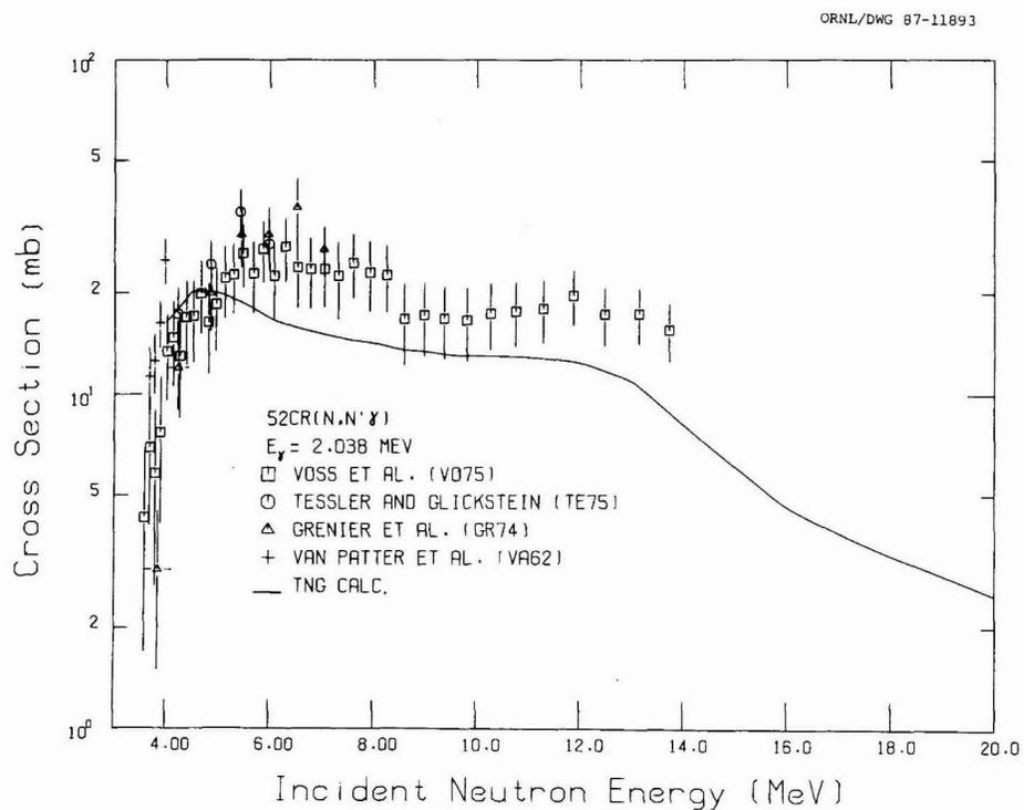
Fig. 50. Comparison of calculated and experimental data of the excitation function for the  $E_\gamma = 2.038 \text{ MeV}$  transition following  $^{52}\text{Cr}(n,n'\gamma)$ .
