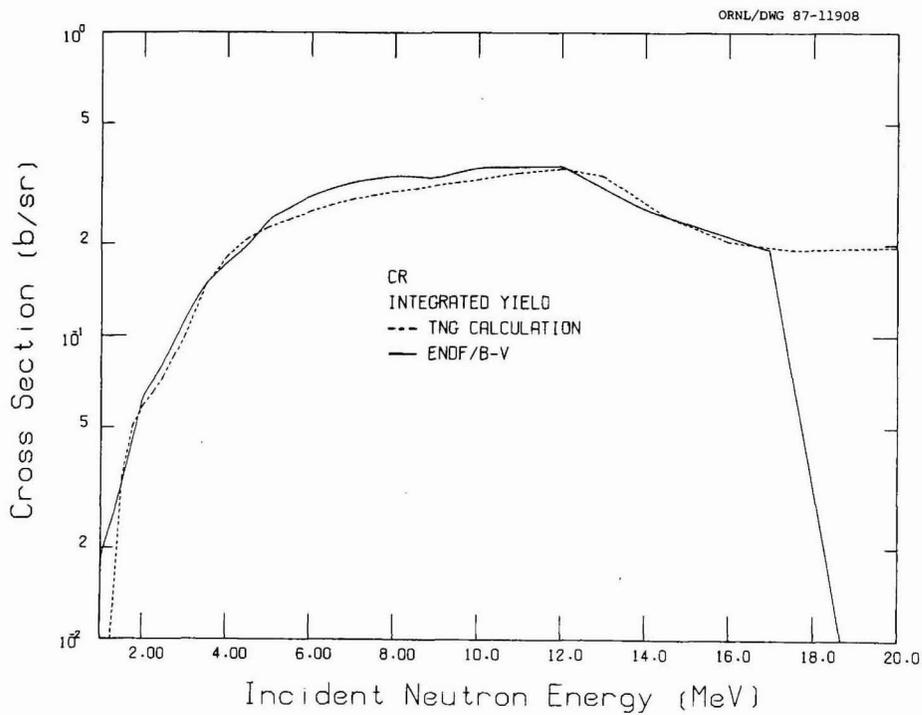
**Fig. 64. Comparison of the TNG calculation with ENDF/B-V for the integrated yield of secondary gamma rays as a function of incident neutron energy.**
