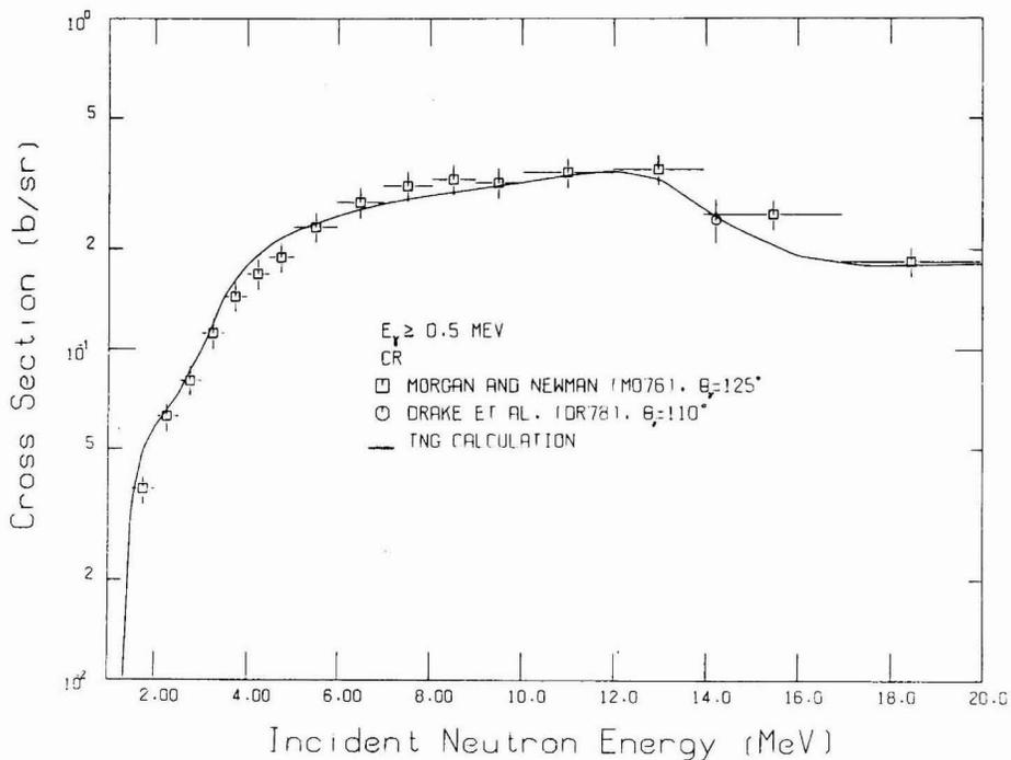
**Fig. 52.** Integrated yield of secondary gamma rays with  $E_\gamma \geq 0.5$  MeV as a function of incident neutron energy. Gamma-ray scattering angles  $\theta_\gamma$  are given in the legend.
