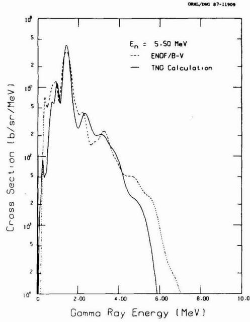
Fig. 65. Comparison of  $(n, x\gamma)$  from ENDF/B-V with the TNG calculation for incident neutron energy of 5.5 MeV.
