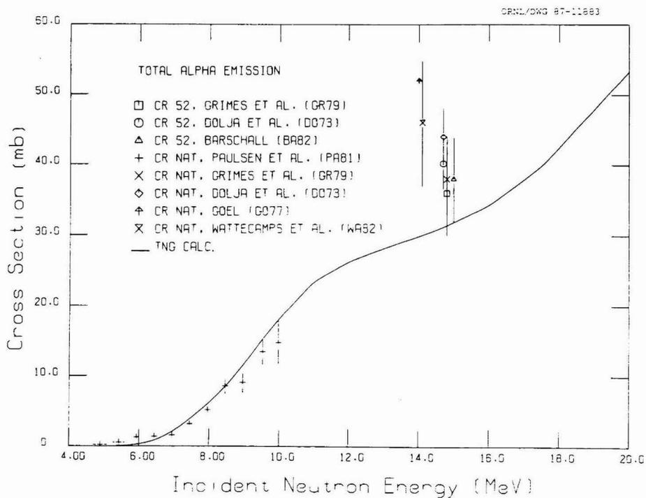
**Fig. 40. Comparison of calculated ( $^{52}\text{Cr}$ ) and experimental ( $^{52}\text{Cr}$  and  $^{nat}\text{Cr}$ ) cross sections for the total alpha emission.**
