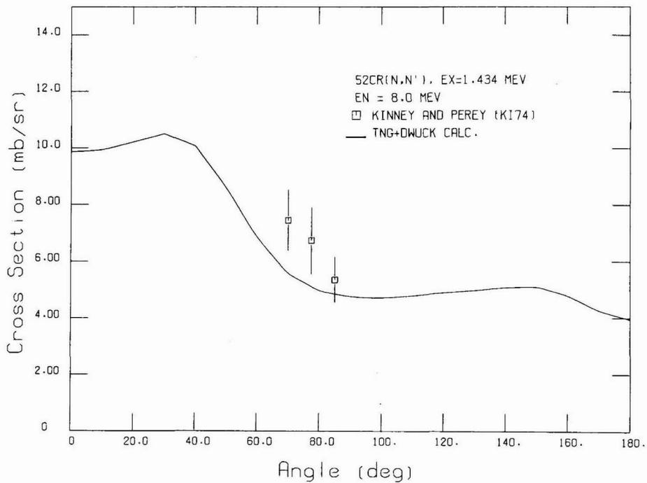
**Fig. 19. Comparison of calculated and experimental differential cross sections for exciting the 1.434-MeV level at  $E_n = 8.0$  MeV.**
