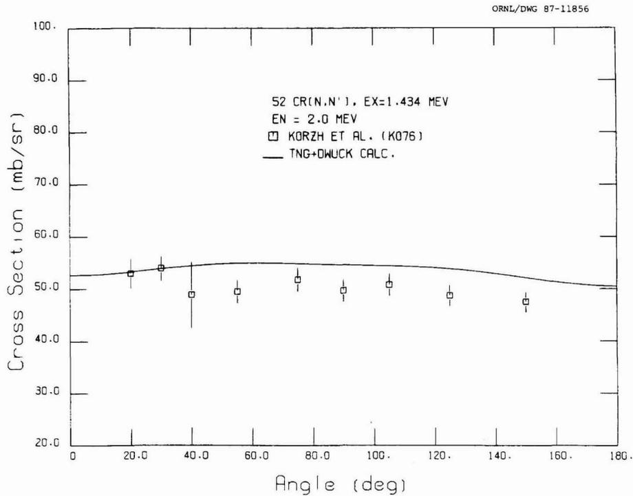
**Fig. 12. Comparison of calculated and experimental differential cross sections for exciting the 1.434-MeV level at  $E_n = 2.0$  MeV.**
