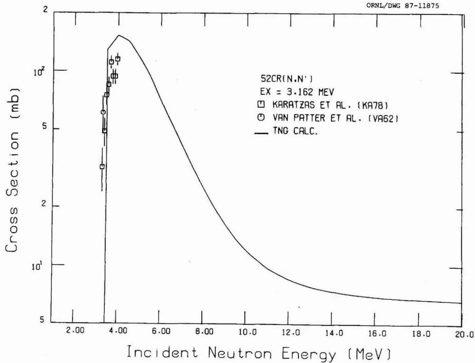
Fig. 31. Comparison of calculated and experimental  $^{52}\text{Cr}(n,n')$  cross sections for exciting the 3.162-MeV level.
