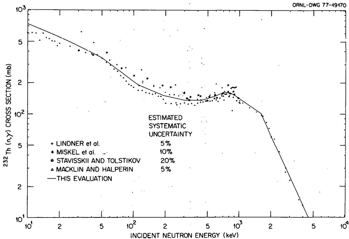
Fig. 4. Comparison of several measurements of the  $^{232}\text{Th}(n,\gamma)$  cross section with the present evaluation in the range 10 keV to 4 MeV. The data have been renormalized as described in the text.
