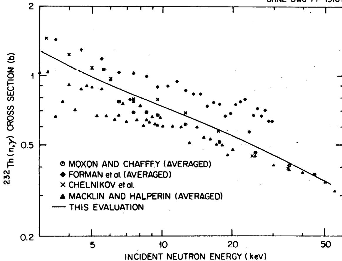
Fig. 1. Comparison of several measurements of the  $^{232}\text{Th}(n,\gamma)$  cross section with the present evaluation in the range 3 to 50 keV. The data have been renormalized as described in the text.
