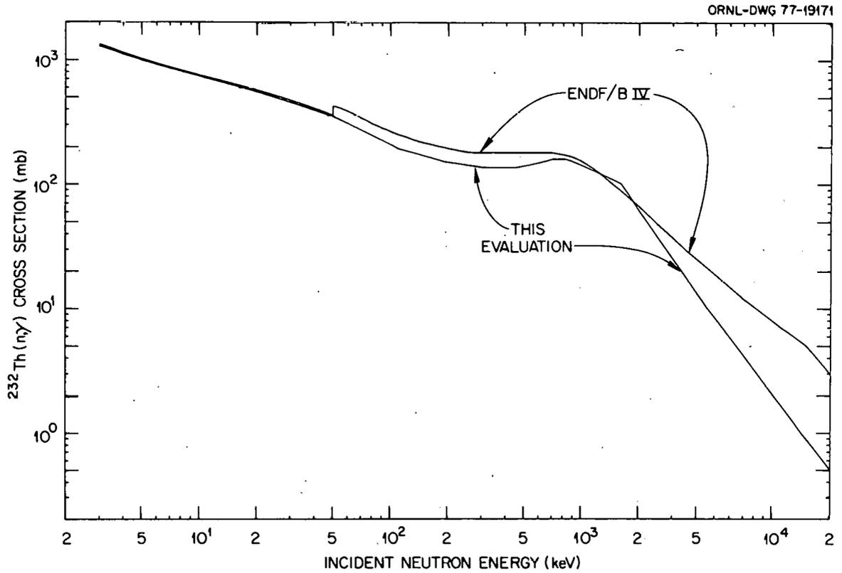
Fig. 6.  $^{232}\text{Th}(n,\gamma)$  cross section. Comparison of this evaluation with ENDF/B-IV.
