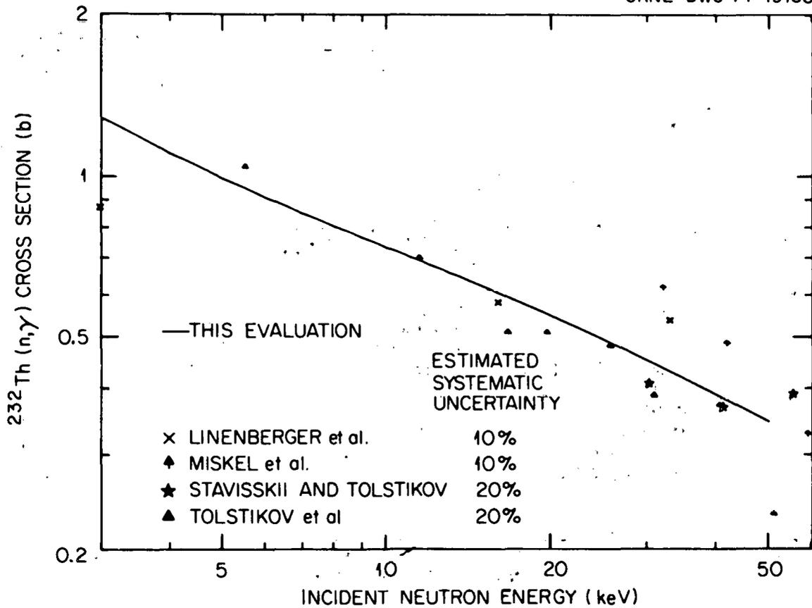
Fig. 2. Comparison of several measurements of the  $^{232}\text{Th}(n,\gamma)$  cross section with the present evaluation in the range 3 to 50 keV. The data have been renormalized as described in the text.
