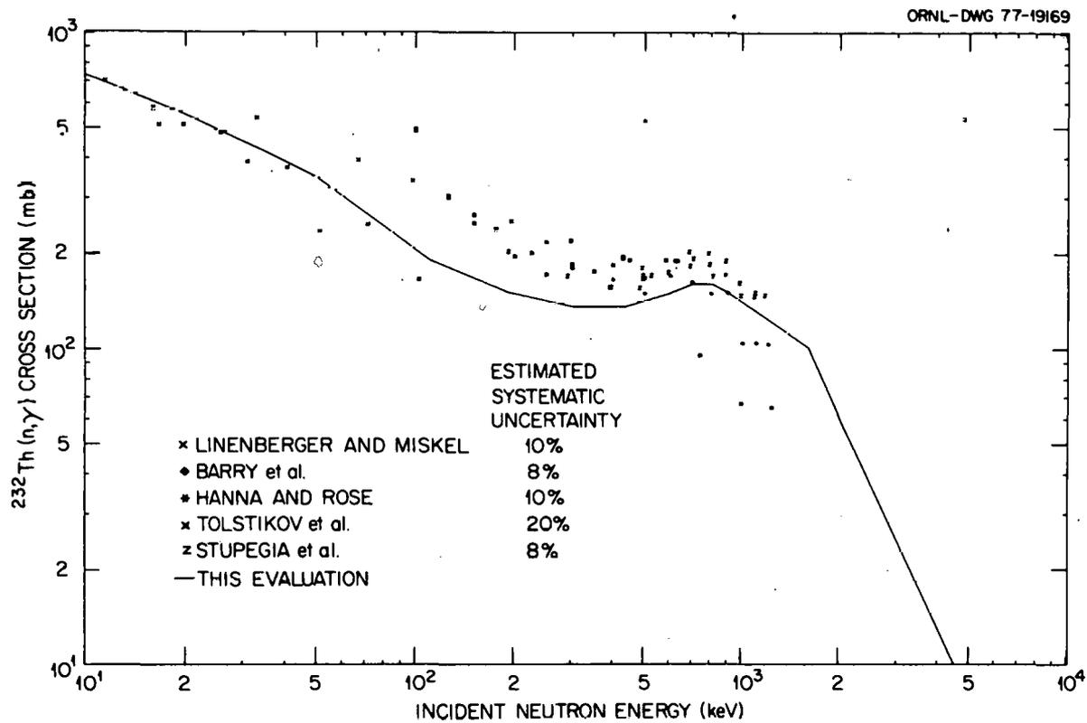
Fig. 3. Comparison of several measurements of the  $^{232}\text{Th}(n,\gamma)$  cross section with the present evaluation in the range 10 keV to 4 MeV. The data have been renormalized as described in the text.
