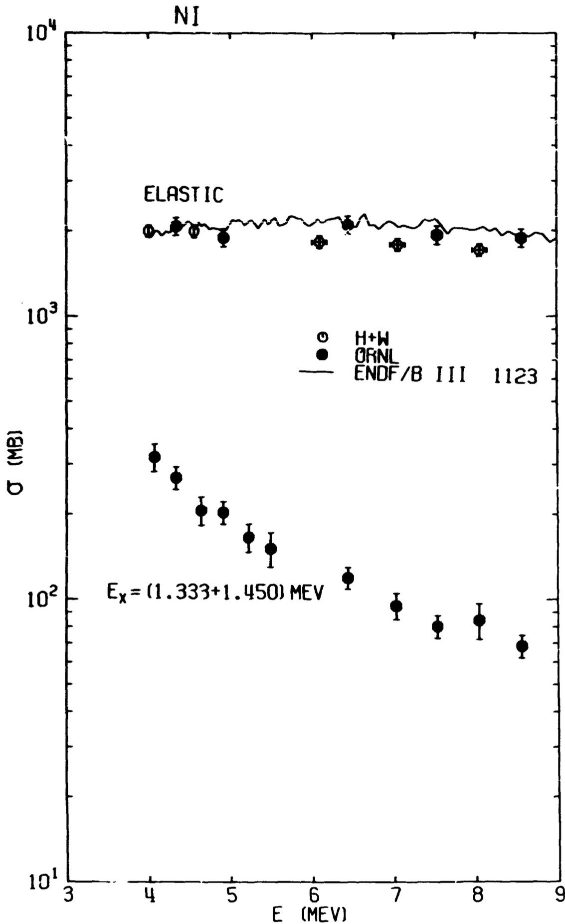
Fig. 11. Our angle-integrated cross sections for neutron elastic scattering on natural nickel and cross sections per atom of natural nickel for inelastic scattering to both the 1.333 MeV level in  $^{60}\text{Ni}$  and the 1.450 MeV level in  $^{58}\text{Ni}$  as a function of incident neutron energy. Elastic data of Holmqvist and Wiedling (H+W)<sup>2</sup> are shown. The curve is from ENDF/B III M... 1123.
