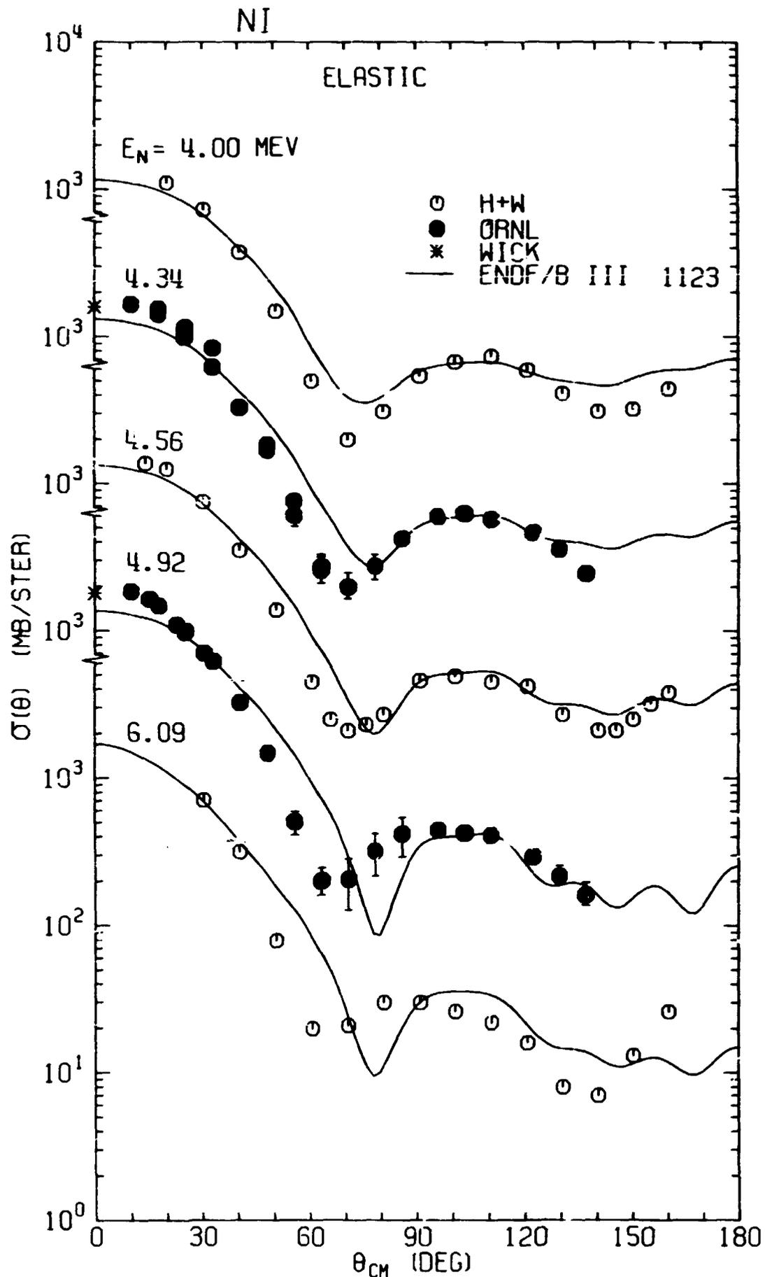
Fig. 3. Our natural nickel neutron differential elastic center-of-mass cross sections compared with the data of Holmqvist and Wiedling  $(H+W)^2$  and with the angular distributions of ENDF/B III MAT 1123 from 4.00 to 6.09 MeV. WICK indicates Wick's Limit. The 7% uncertainty in absolute normalization common to all points is not included in the error bars.
