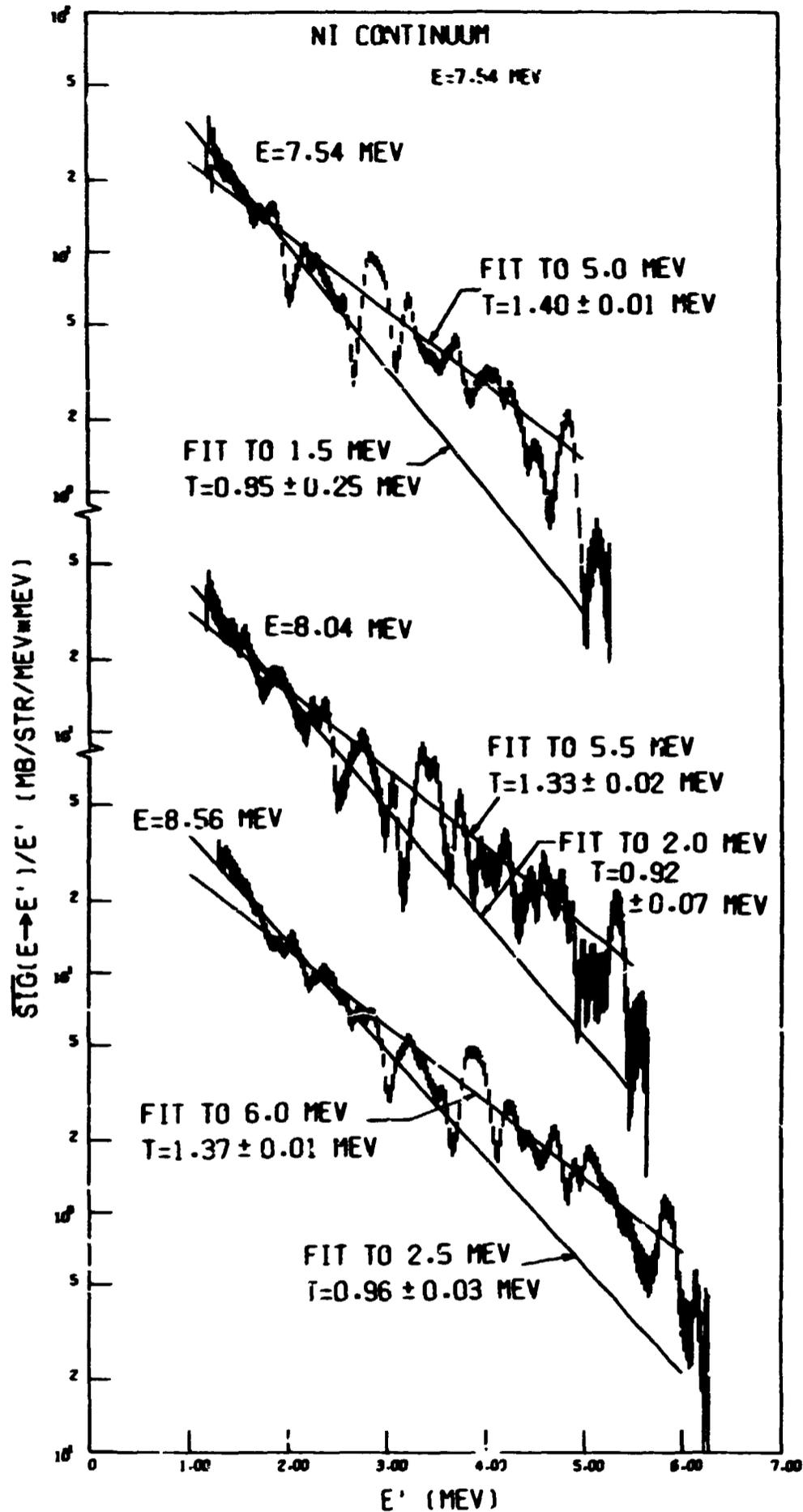
Fig. 14. Natural nickel angle-averaged cross sections for inelastic scattering to the continuum divided by the out-going neutron energy,  $E'$ , as a function of out-going neutron energy for incident neutron energies,  $E$ , from 7.54 to 8.56 MeV. Least squares fits were made to two different indicated upper limits in  $E'$  for each set of data with resulting temperatures,  $T$ , being shown. The lower value of  $E'$  was equal to the lowest value of the data in all cases.
