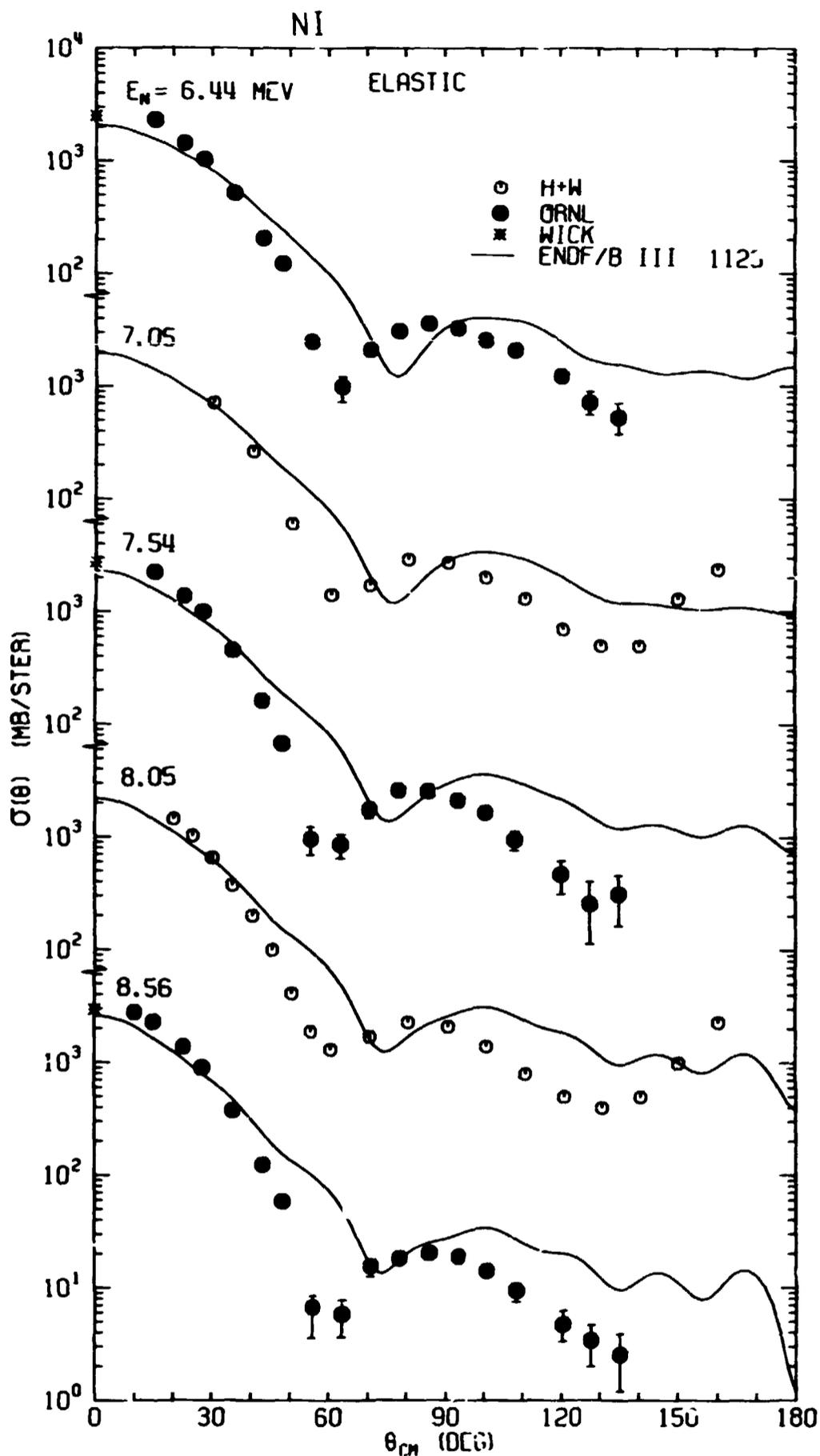
Fig. 4. Our natural nickel neutron differential elastic center-of-mass cross sections compared with the data of Holmqvist and Wiedling (H+W)<sup>2</sup> and with the angular distributions of ENDF/B III MAT 1123 from 6.44 to 8.56 MeV. WICK indicates Wick's Limit. The 7% uncertainty in absolute normalization common to all points is not included in the error bars.
