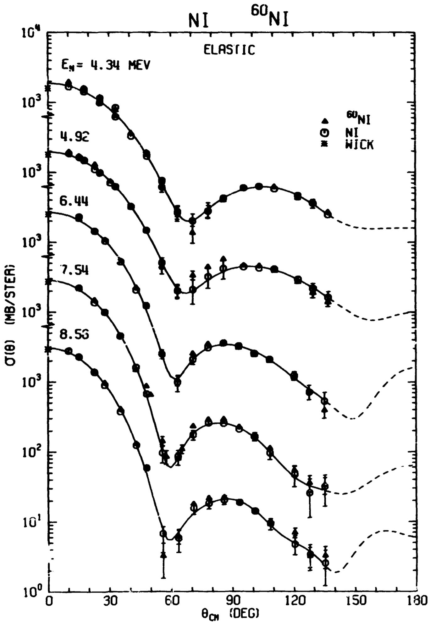
Fig. 8. A comparison of our natural nickel and <sup>60</sup>Ni neutron differential elastic center-of-mass scattering cross sections with least squares Legendre fits to the natural nickel data.
