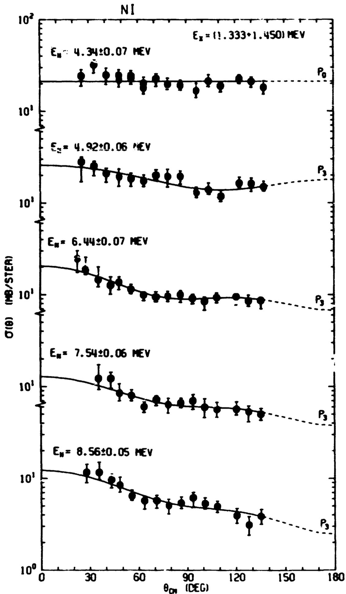
Fig. 9. Our differential center-of-mass cross sections per atom of natural nickel for combined neutron inelastic scattering to the 1.333 MeV level in  $^{60}\text{Ni}$  and to the 1.450 MeV level in  $^{58}\text{Ni}$ . The curves are least squares Legendre fits to the data.
