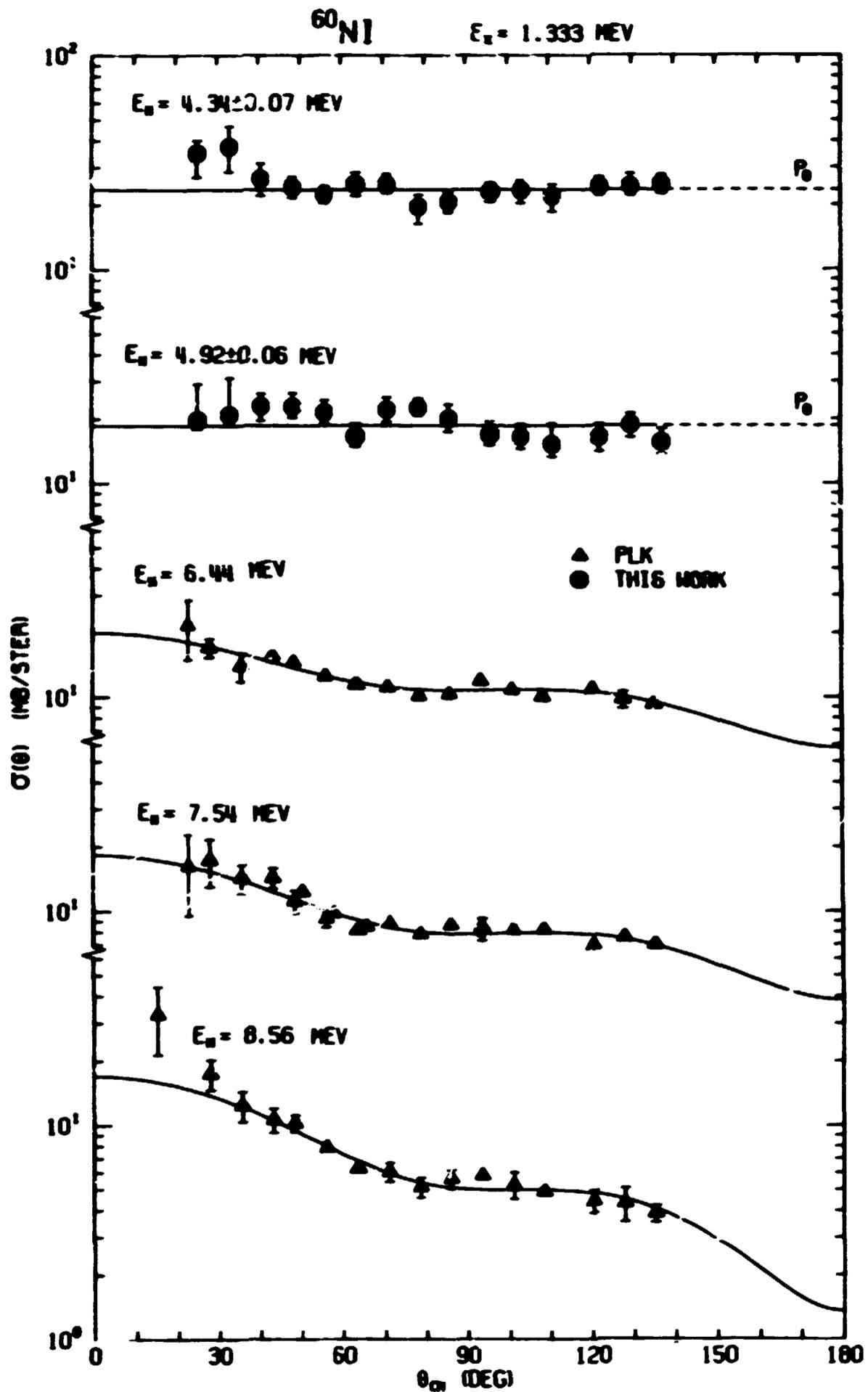
Fig. 10. Our differential center-of-mass cross sections for neutron inelastic scattering to the 1.333 MeV level in  $^{60}\text{Ni}$ . The cross sections are per atom of  $^{60}\text{Ni}$ . The curves result from least squares Legendre fits to the data.
