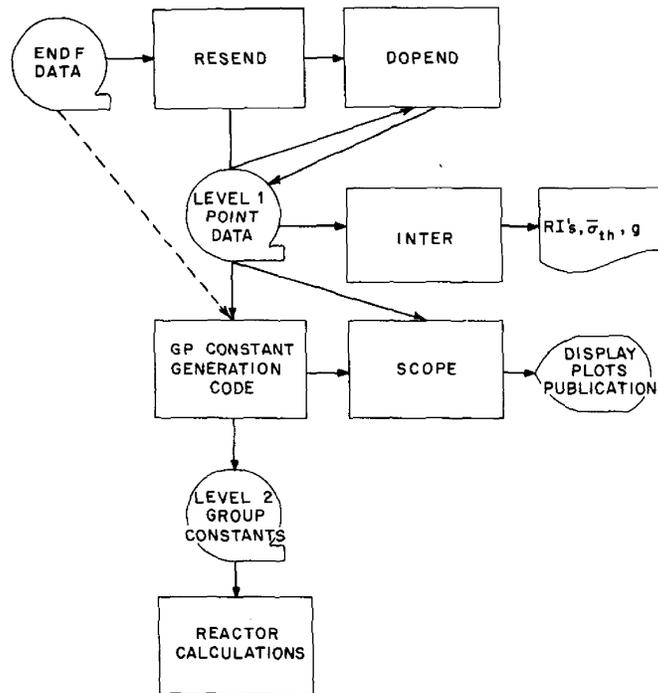
Figure 4. Generation and Application of Pre-Processed Data Files.
