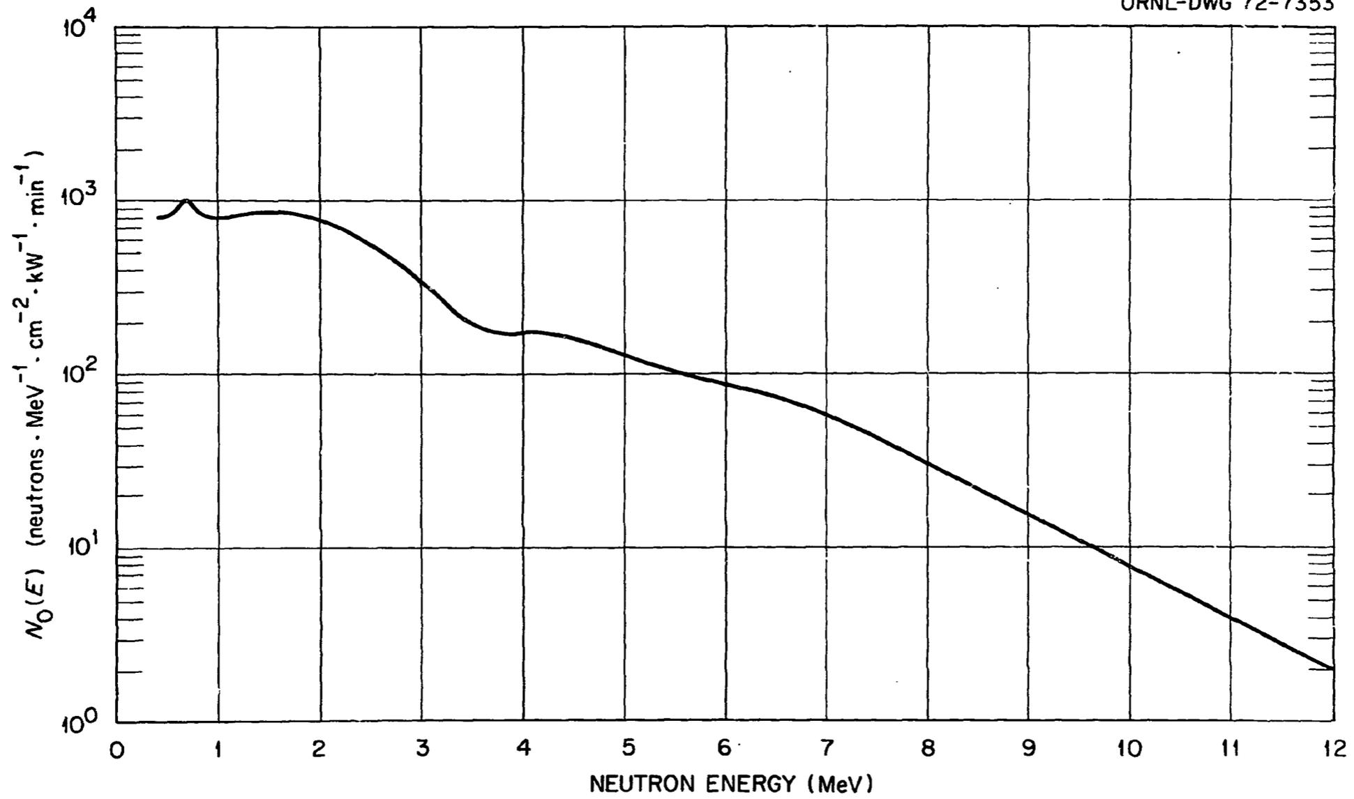
Fig. 3. Source Spectrum for Oxygen.
