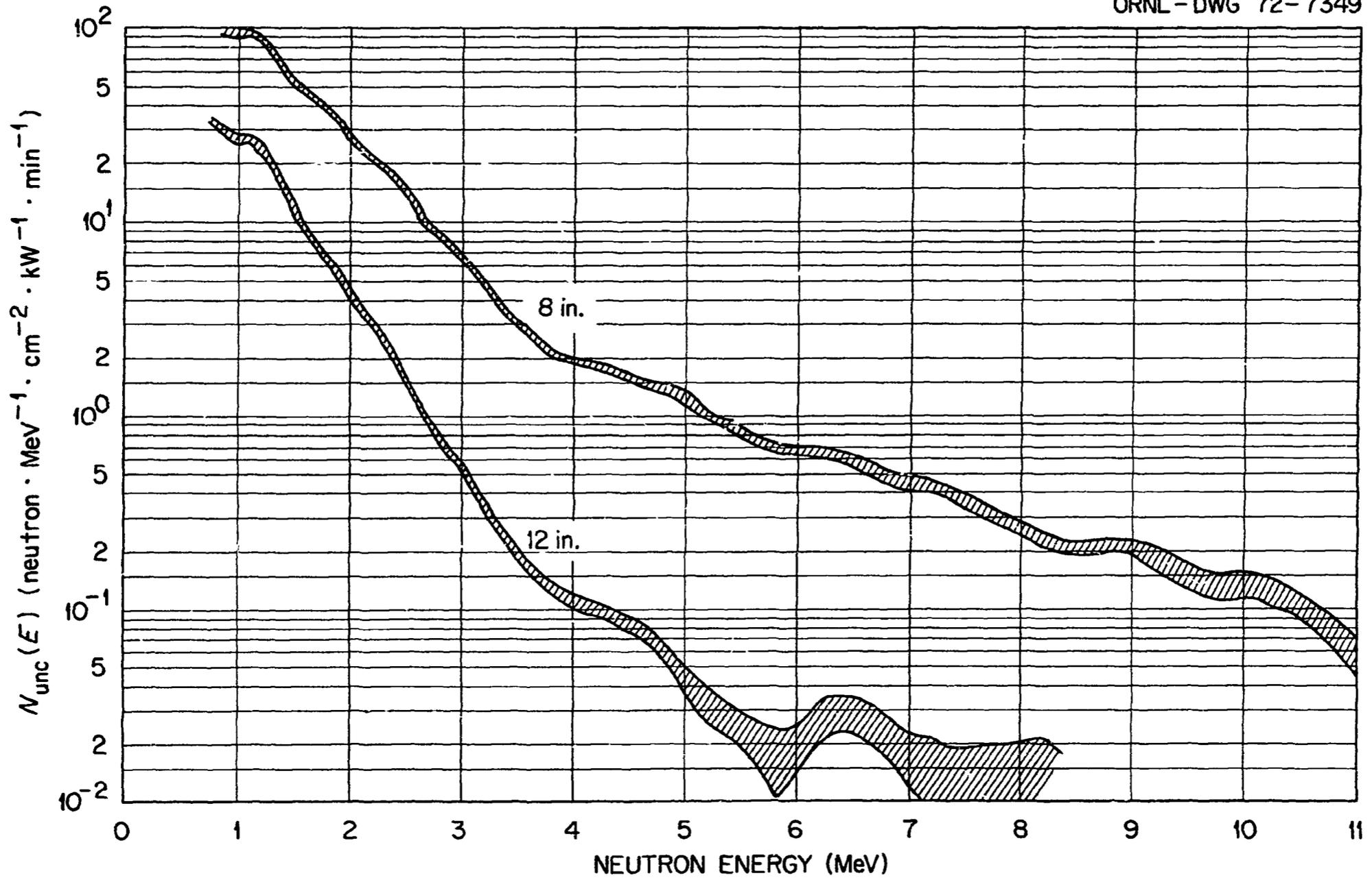
Fig. 2. Transmitted Spectrum Through Iron.
