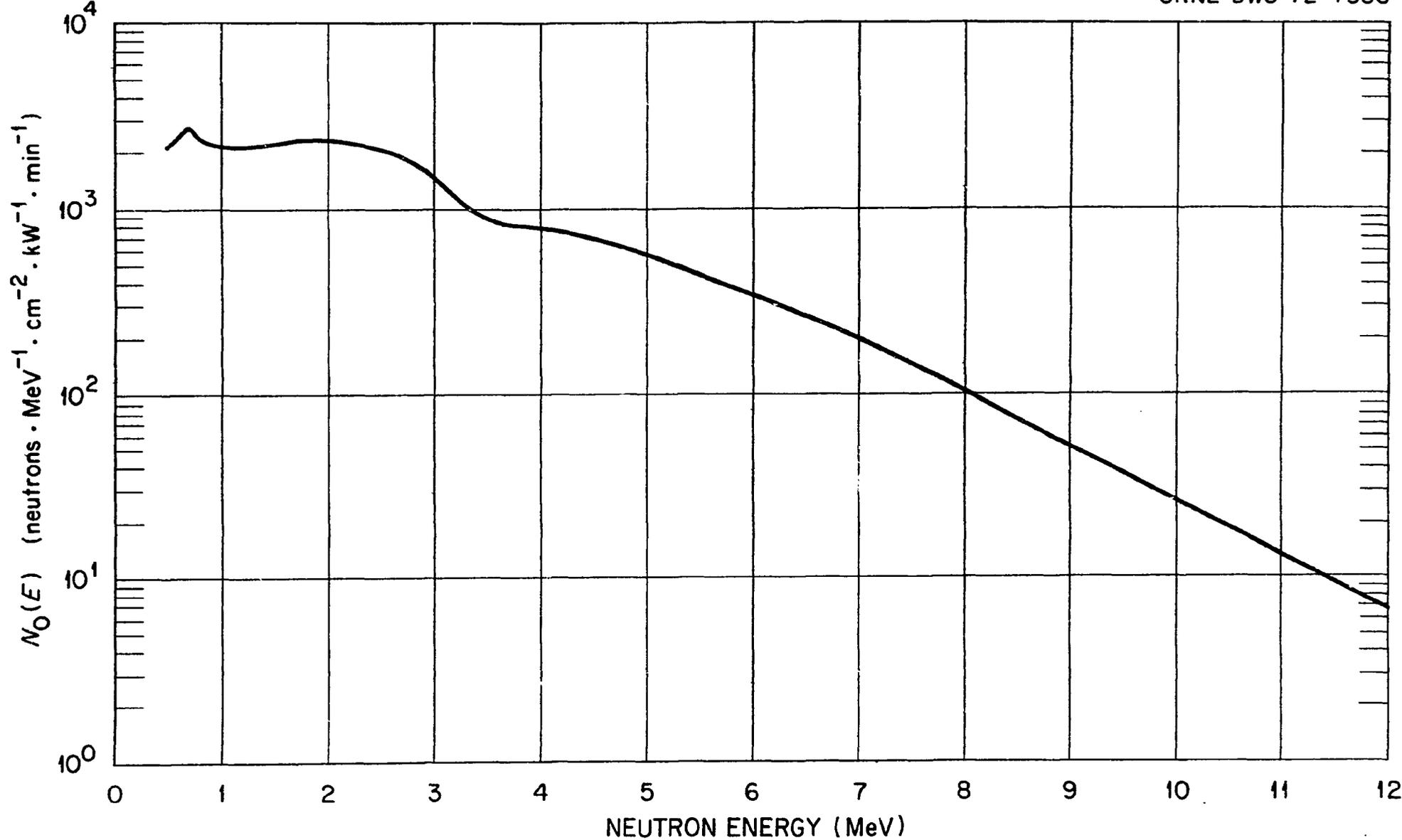
Fig. 3. Source Spectrum for Iron.
