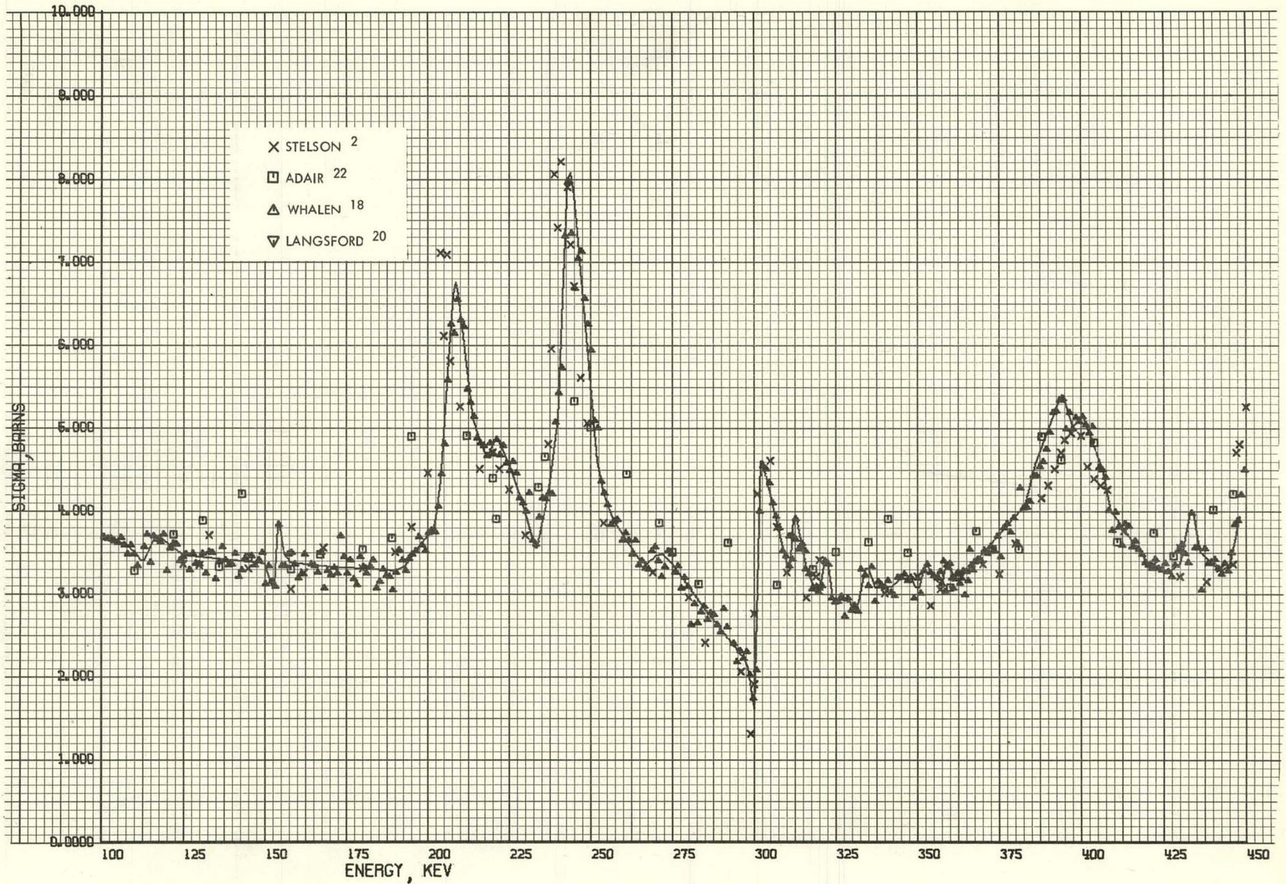
FIG. 4 TOTAL CROSS SECTION, 0.10 TO 0.45 MEV
