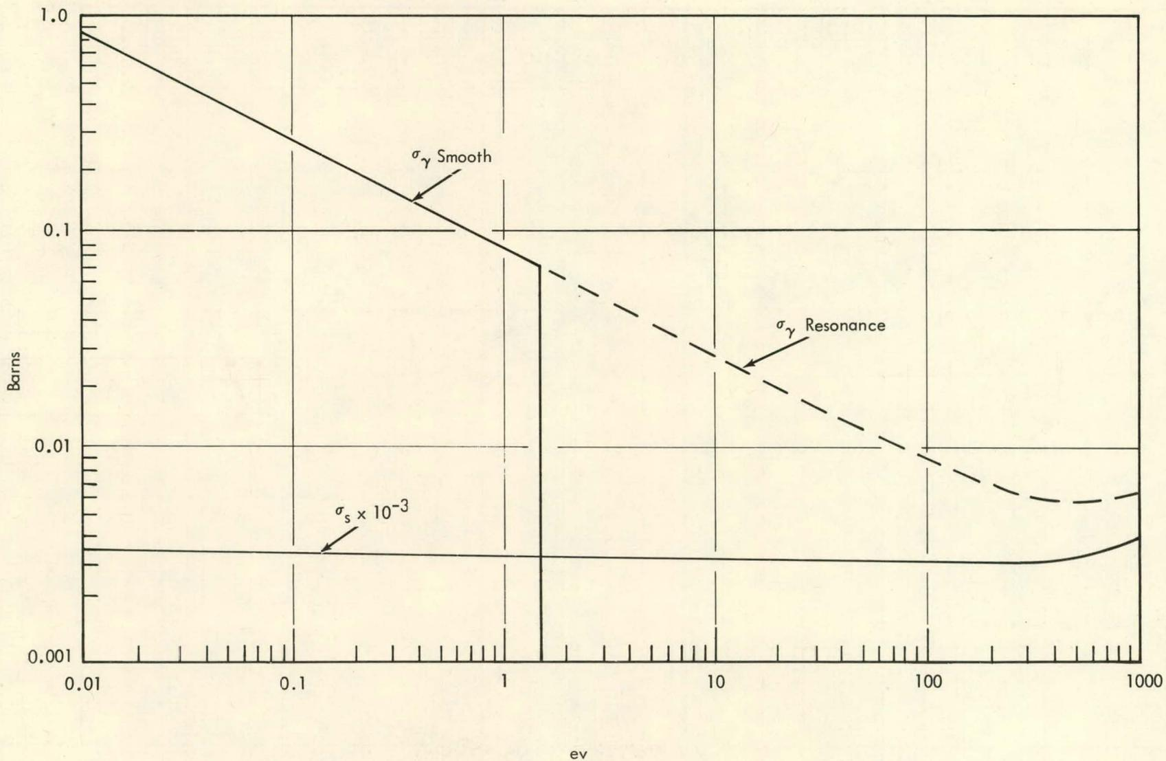
FIG. 3 SCATTERING AND CAPTURE CROSS SECTIONS, 0.01 TO 1000 EV
