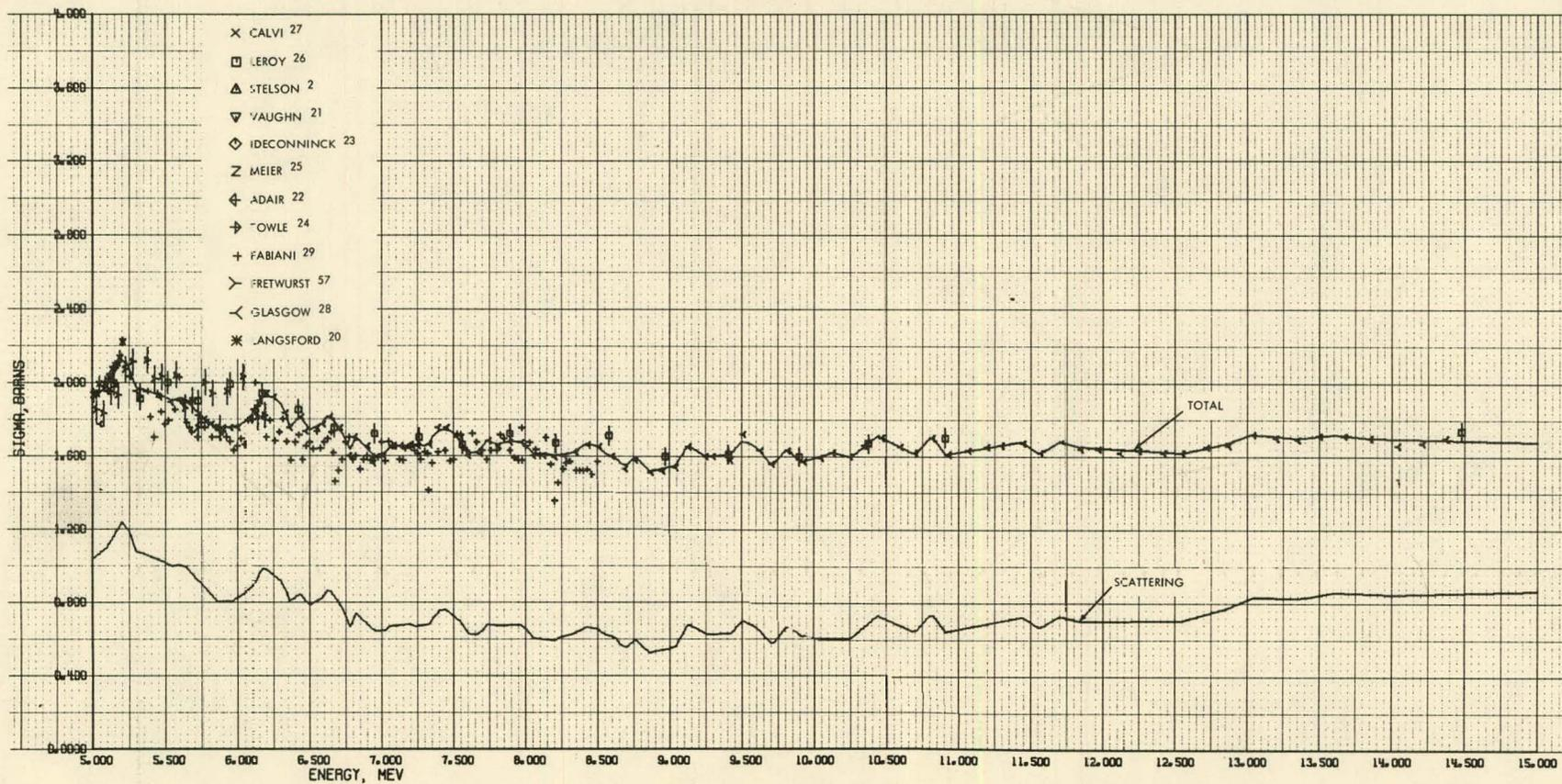
FIG. 8 TOTAL AND SCATTERING CROSS SECTION, 5.0 TO 15.0 MEV
