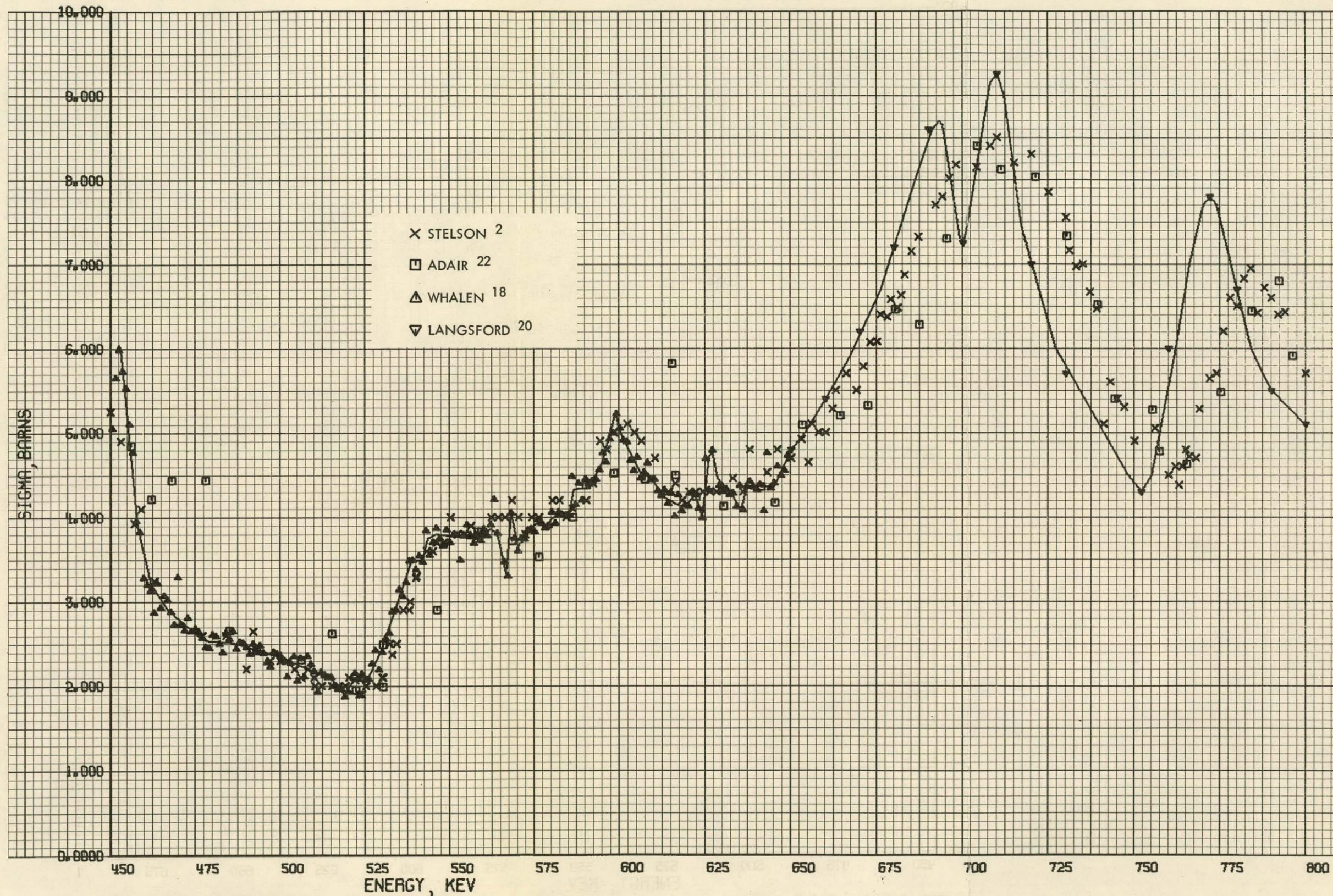
FIG. 5 TOTAL CROSS SECTION, 0.45 TO 0.80 MEV
