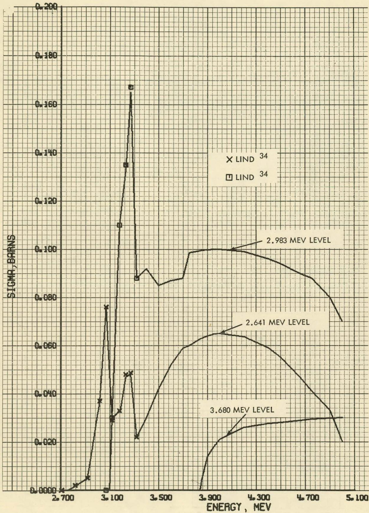
FIG. 13 INELASTIC SCATTERING CROSS SECTIONS, 2.641, 2.983, AND 3.680 MEV LEVELS
