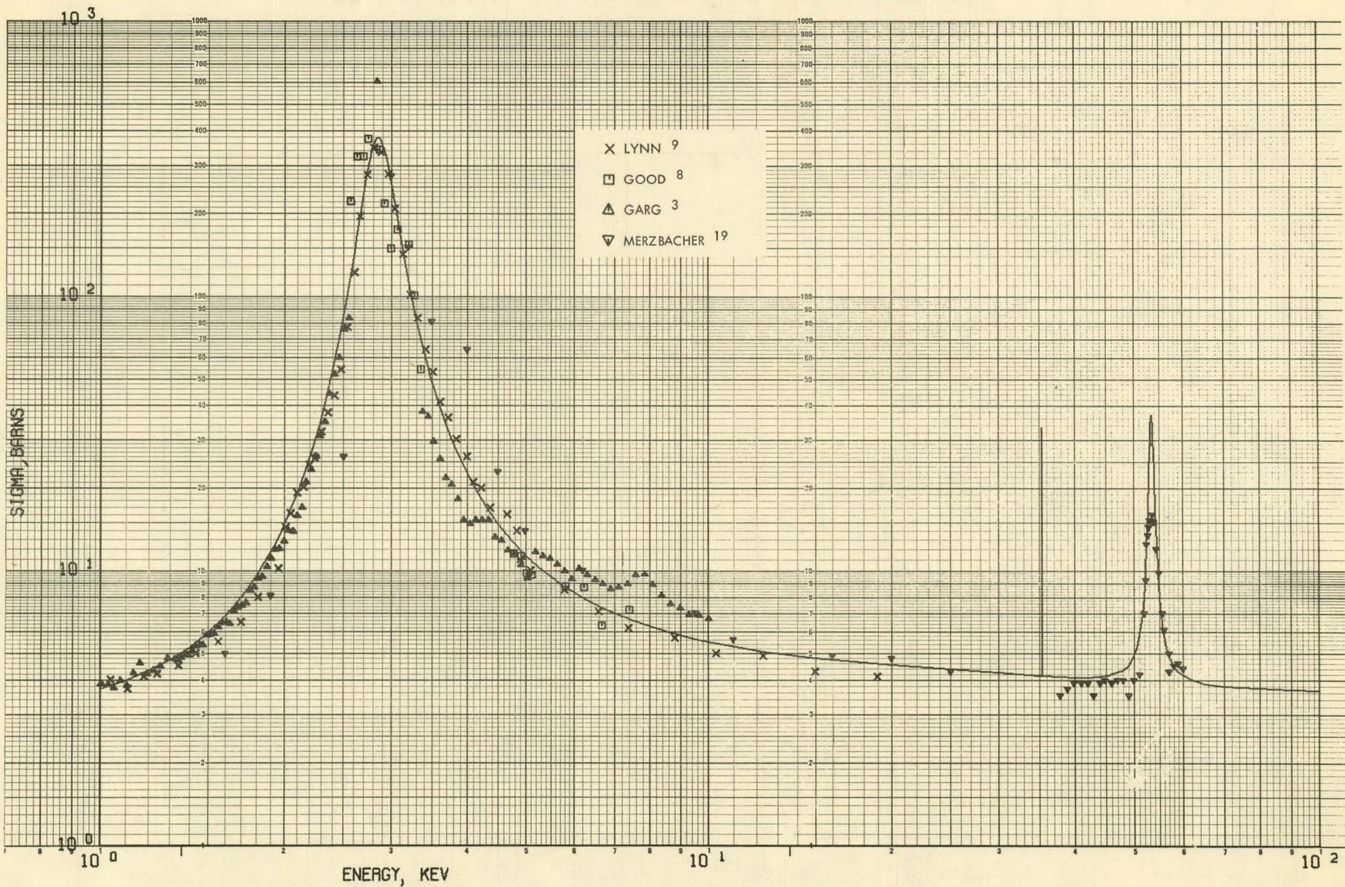
FIG. 2 EVALUATED TOTAL CROSS SECTION, 1 TO 100 KEV
