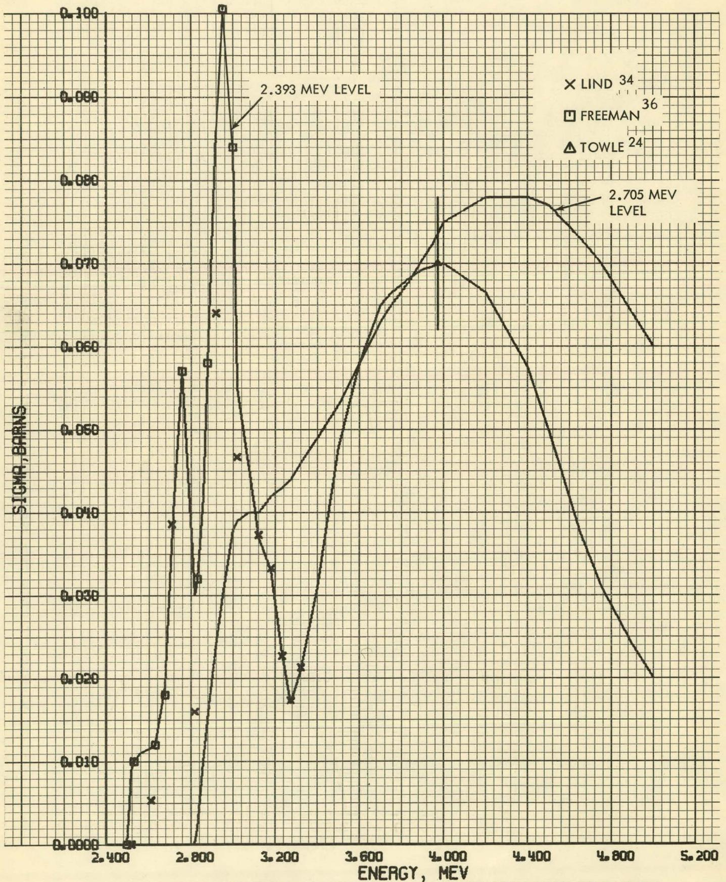
FIG. 12 INELASTIC SCATTERING CROSS SECTIONS, 2.393 AND 2.705 MEV LEVELS
