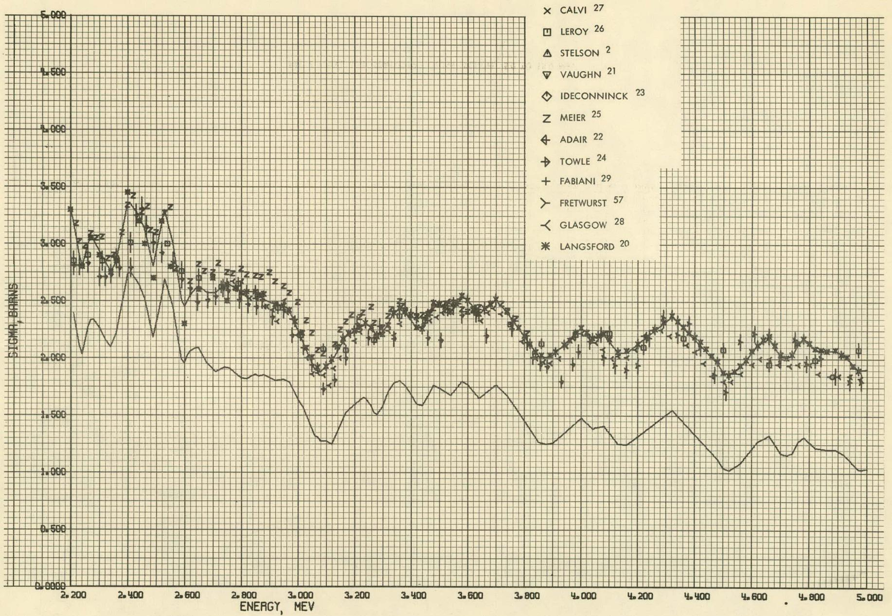
FIG. 7 TOTAL AND SCATTERING CROSS SECTION, 2.2 TO 5.0 MEV
