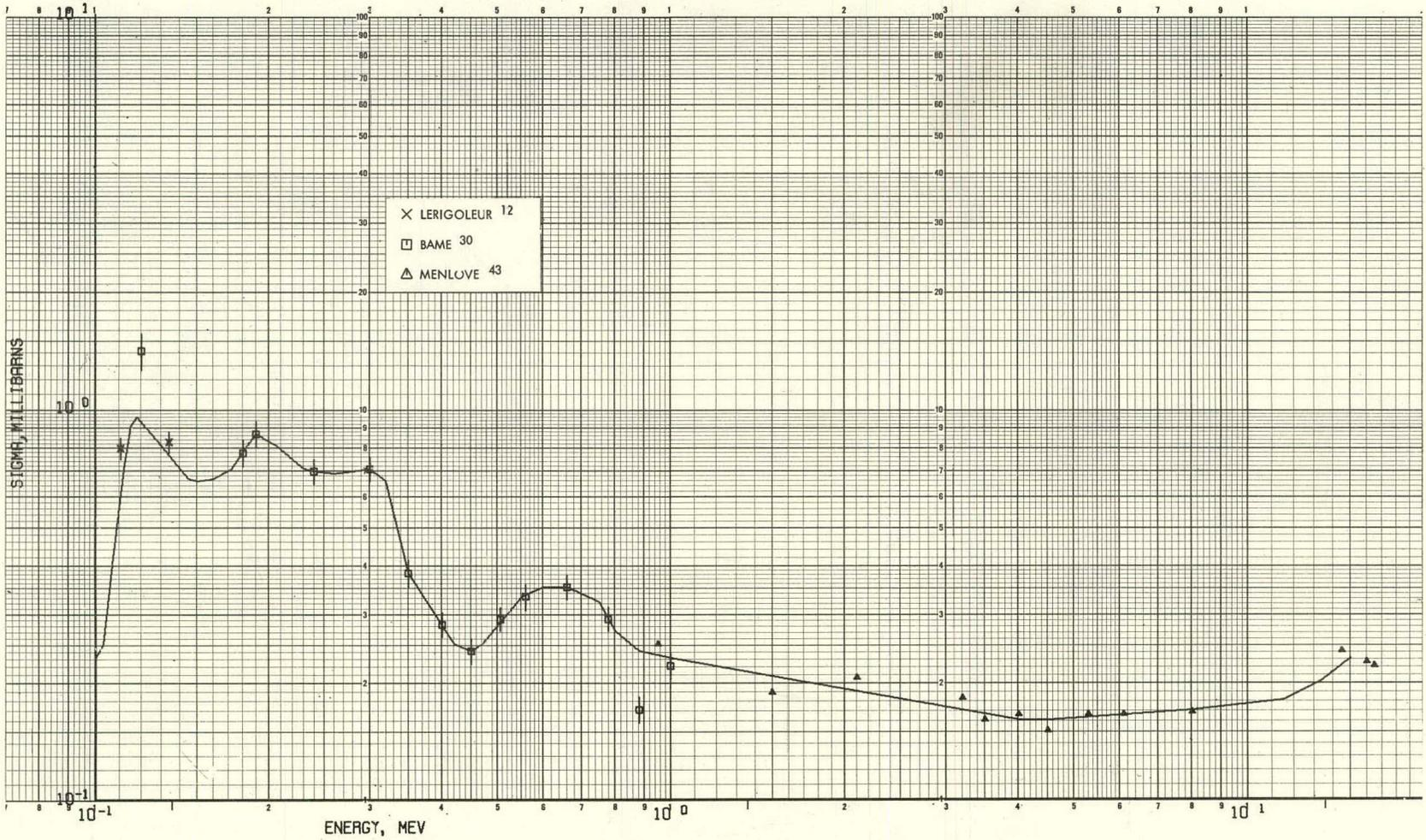
FIG. 10 (n,  $\gamma$ ) CROSS SECTION, 1.0 TO 15 MEV
