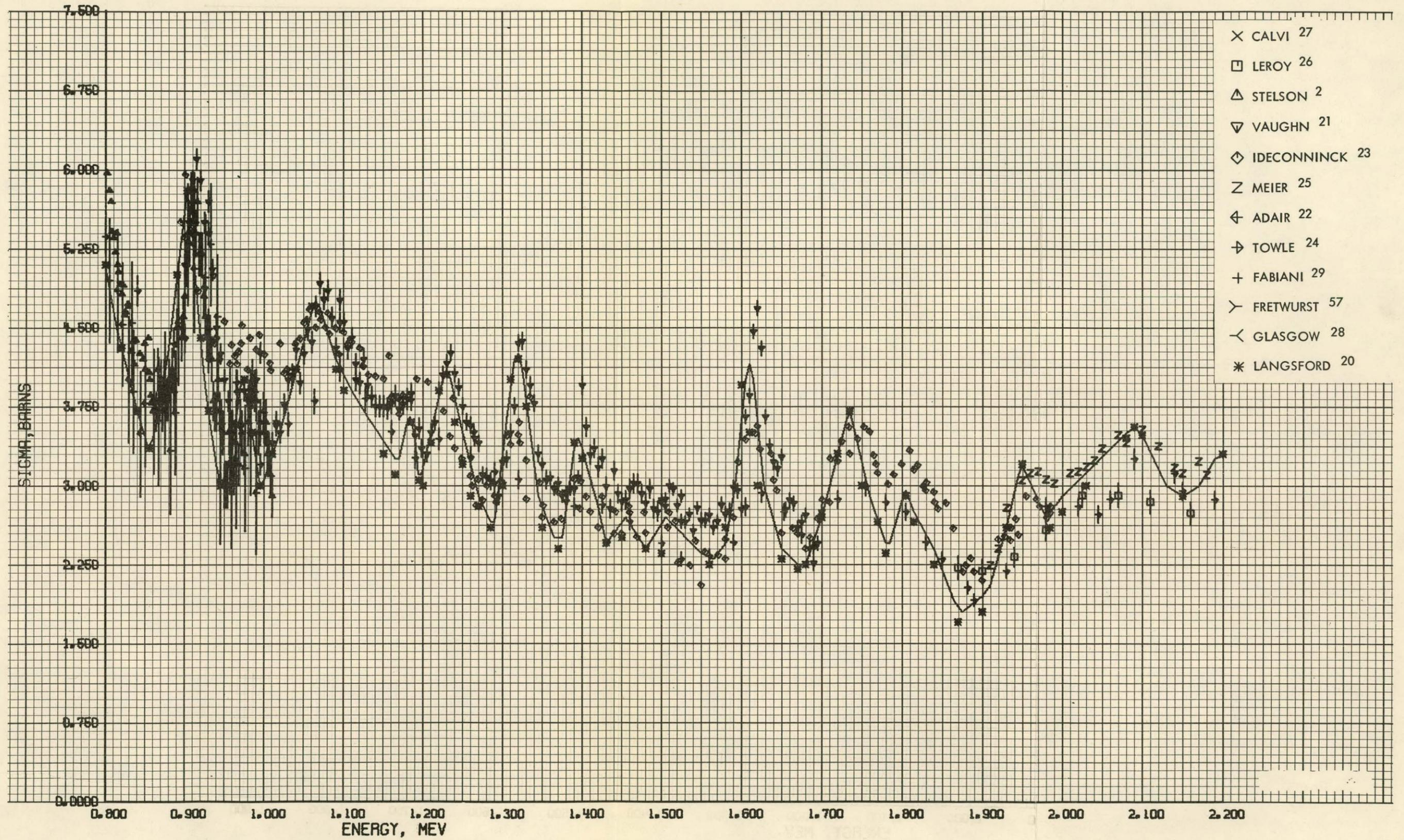
FIG. 6 TOTAL CROSS SECTION, 0.80 TO 2.20 MEV
