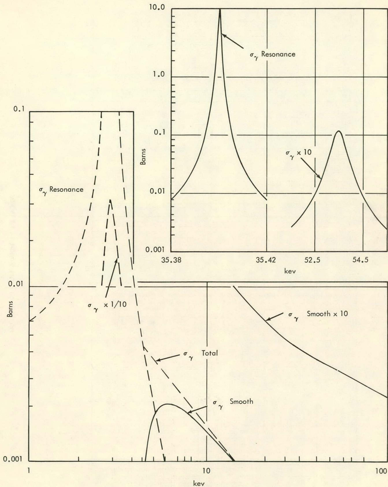
FIG. 9  $(n, \gamma)$  CROSS SECTION, 1.0 TO 100.0 KEV
