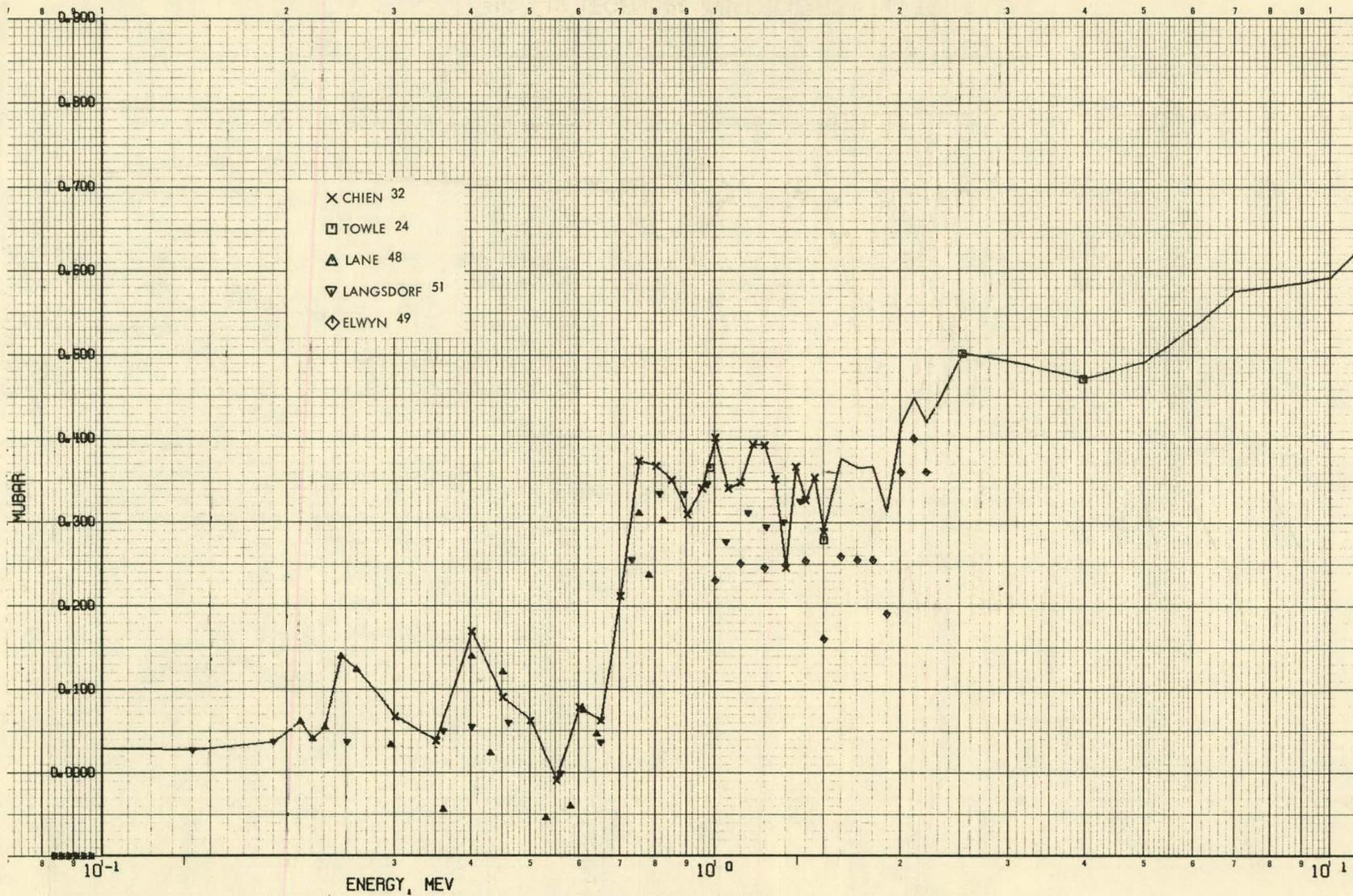
FIG. 18 AVERAGE COSINE OF SCATTERING ANGLE,  $\bar{\mu}$
