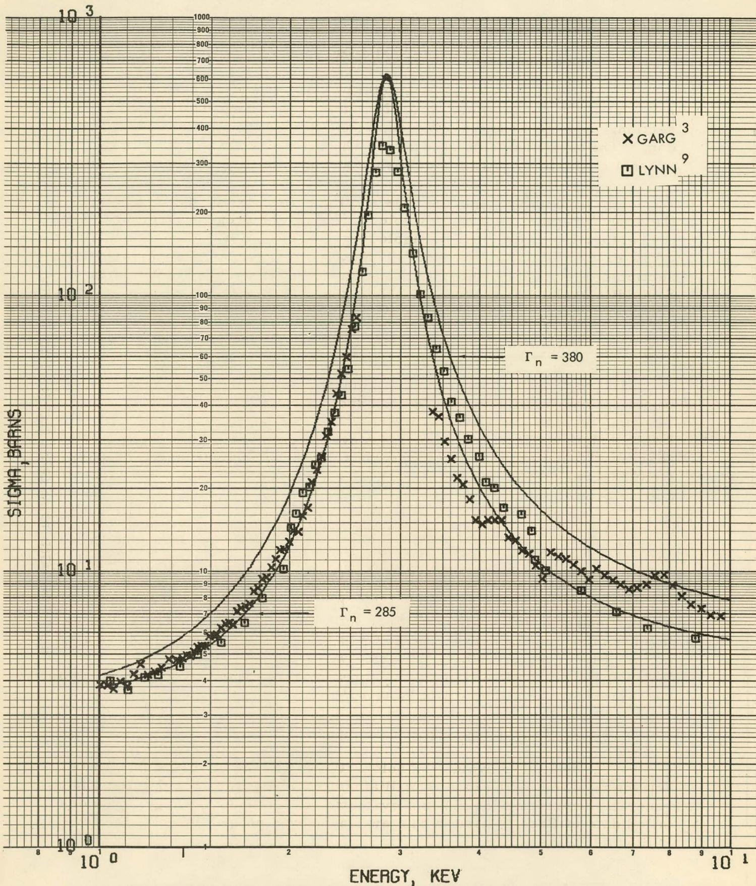
FIG. 1 COMPARISON OF EXPERIMENTAL TOTAL CROSS SECTIONS WITH CALCULATIONS FOR  $J=2$ , 2.85 KEV RESONANCE
