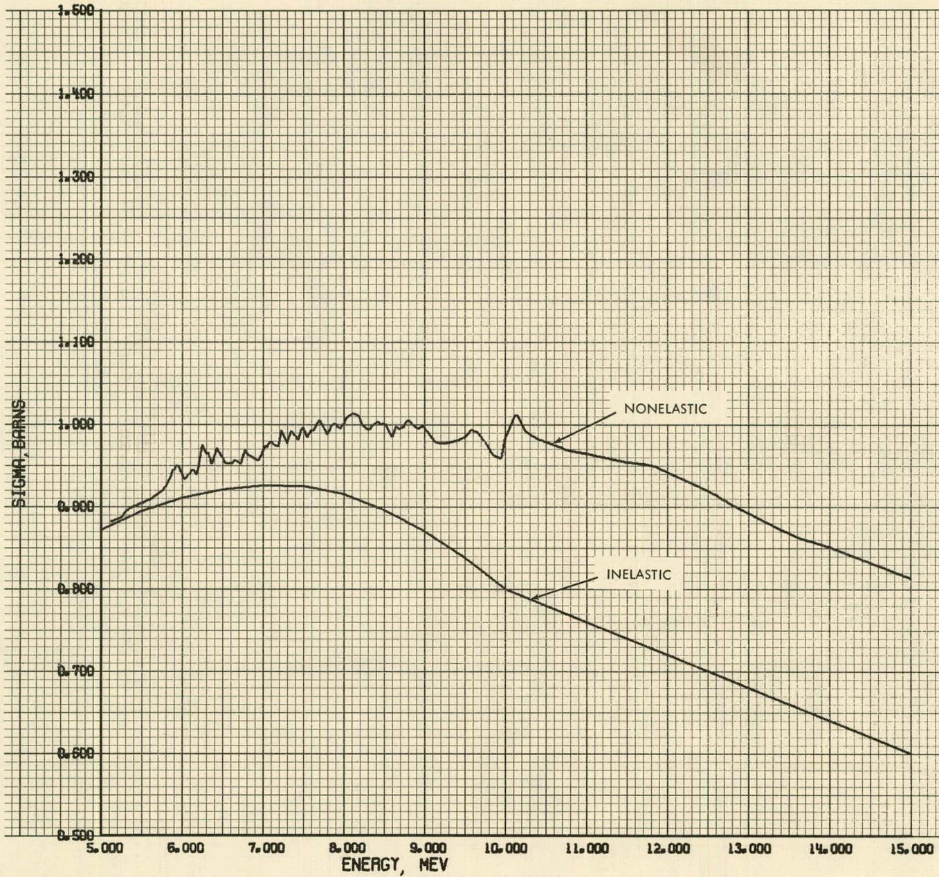
FIG. 14 TOTAL INELASTIC SCATTERING AND NONELASTIC CROSS SECTIONS, 5 TO 15 MEV
