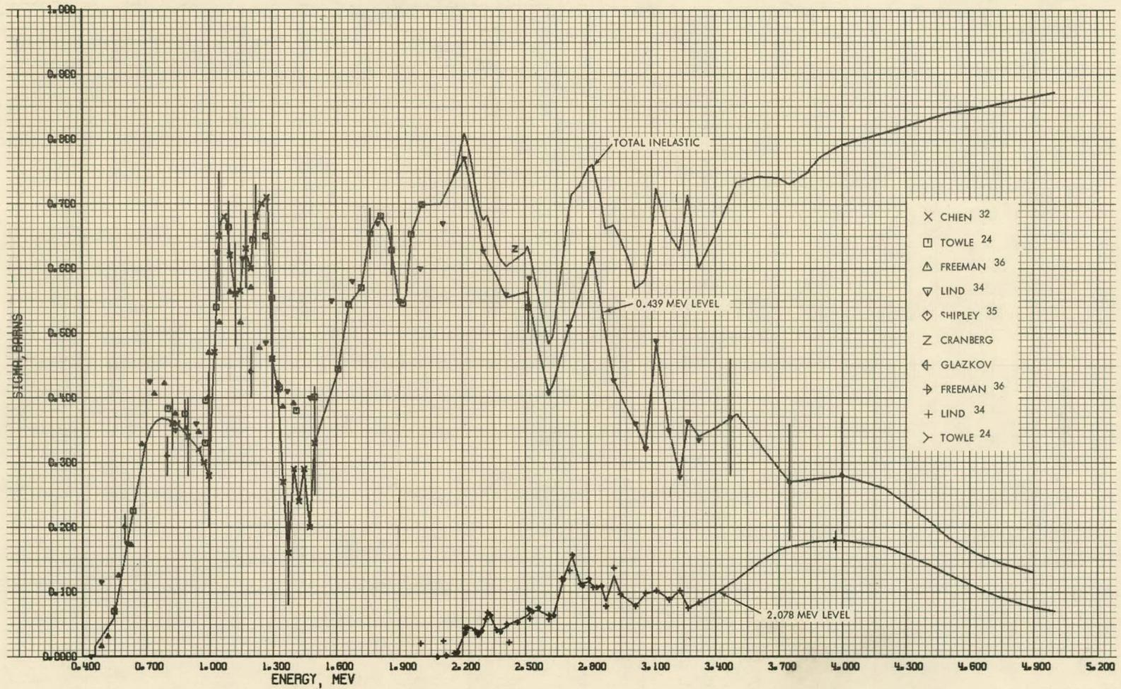
FIG. 11 INELASTIC SCATTERING CROSS SECTIONS, 0.439, 2.078 MEV LEVELS AND TOTAL INELASTIC
