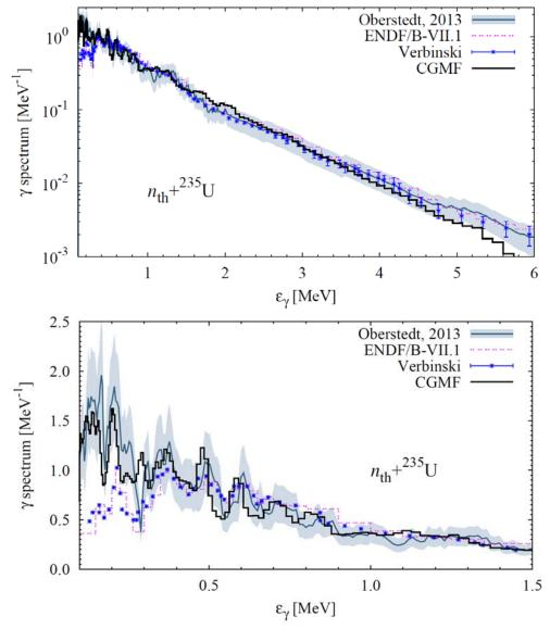
Calculated prompt gamma-ray energy spectra for the thermal neutron induced fission on <sup>235</sup>U with the Monte Carlo Hauser-Feshbach method developed at LANL (shown by the thick histogram), compared with the experimental data. The bottom panel shows the zoomed plot in the low energy region, where the structure in the spectrum evidences importance of the nuclear structure database, ENSDF.
