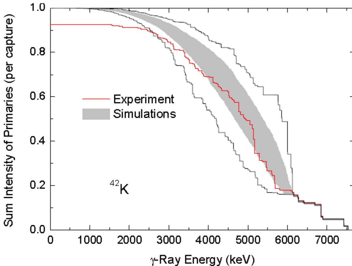
Simulation of primary  $\gamma$ -ray intensities. 100 simulations were performed, 68% fall in the gray area. Experimental primary  $\gamma$ -ray are complete >4 MeV and 92% of primary intensity is observed.
