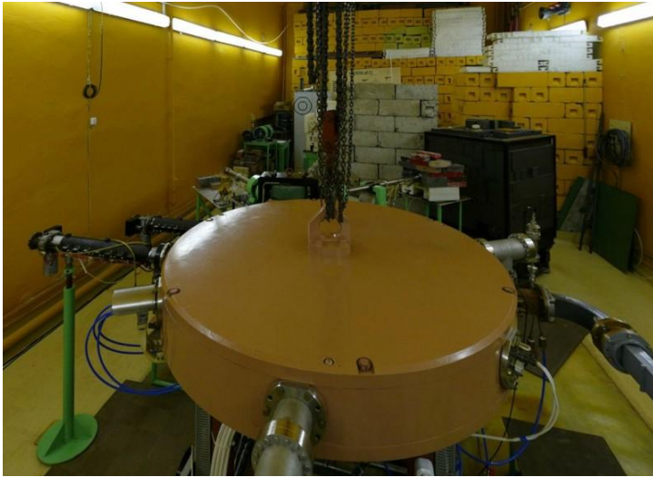
Microntron MT-25 – 5-25 MeV electrons, 25 ma
