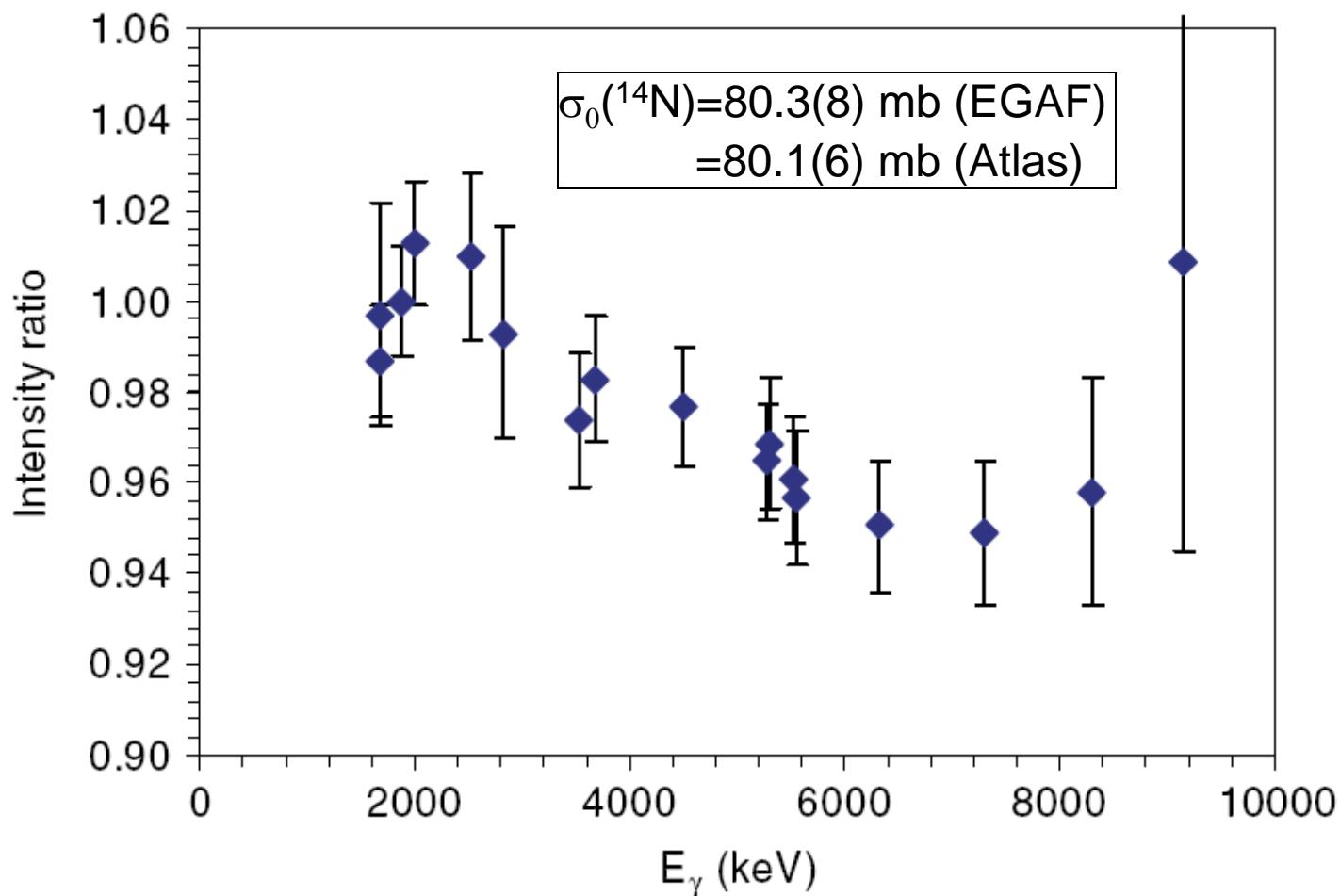
Ratio of  $^{14}\text{N}(\text{n},\gamma)$  gamma-ray intensities measured by Journey (PRC 56, 118, 1997) to those determined from a least-squares fit to the  $^{15}\text{N}$  level scheme by Belgya (PRC 74, 024603, 2006). Journey's values are efficiency standards for high-energy gamma-rays.
