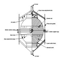
Figure 3. The Active Portion of the Original Jezebel Assembly.
