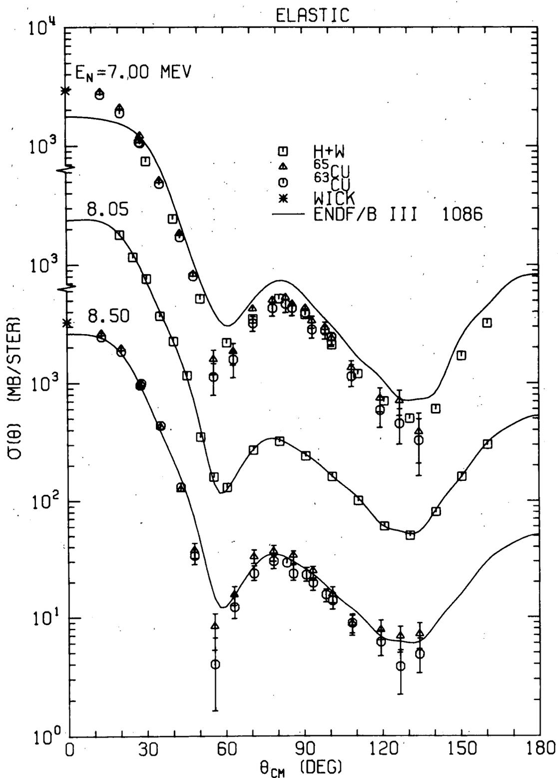
Fig. 5. Our  $^{63}\text{Cu}$  and  $^{65}\text{Cu}$  neutron differential elastic center-of-mass scattering cross sections compared with the data of Holmqvist and Wiedling<sup>2</sup> (H+W) and with ENDF/B III MAT 1086.
