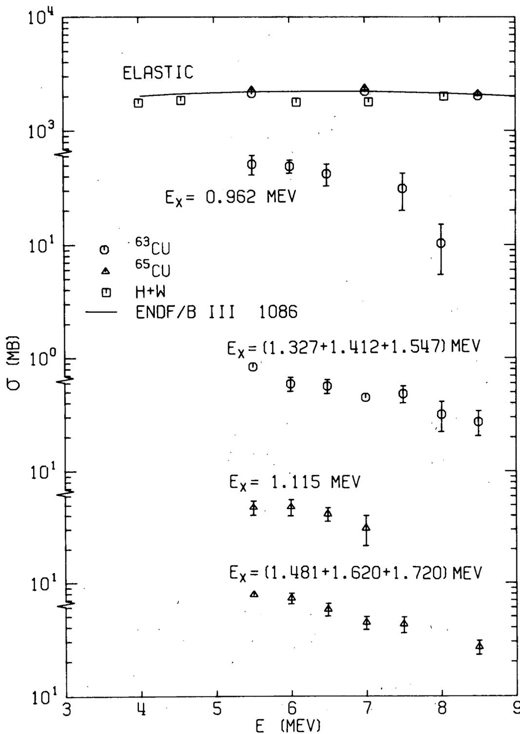
Fig. 10. Our  $^{63}\text{Cu}$  and  $^{65}\text{Cu}$  angle-integrated differential cross sections as a function of incident neutron energy with the elastic data of Holmqvist and Wiedling<sup>2</sup> (H+W) and the curve from ENDF/B III MAT 1086. The 7% uncertainty in absolute normalization is included in our error bars.
