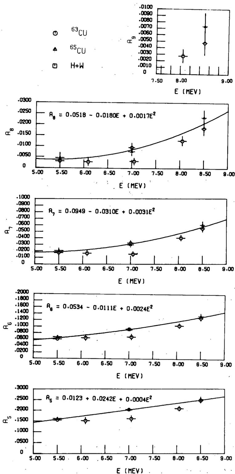
Fig. 7. The fifth through ninth normalized Legendre expansion coefficients obtained from fitting our  $^{63}\text{Cu}$  and  $^{65}\text{Cu}$  elastic differential cross sections and the data of Holmqvist and Wiedling<sup>2</sup> (H+W). The curves are quadratic least squares fits to our data with constants given in the equations.
