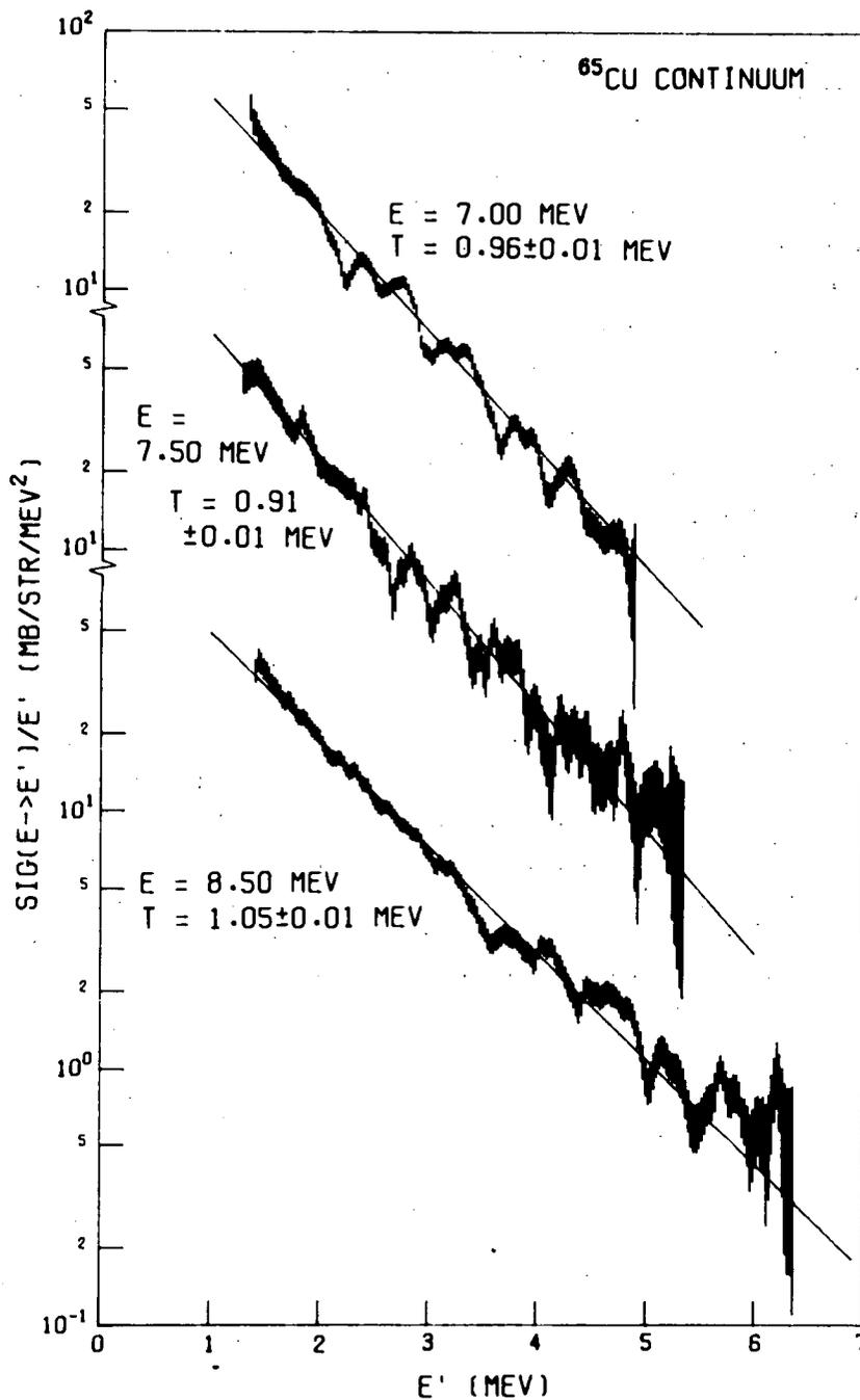
Fig. 16. Our <sup>65</sup>Cu angle-averaged double-differential cross sections for scattering from incident neutron energy E to outgoing neutron energy dE' about E' divided by E' as a function of E'. The straight lines are least squares fits to the data corresponding to excitation energy > 3.5 MeV with resulting temperatures indicated. The uncertainties on the temperatures are fitting uncertainties only.
