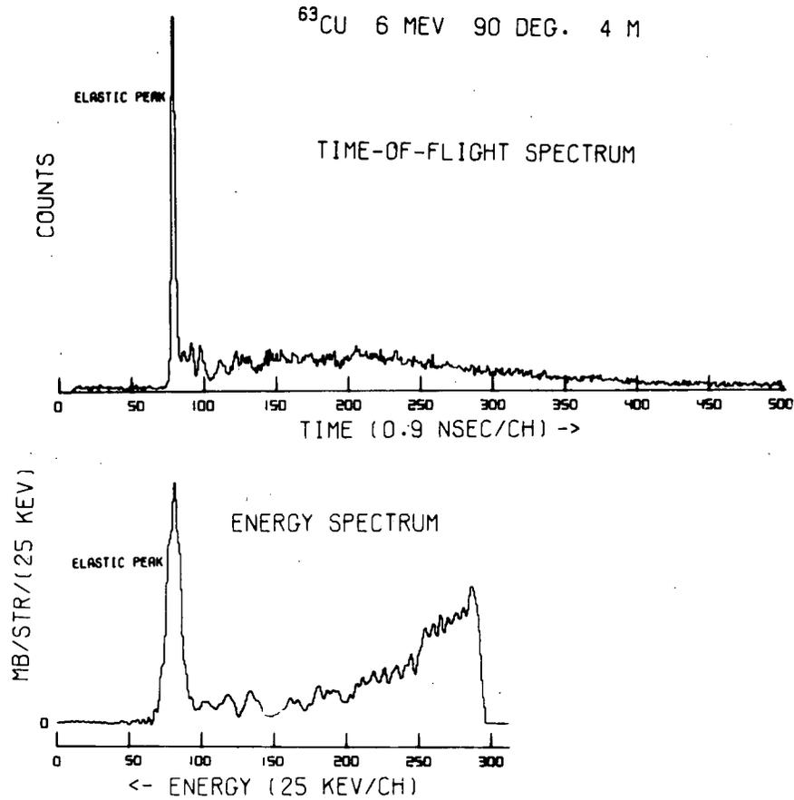
Fig. 1. A typical  $^{63}\text{Cu}$  time-of-flight spectrum with its transformed energy spectrum. The data were taken at an incident neutron energy of 6.00 MeV and at an angle of 90 deg. with a flight path of 4 m. Note that the energy spectrum has been offset to allow negative excursions due to statistics in the subtraction of the sample-out background.
