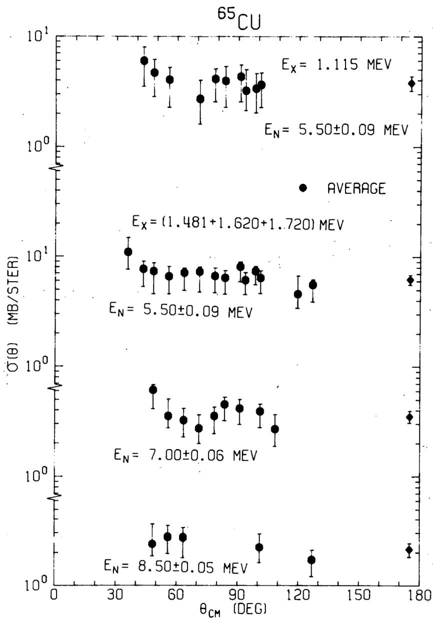
Fig. 9. Our  $^{65}\text{Cu}$  neutron center-of-mass differential inelastic scattering cross sections. The 7% uncertainty in absolute normalization common to all points is not included in the error bars.
