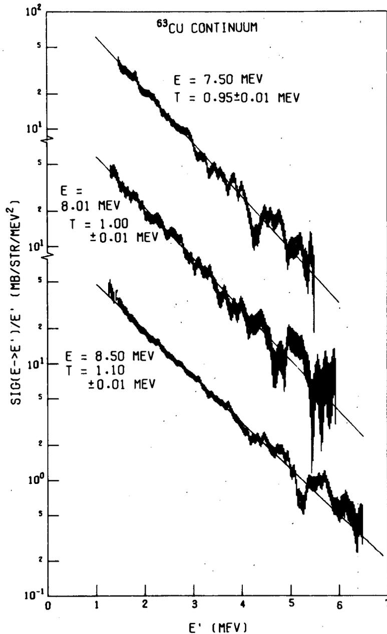
Fig. 14. Our  $^{63}\text{Cu}$  angle-averaged double-differential cross sections for scattering from incident neutron energy,  $E$ , to outgoing neutron energy  $dE'$  about  $E'$  divided by  $E'$  as a function of  $E'$ . The straight lines are least squares fits to the data corresponding to excitation energy  $> 3.5$  MeV with resulting temperatures indicated. The uncertainties on the temperatures are fitting uncertainties only.
