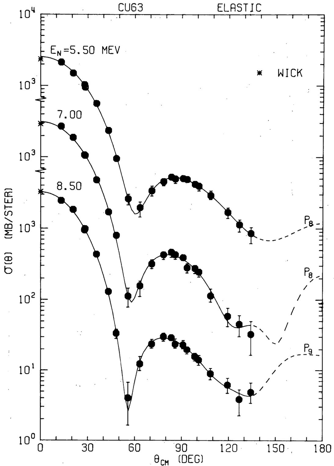
Fig. 2. Our  $^{63}\text{Cu}$  neutron differential elastic center-of-mass scattering cross sections with Legendre fits to the data. WICK indicates Wick's Limit which was used in the fitting. The 7% uncertainty in absolute normalization common to all points is not included in the error bars.
