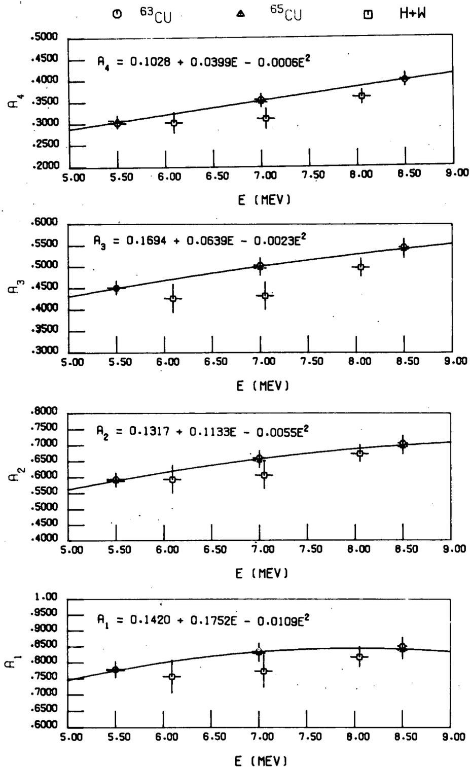
Fig. 6. The first through fourth normalized Legendre expansion coefficients obtained from fitting our <sup>63</sup>Cu and <sup>65</sup>Cu elastic differential cross sections and the data of Holmqvist and Wiedling<sup>2</sup> (H+W). The curves are quadratic least squares fits to our data with constants given in the equations.
