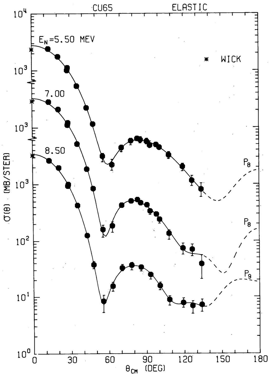
Fig. 3. Our  $^{65}\text{Cu}$  neutron differential elastic center-of-mass scattering cross sections with Legendre fits to the data. WICK indicates Wick's Limit which was used in the fitting. The 7% uncertainty in absolute normalization common to all points is not included in the error bars.
