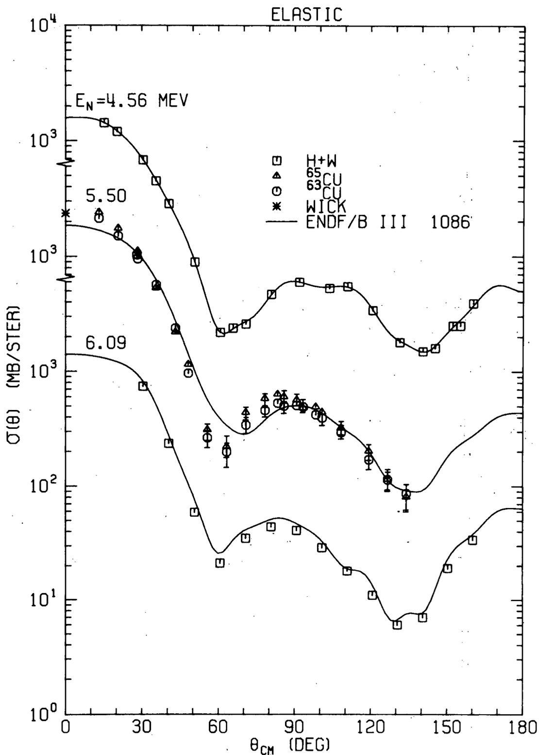
Fig. 4. Our  $^{63}\text{Cu}$  and  $^{65}\text{Cu}$  neutron differential elastic center-of-mass scattering cross sections compared with the data of Holmqvist and Wiedling<sup>2</sup> (H+W) and with ENDF/B III MAT 1086.
