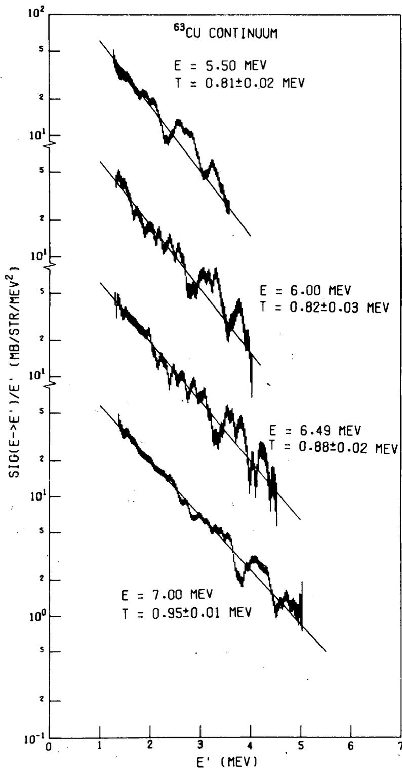
Fig. 13. Our  $^{63}\text{Cu}$  angle-averaged double-differential cross sections for scattering from incident neutron energy  $E$  to outgoing neutron energy  $dE'$  about  $E'$  divided by  $E'$  as a function of  $E'$ . The straight lines are least squares fits to the data corresponding to excitation energy  $> 3.5$  MeV with resulting temperatures indicated. The uncertainties on the temperatures are fitting uncertainties only.
