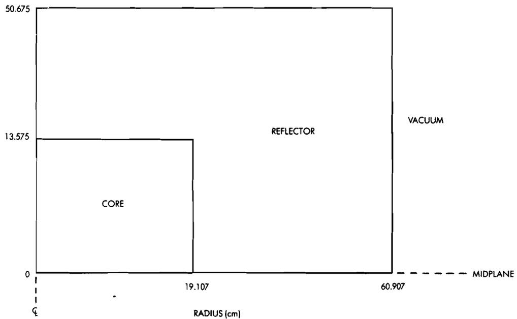
Figure 2. Two-Dimensional (R-Z) Model of VERA-1B Assembly
