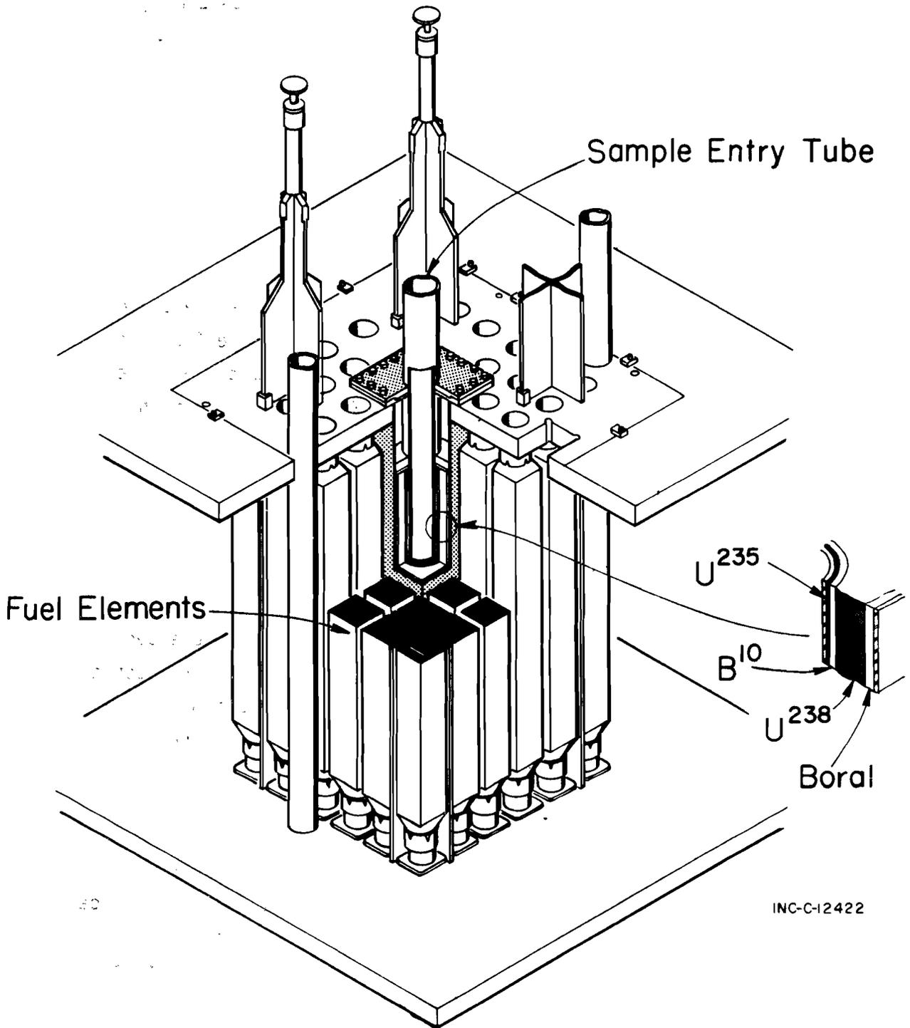
Fig. 1 Cutaway pictorial diagram showing general assembly of the CFRMF.
