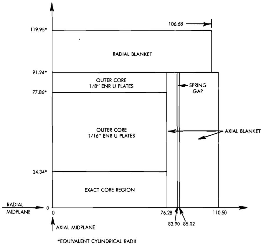
Figure 3. Axial Cross Section for 75.1 Ih Excess Reactivity, As-Built ZPR-6 Assembly 6A, ANL-Neg. No. 116-892.
