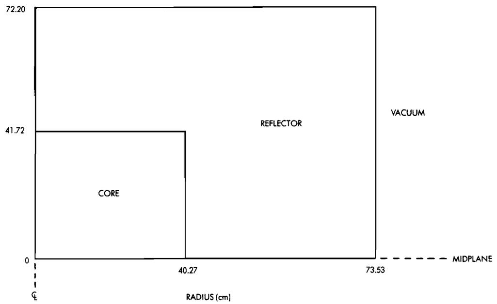
Figure 2. Two-Dimensional (R-Z) Model of ZEBRA-2 Assembly
