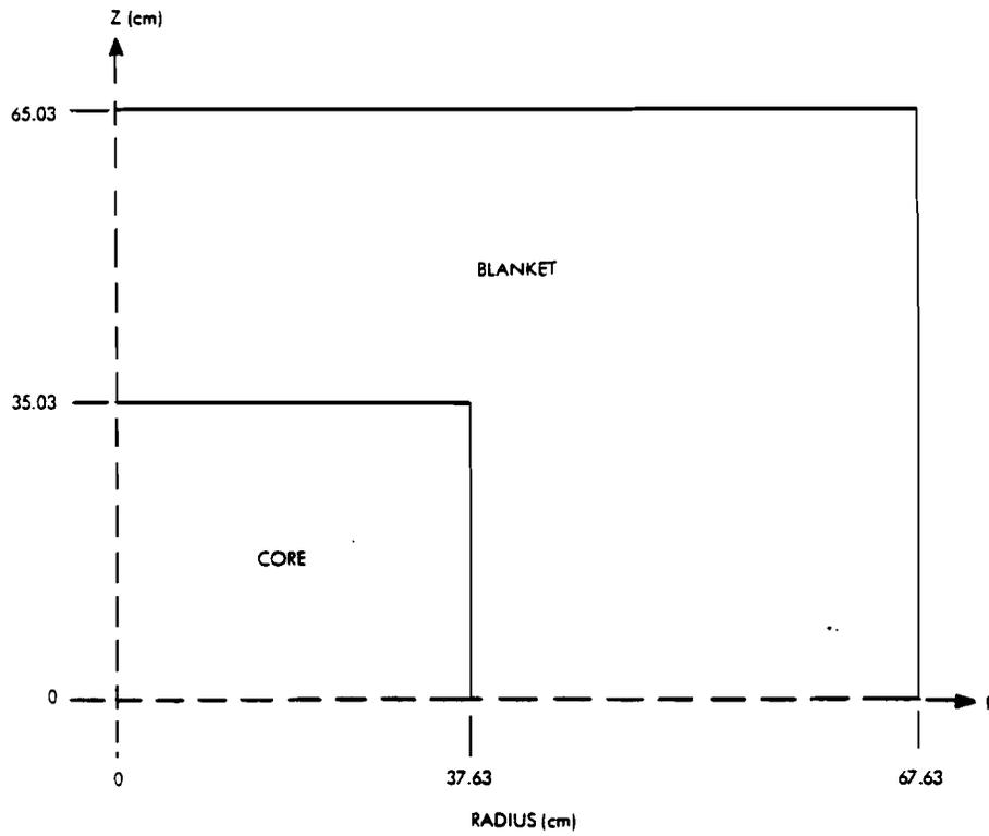
Figure 1. RZ-model for assembly SNEAK-7B.
