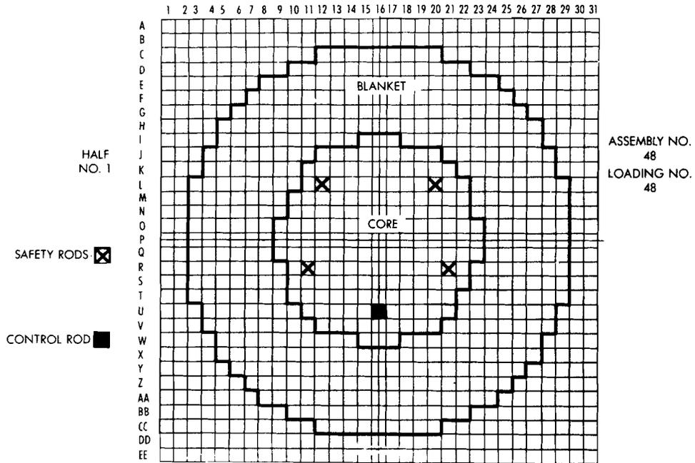
Figure 2. Assembly 48 Drawer Arrangement in Half No. 1
