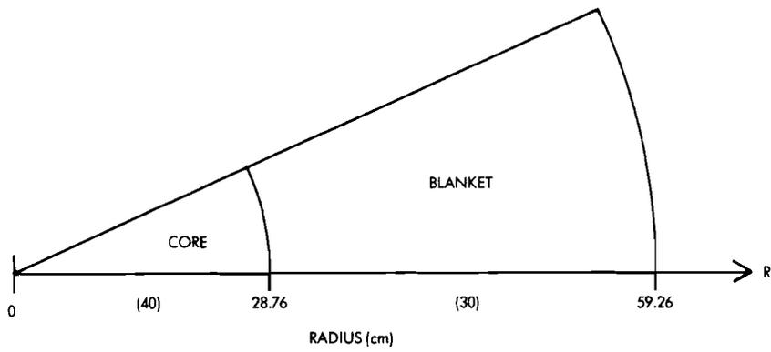
Figure 1. Spherical Model of ZPR-III Assembly 12.
