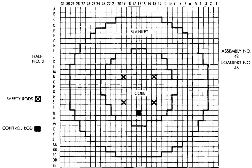
Figure 3. Assembly 48 Drawer Arrangement in Half No. 2
