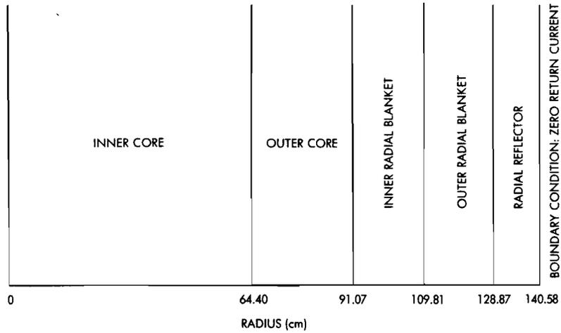
Figure 2. Radial Model of ZPPR Assembly 02.
