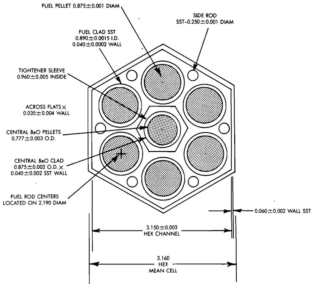
Figure 4. SEFOR Fuel Subassembly
