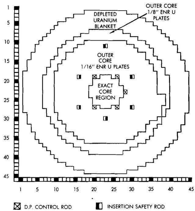
Figure 2. Radial Cross Section for 75.1  $\Delta k$  Excess Reactivity, As-Built ZPR-6 Assembly 6A, ANL-Neg. No. 116-890.
