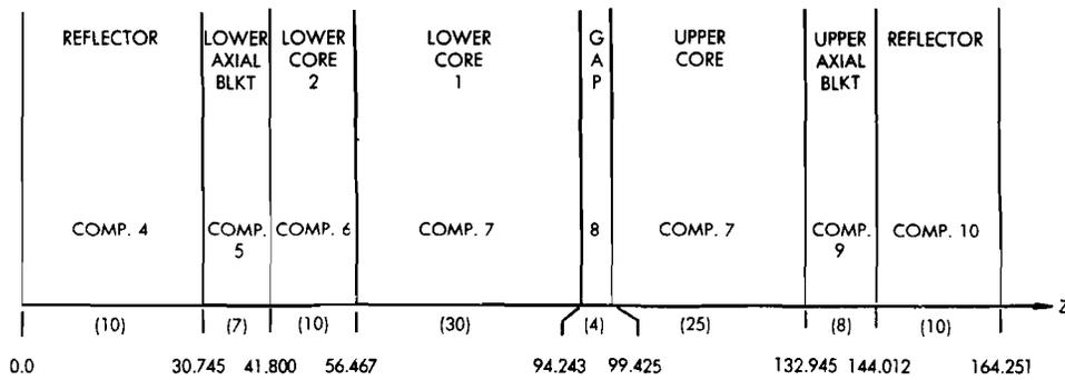
Figure 2. SEFOR Doppler Benchmark Axial One-Dimensional Model.
