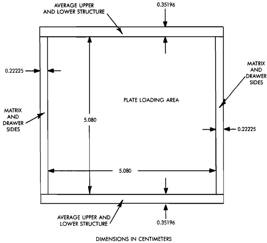
Figure 3. Geometry of ZPPR Unit-Matrix Cells
