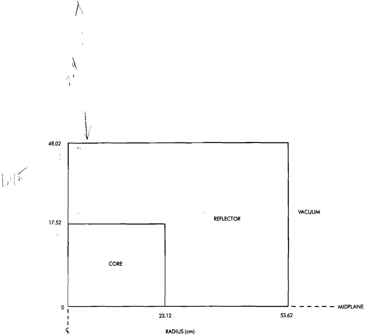
Figure 2. Two-Dimensional (R-Z) Model of ZEBRA-3 Assembly
