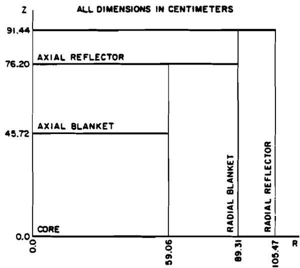
Figure 5. Carbide benchmark R-Z calculational model.
