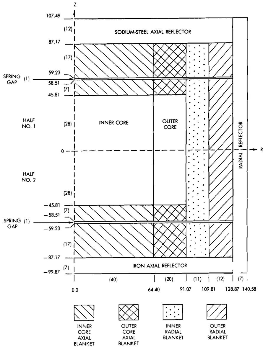
Figure 1. Benchmark Model of ZPPR Assembly O2.
