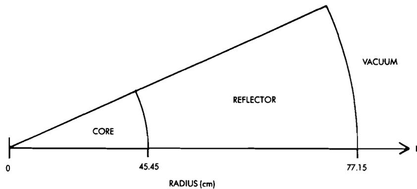
Figure 1. Spherical Model of ZEBRA-2 Assembly
