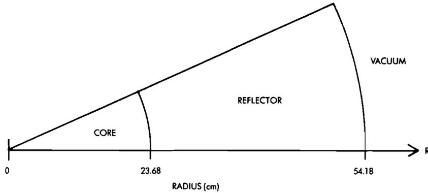
Figure 1. Spherical Model of ZEBRA-3 Assembly
