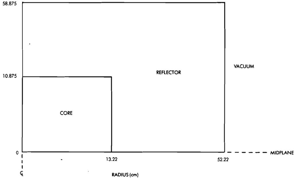
Figure 2. Two-Dimensional (R-Z) Model of VERA-11A Assembly
