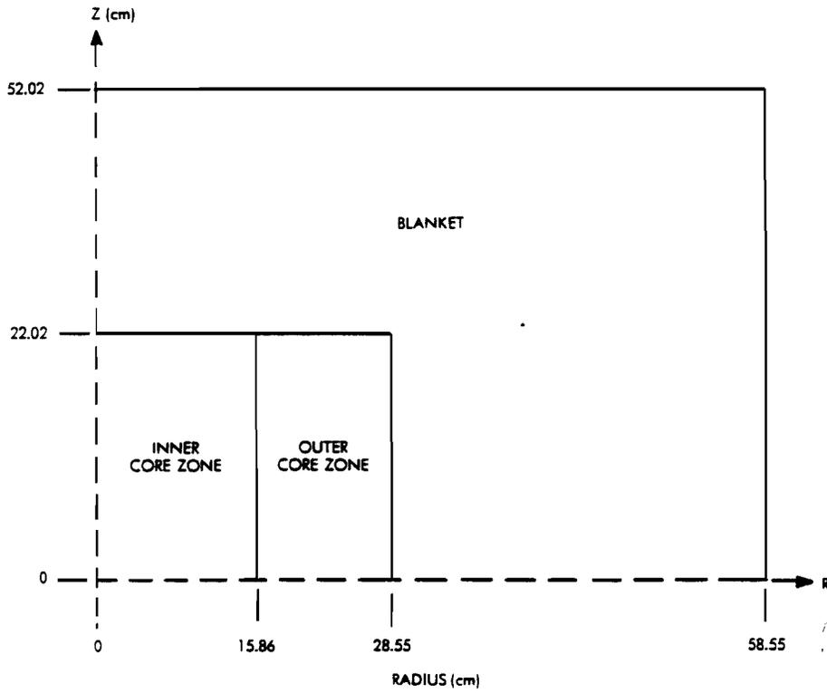
Figure 1. RZ-model for assembly SNEAK-7A.
