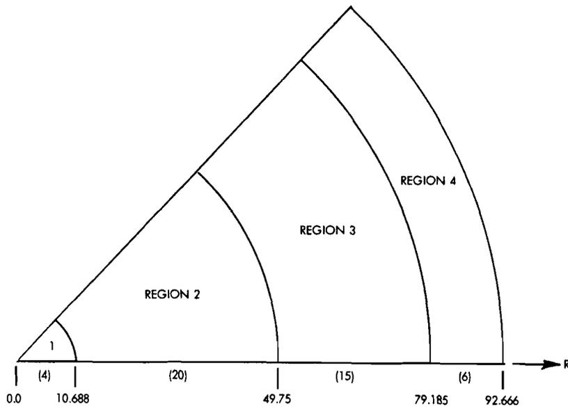
Figure 1. SEFOR Doppler Benchmark Spherical Model.
