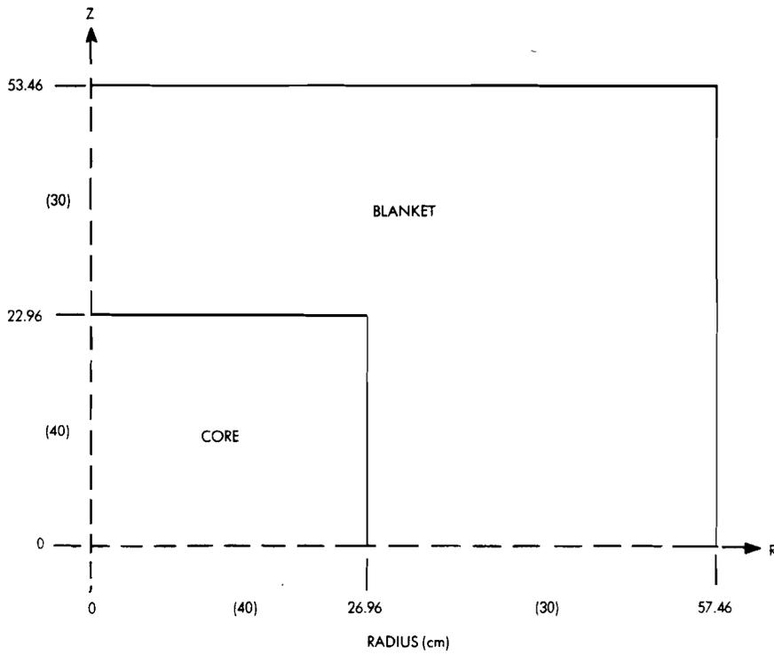
Figure 2. Two-Dimensional (R-Z) Model of ZPR-III Assembly 12.
